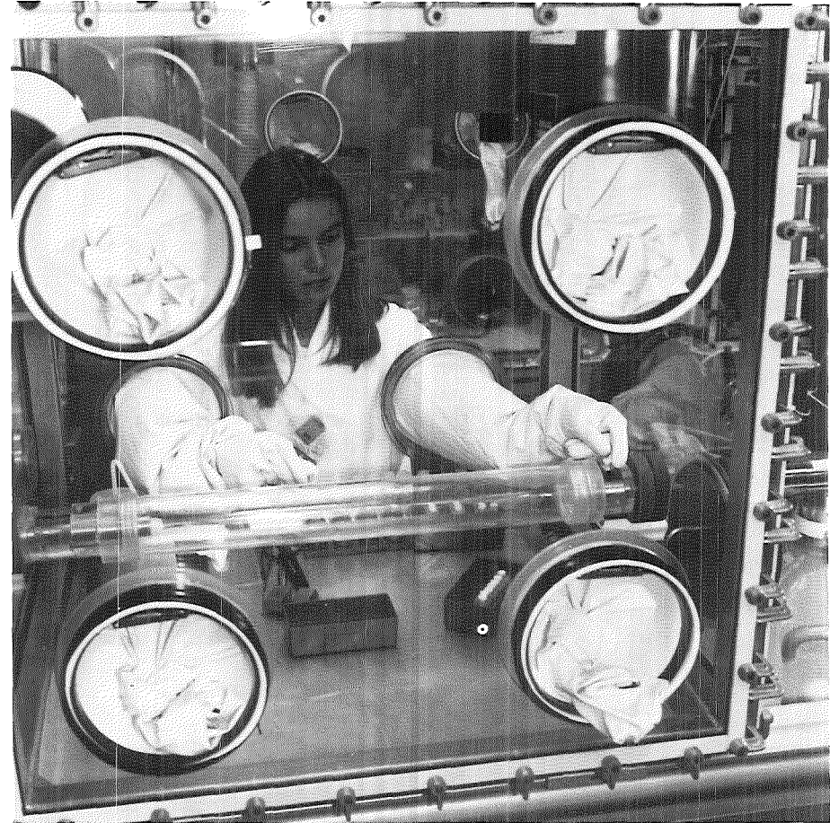
Fig. 6 View into the glovebox showing the beam tube with the sample adapters for densitometry (left) and Pu isotopic analysis (right).
