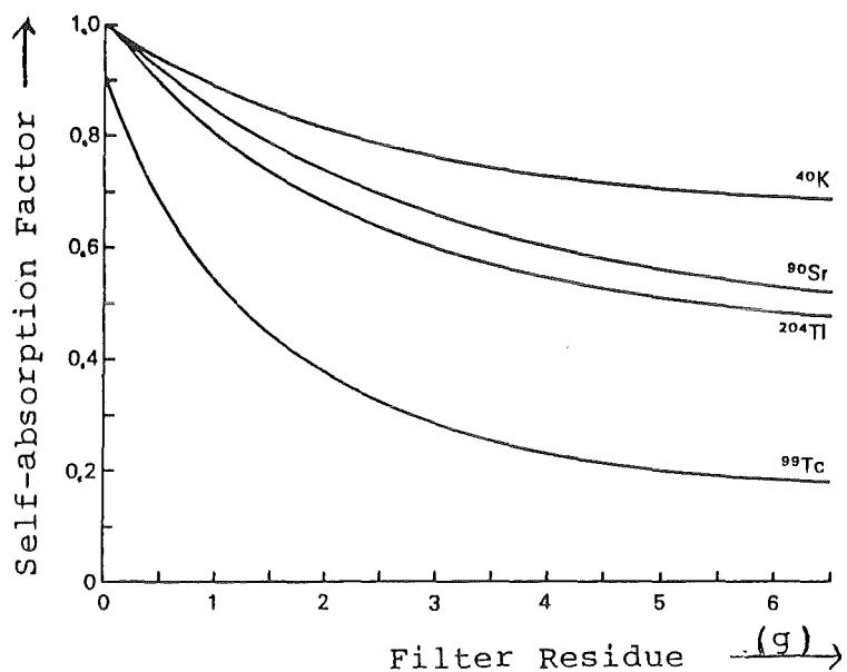
Figure 57: Correction Curve for Self-absorption
