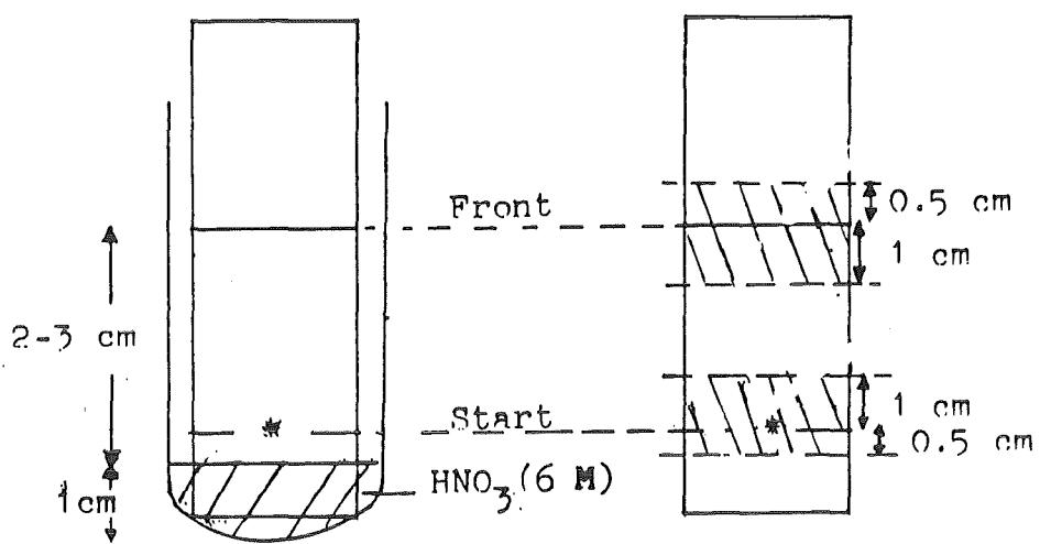
Figure 46: Chromatographic Separation of  $^{137}\text{Cs}/^{137\text{m}}\text{Ba}$
