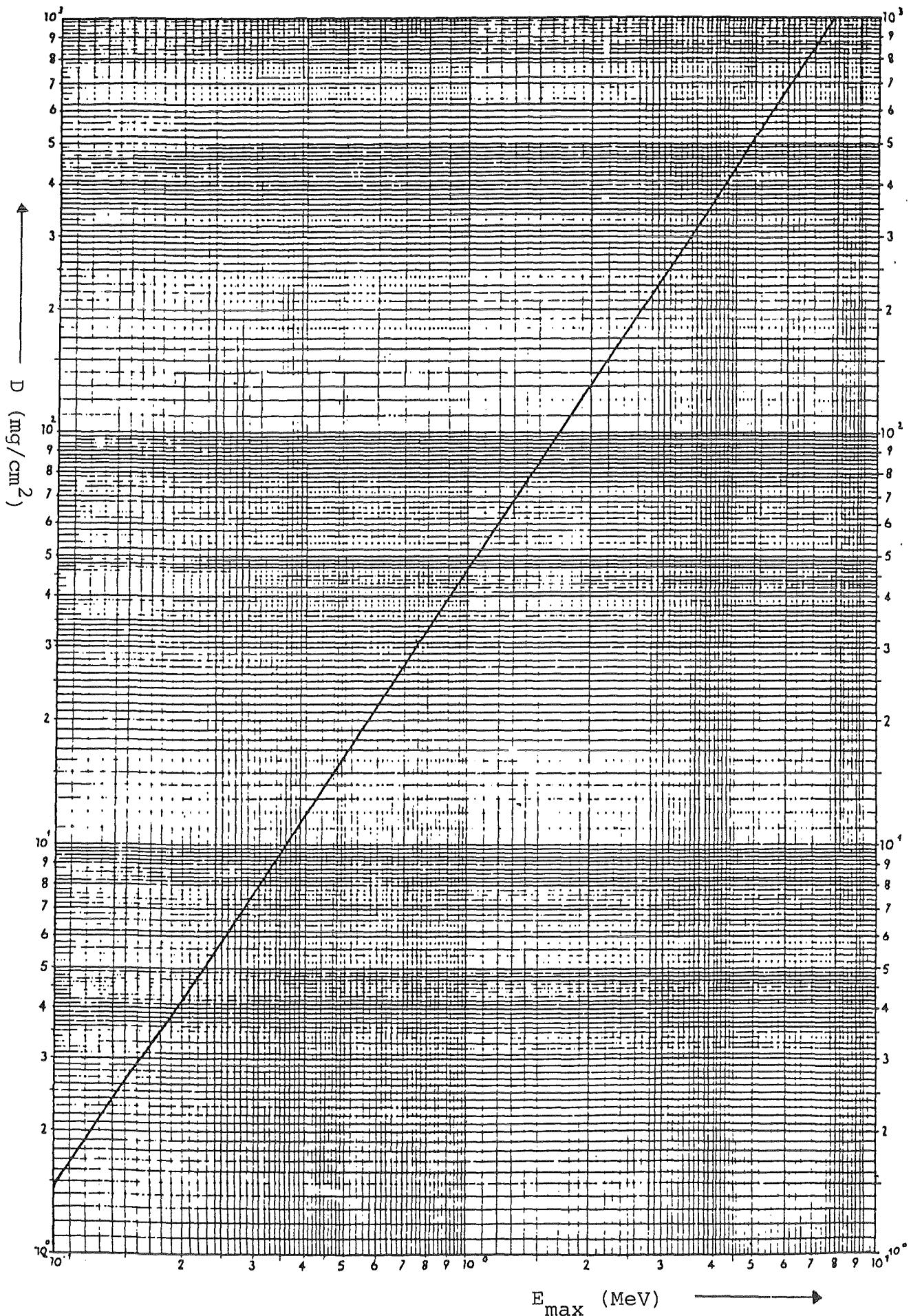
Figure 15: Half-thickness  $D$  of Al as a Function of Maximum Energy  $E_{\max}$  of the  $\beta$ -spectrum
