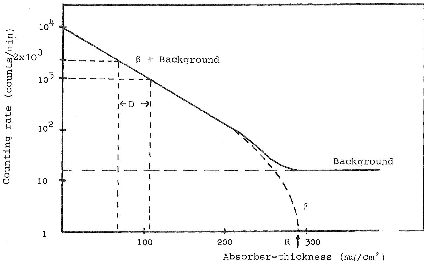
Figure 13: Determination of Half-thickness  $D$  and Maximum Range  $R$
