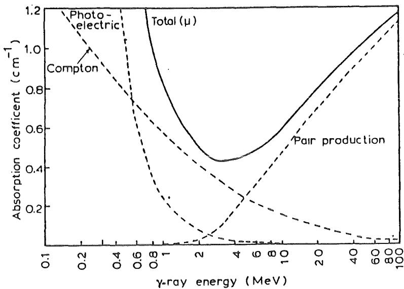
Figure 20: Total and Partial Absorption Coefficients for  $\gamma$ -rays in Lead
