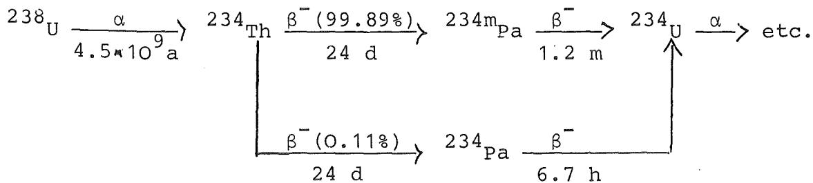
This experiment illustrates the separation of the daughter products produced in the decay of  $^{238}\text{U}$ , using the techniques of solvent extraction and ion exchange.
