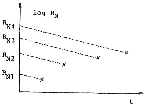
Figure 64: Scheme for Extrapolation of  $R_N$
