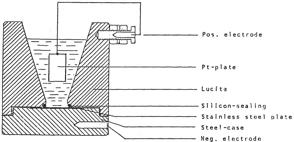
Figure 37: Electrolytic Cell
