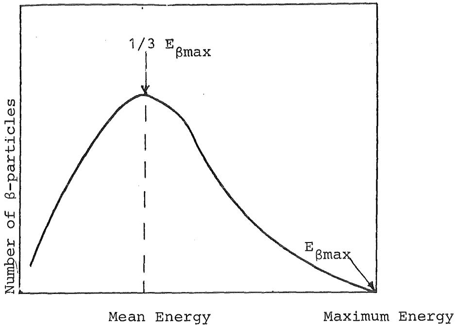
Figure 10: Energy Distribution of  $\beta$ -radiation
