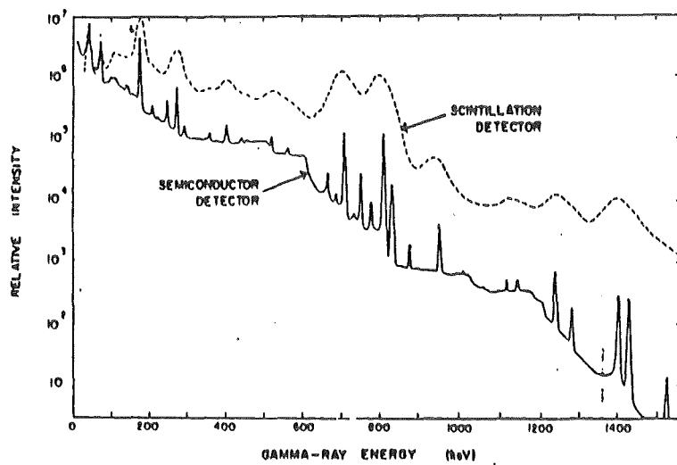
**Figure 23:** Comparison of Pulse-height Analyser Results for  $\gamma$ -rays from  $^{166m}\text{Ho}$  Using Scintillation and Lithium-drifted Germanium Detector.
