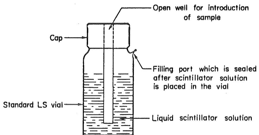
Figure 33: Vial for Counting Gamma Emitters ( $\gamma$ -vial)
