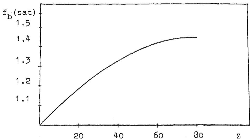
Figure 9: Backscattering Factor at Saturation Thickness
