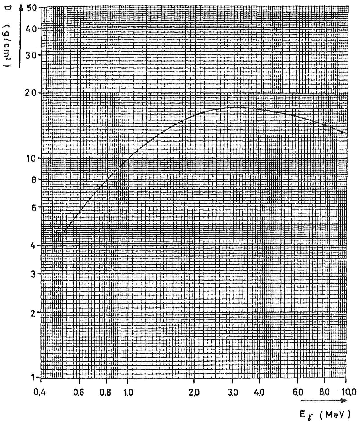
Figure 21: Half-thickness  $D$  for  $\gamma$ -photons in Lead
