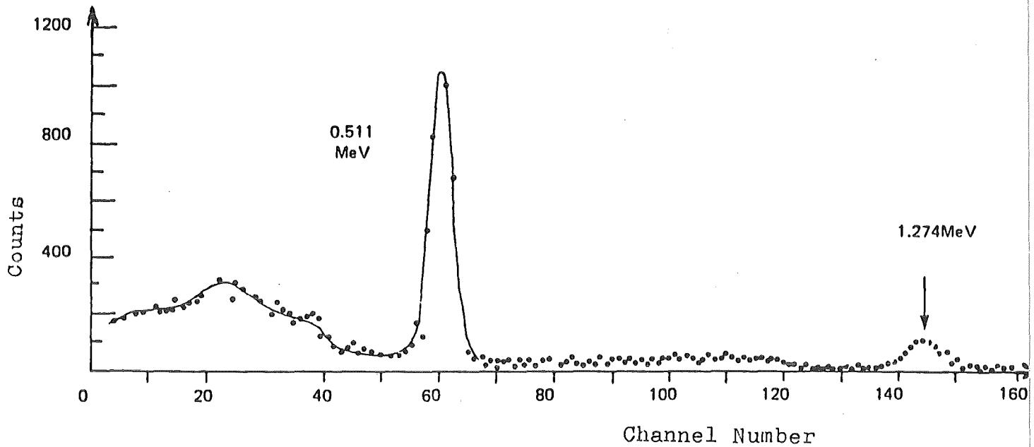
Figure 26:  $\gamma$ -ray Spectrum of  $^{22}\text{Na}$
