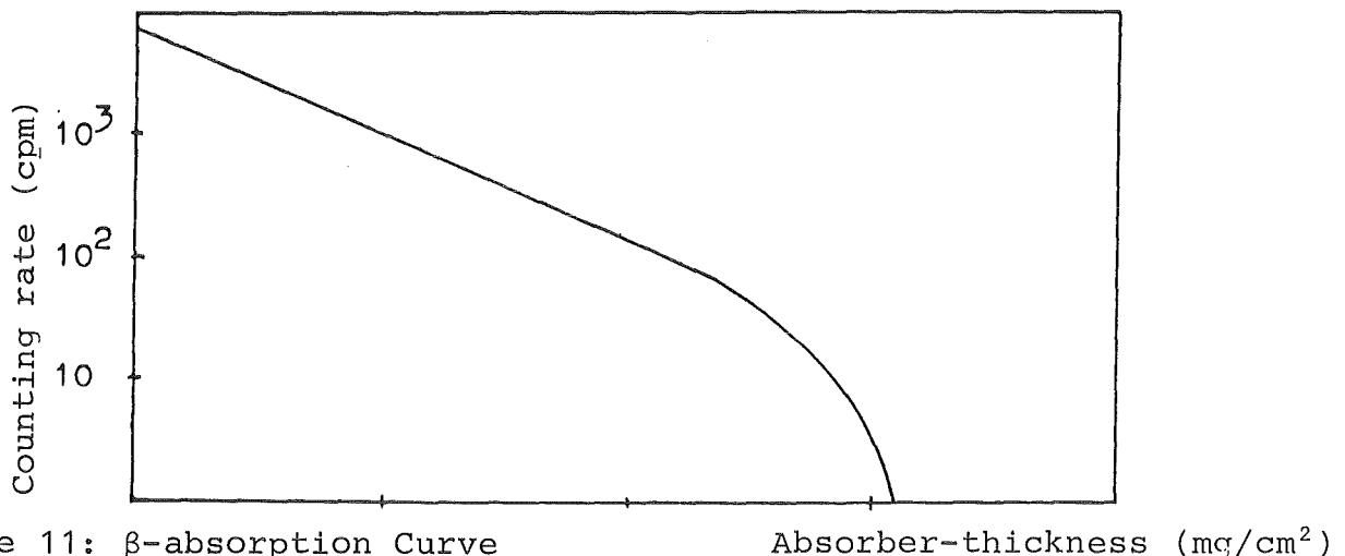
The resulting graph is nearly linear. The exponential absorption of  $\beta$ -radiation from a simple  $\beta$ -emitter is a fortuitous result of the continuous  $\beta$ -spectrum and the effects of scattering.
