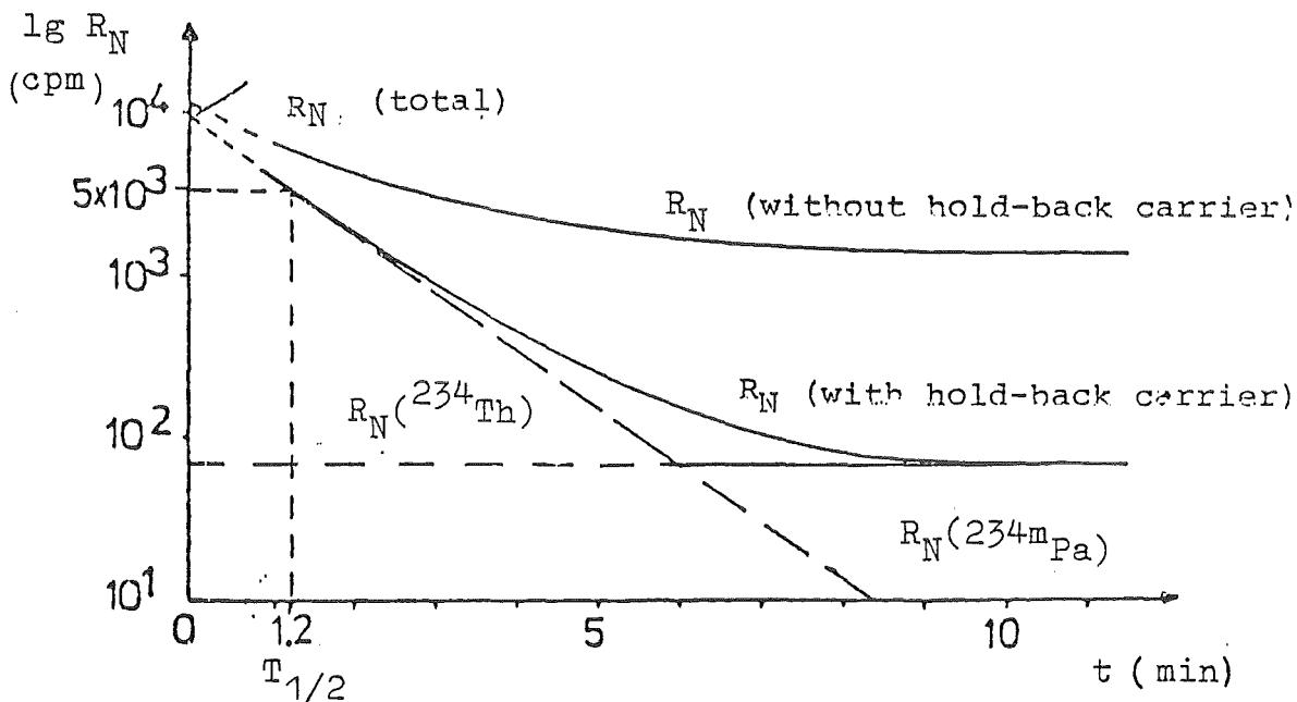
Figure 50: Decay Curve of  $^{234m}\text{Pa}$  with  $^{234}\text{Th}$  as Contamination
