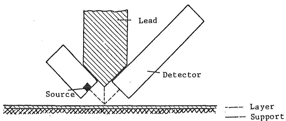
Figure 59: Arrangement for Measurement of Layer Thicknesses
