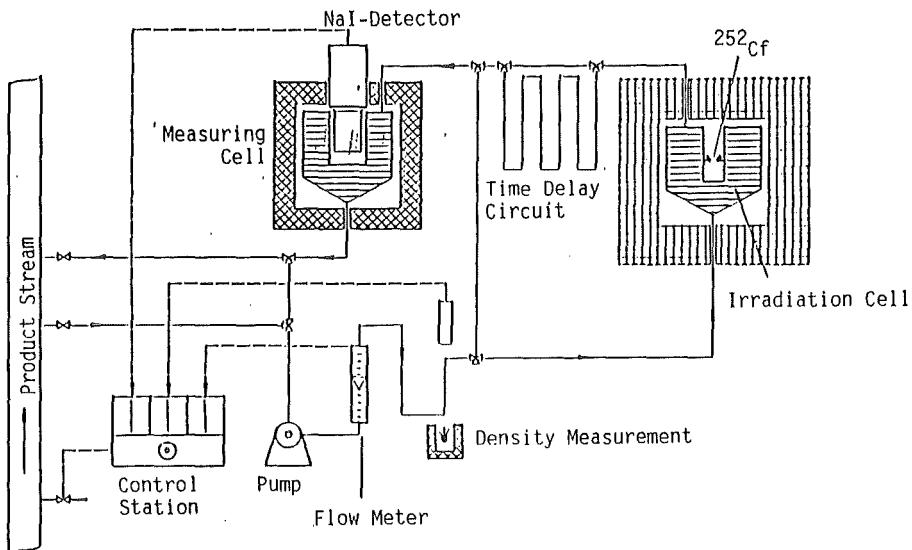
Figure 57c: On-line Loop Arrangement for Determination of Trace Elements in Process Streams
