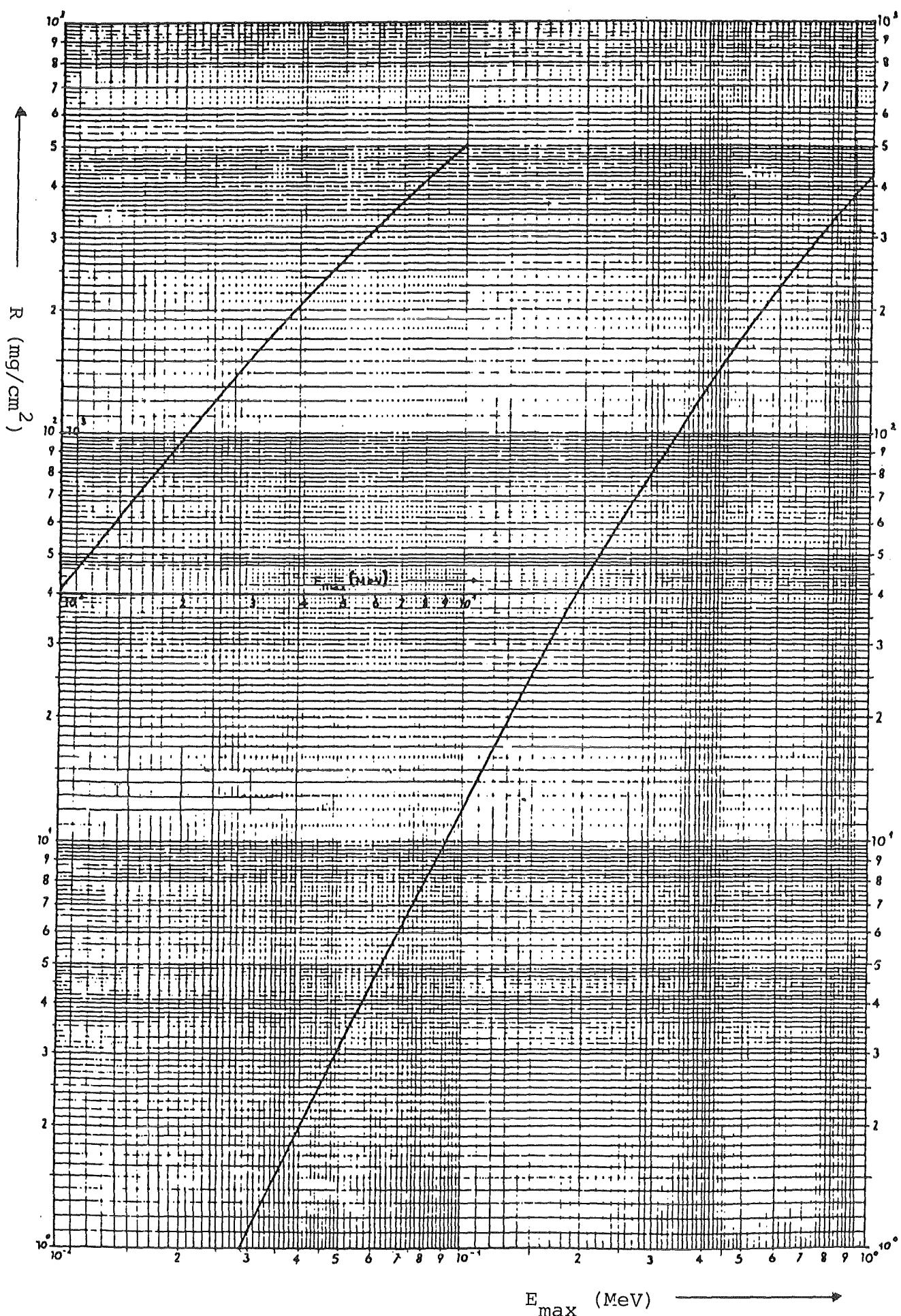
Figure 16: Maximum Range in Al as a Function of
