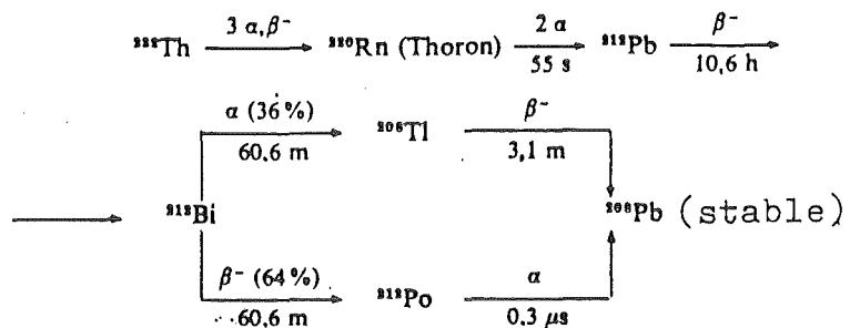
These decay products might be deposited on a negatively charged metal plate (Pt).
