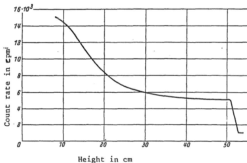
Figure 60: Typical Characteristic for Level Measurements (2-source-system)
