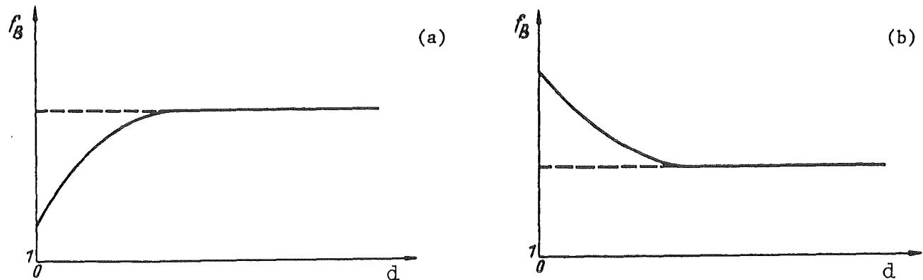
Figure 61: Backscattering Factor  $f_B$  vs. Layer Thickness  $d$
