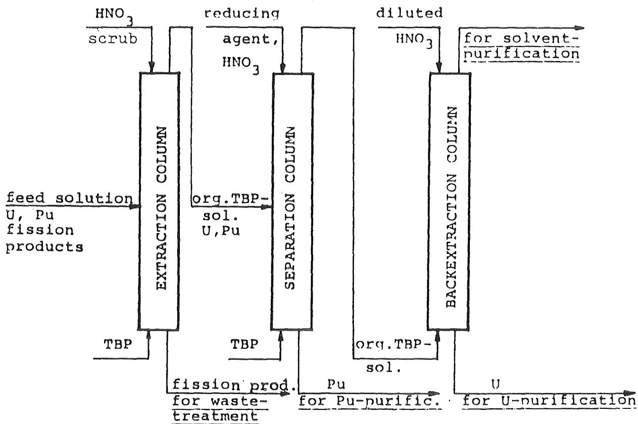
Figure 53: Scheme of PUREX-extraction Process
