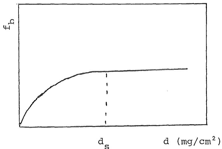
Figure 8: Backscattering Factor  $F_b$  Plotted Against the Thickness of the Support
