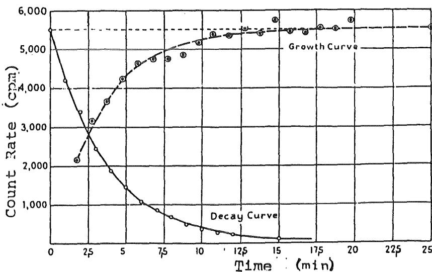
Figure 45: Secular Equilibrium for  $^{137}\text{Cs}/^{137m}\text{Ba}$
