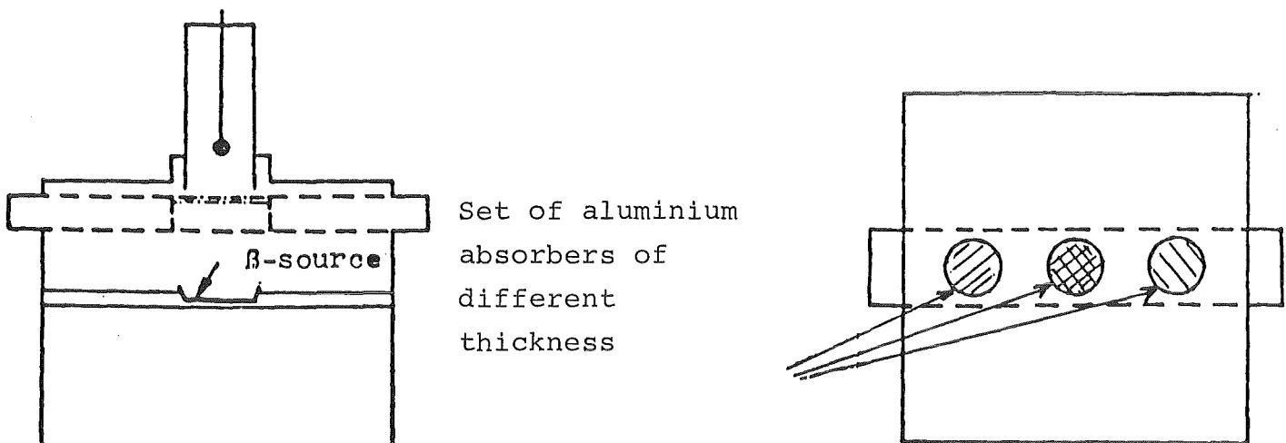
Figure 12: Measuring Apparatus (schematic)
