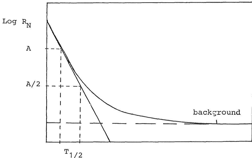
Figure 41: Determination of the Half-life from the Decay Curve
