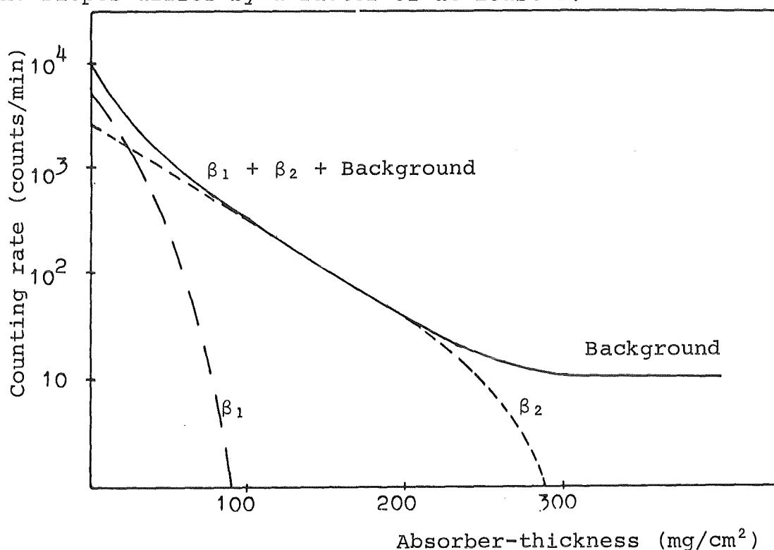
Figure 14: Analysis of the Absorption Curve of a Complex  $\beta$ -Spectrum (2 components):
