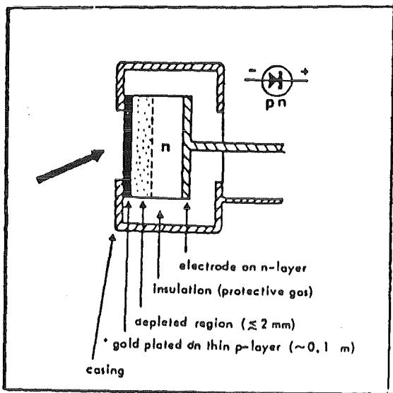
Figure 36: Surface Barrier Detector; the Thickness of the Gold and the p-layer is exaggerated.
