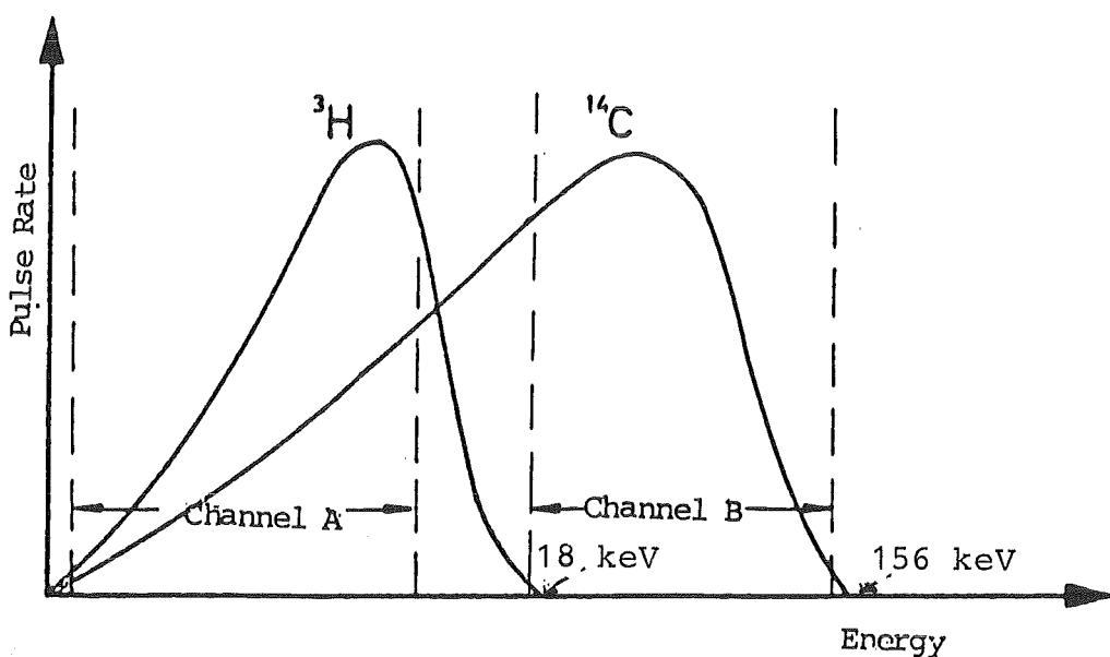
Figure 32: Channel Setting for Measurement of Dual-Labelled Samples
