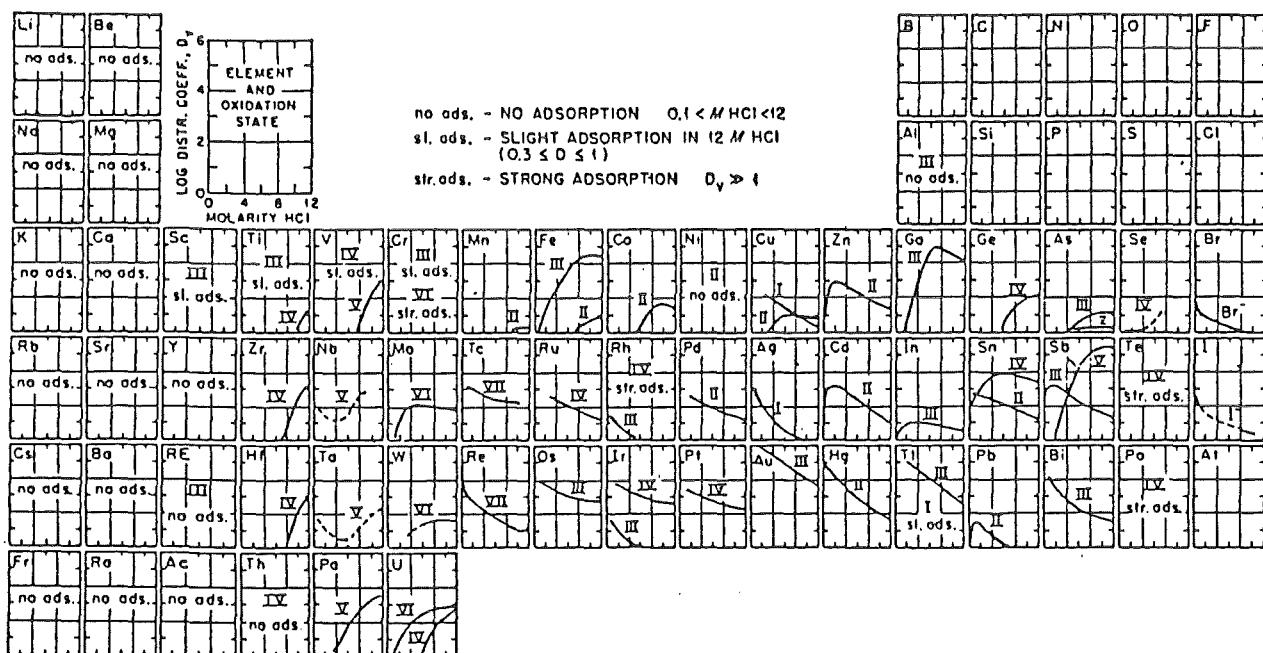
Figure 55: Adsorption of the Elements from Hydrochloric Acid
