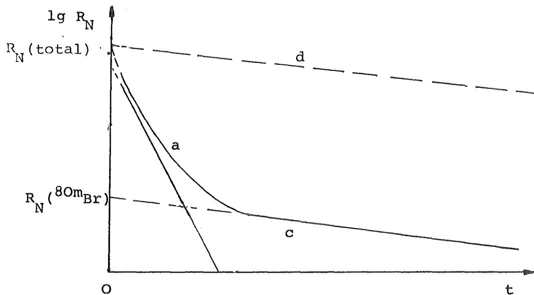
Figure 66: Decay Curve for the Isomeric System  $^{80}\text{Br}/{}^{80\text{m}}\text{Br}$
