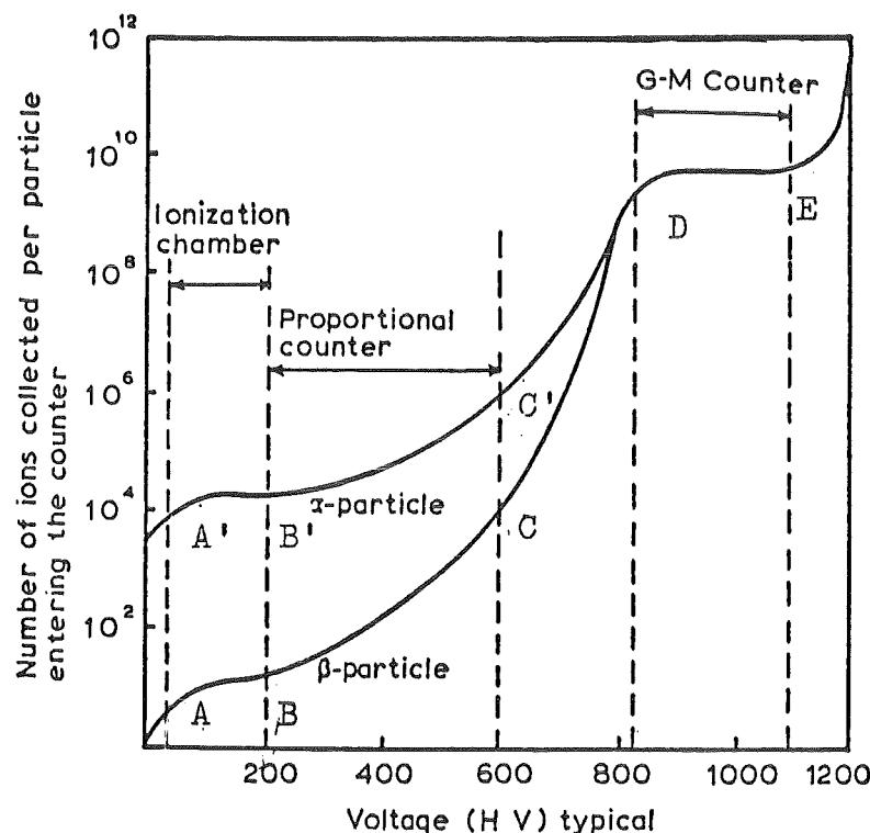
Figure 3: Ionization Curves against Applied Voltage
