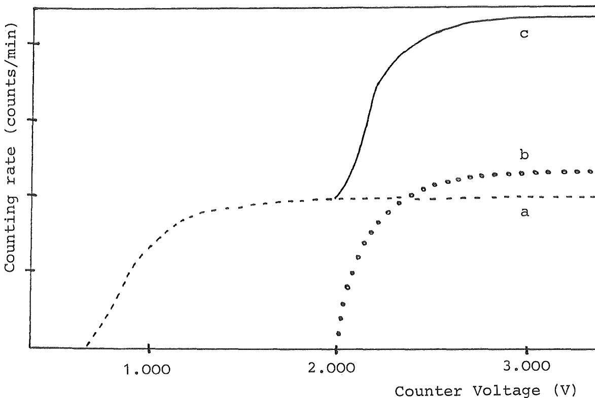
Figure 4: Characteristics of a Proportional Counter
