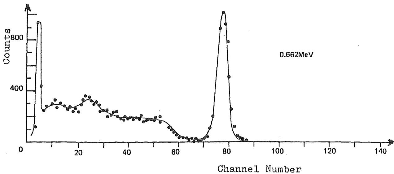
Figure 25:  $\gamma$ -ray Spectrum of  $^{137}\text{Cs}$
