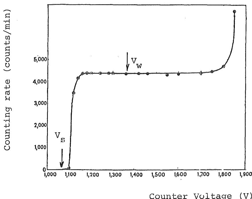
Figure 5: Characteristic of a Geiger-Müller Tube
