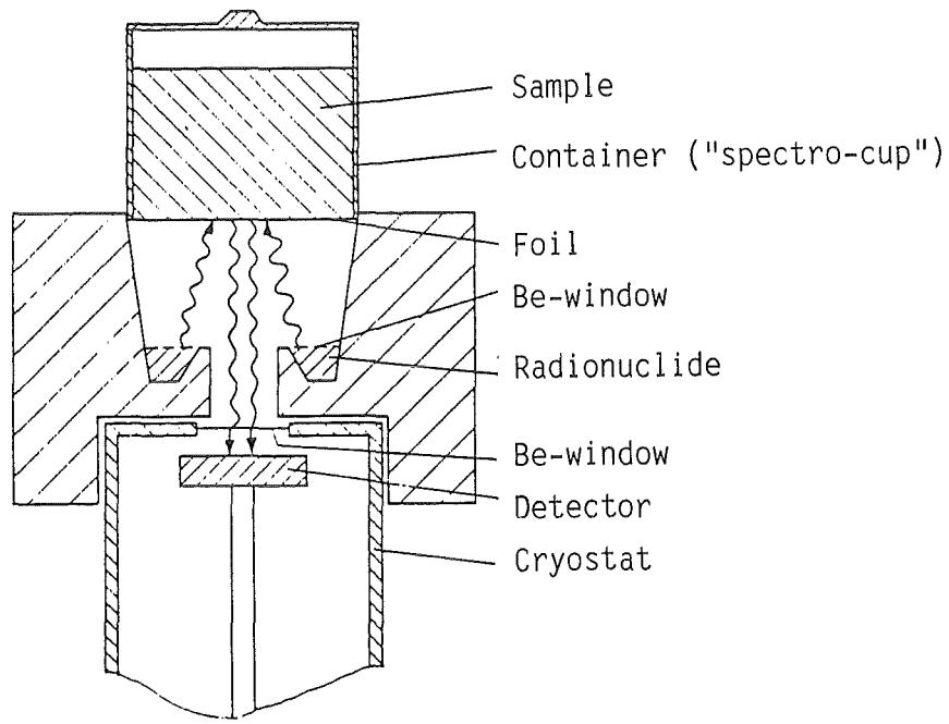
Figure 62: Radionuclide Activated XRF
