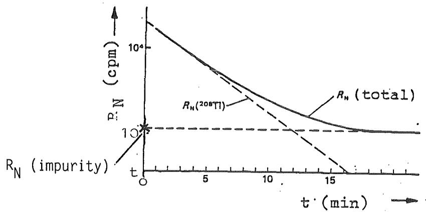
Figure 48: Decay Curve of  $^{208}\text{Tl}$
