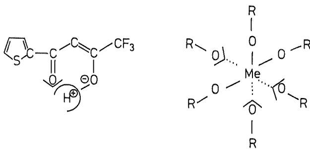
As neutral complex with a great organic residue structure the chelate formed is highly organophil and easily to be extracted into the organic phase. From the ions involved,  $\text{UO}_2^+$ ,  $\text{Th}^{4+}$ ,  $\text{Pa}^{5+}$  the highly positive charged Pa forms the most stable chelate and thus is extracted even in 4M acidic HCl-solution.
