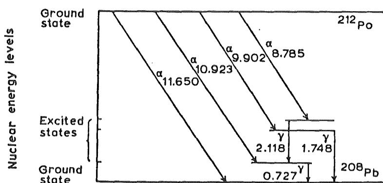
Figure 35:  $\alpha$ -decay of  $^{212}\text{Po}$  (the units are in MeV). The figure shows why  $\alpha$ -emission is frequently accompanied by  $\gamma$ -emission since the product nucleus, in this case  $^{208}\text{Pb}$ , may be in an excited state. The excess energy must be emitted as a  $\gamma$ -ray.
