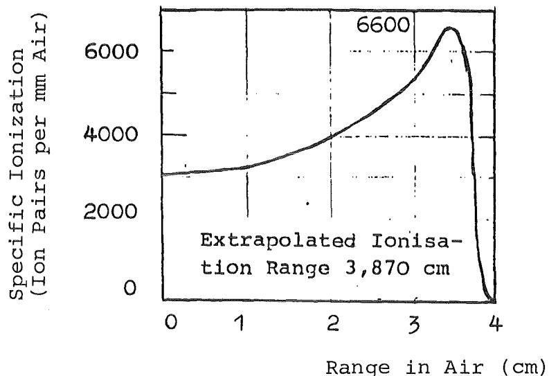
Figure 34: Specific Ionisation of  $\alpha$ -radiation of  $^{210}\text{Po}$  in Air as a Function of Way (Bragg Curve)
