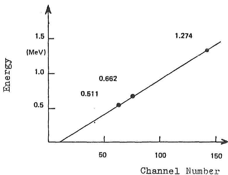
Figure 28: Energy Calibration Curve
