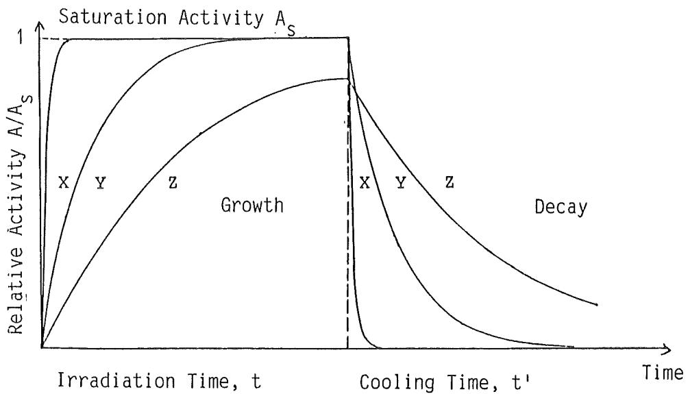
Figure 57b: Growth and Decay of Radionuclides
