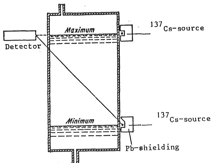
Figure 58: Arrangement for Measurement of Liquid Levels
