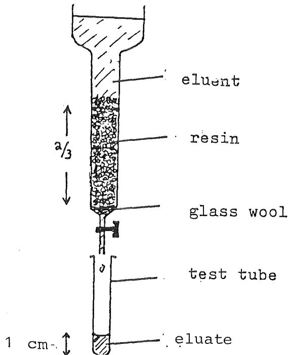
Figure 56: Ion Exchange Column
