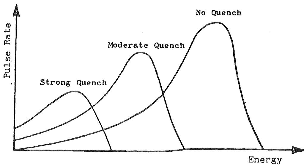
Figure 29: Spectra of Different Quenched  $^{14}\text{C}$ -samples
