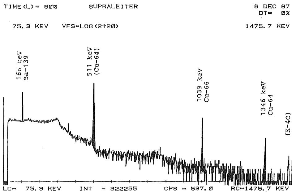
Figure 57d:  $\gamma$ -Spectrum of a n-activated "Warm Superconductor" (Y-Ba-Cu-Oxide, irradiation time 16 h, no cooling time, measuring time 10 m)
