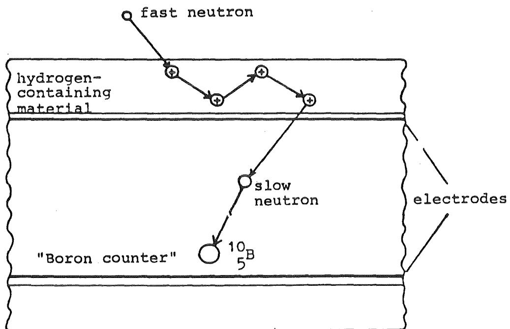
Figure 38: Detection of Neutrons: Boron Counter
