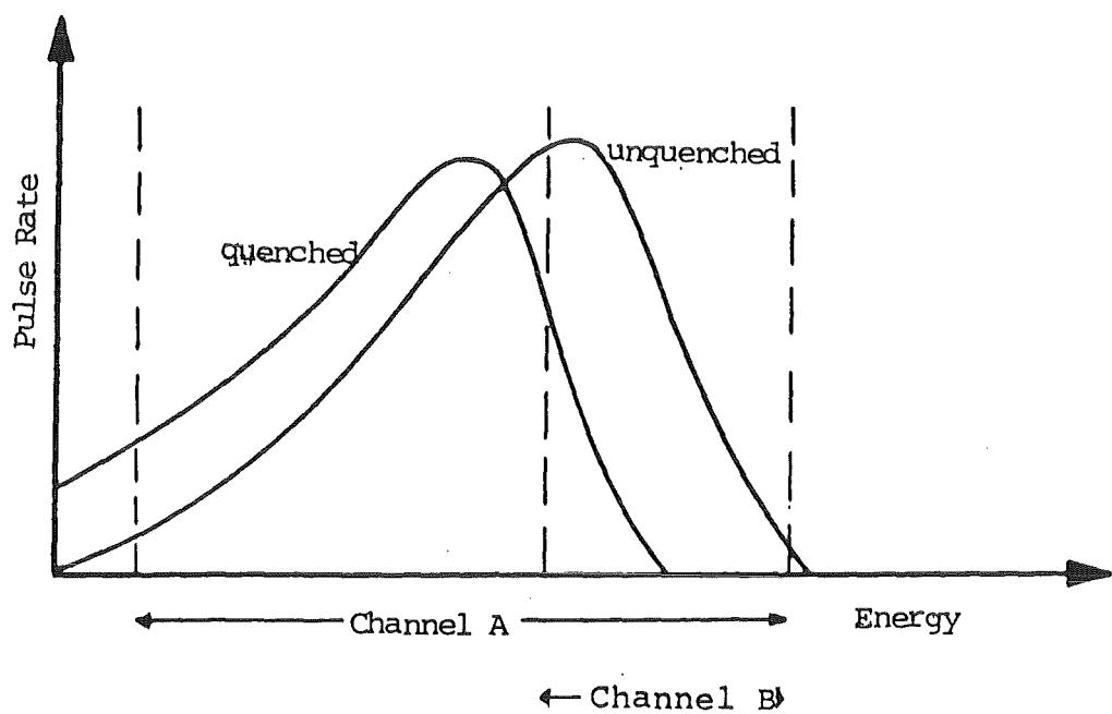
Figure 30: Channel Setting for Quench Correction by Channel Ratio
