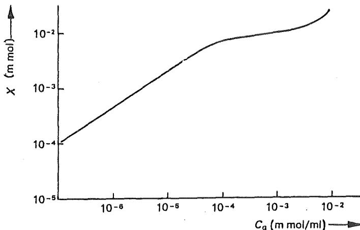
Figure 49: Adsorbed Amount of Phosphate  $X$  vs. Equilibrium concentration of Phosphate  $C_G$
