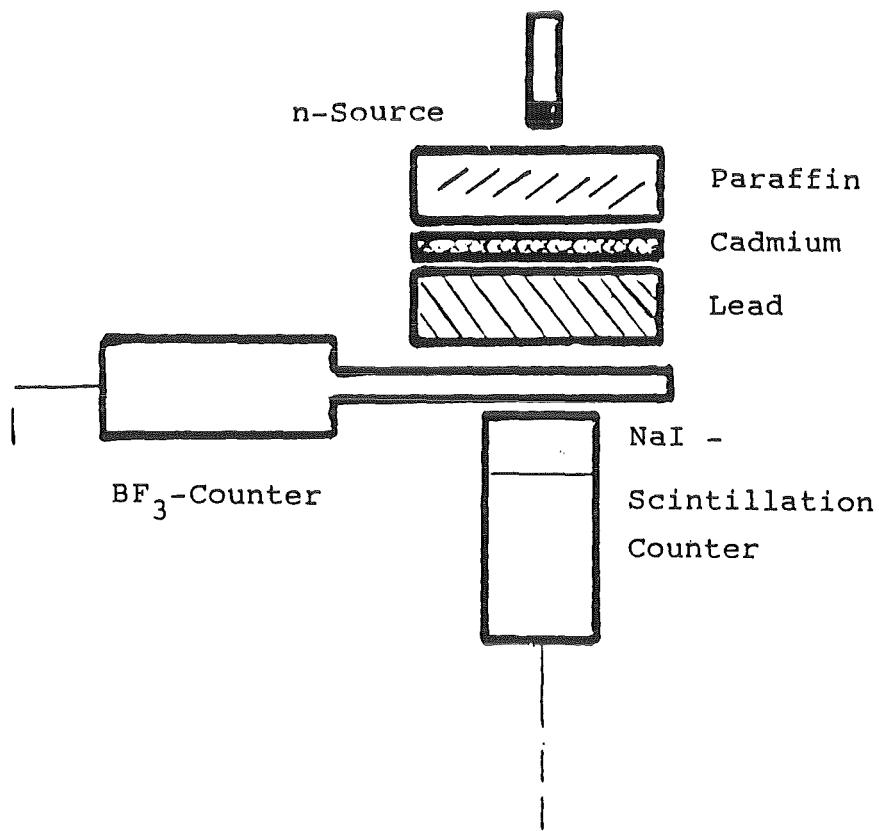
Figure 40: Experimental Arrangement for Moderation and Absorption of Neutrons
