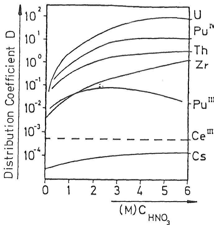
Figure 52: Distribution Coefficients for Fissionable Nuclides and Fission Products vs.  $\text{HNO}_3$ -concentration (metal concentration  $\gg 0.1 \text{ Mol/l}$ , 30% TBP in kerosene)
