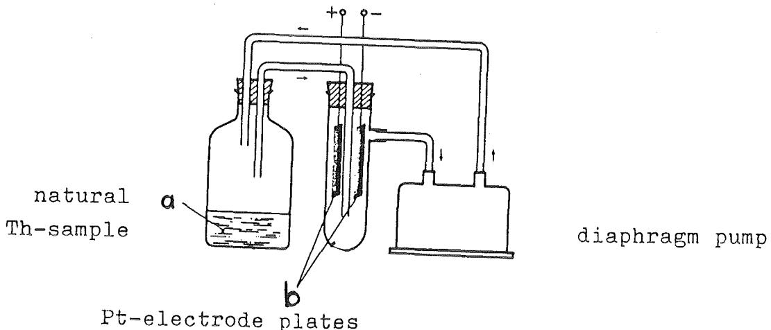
Figure 47: Arrangement for Electrodeposition of Carrier-free  $^{212}\text{Pb}$  From Natural Thorium ("Thorium Cow")
