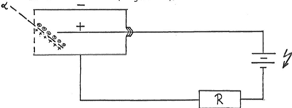
Figure 2: Circuit Diagram of a Gas Counter
