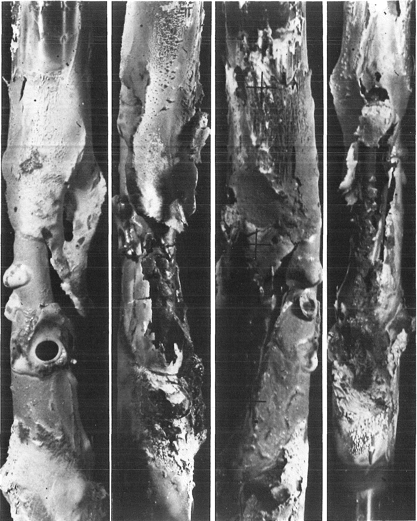
FIG. 53: DETAILS OF THE ESSI-7 FUEL ROD SIMULATOR AND SHROUD
