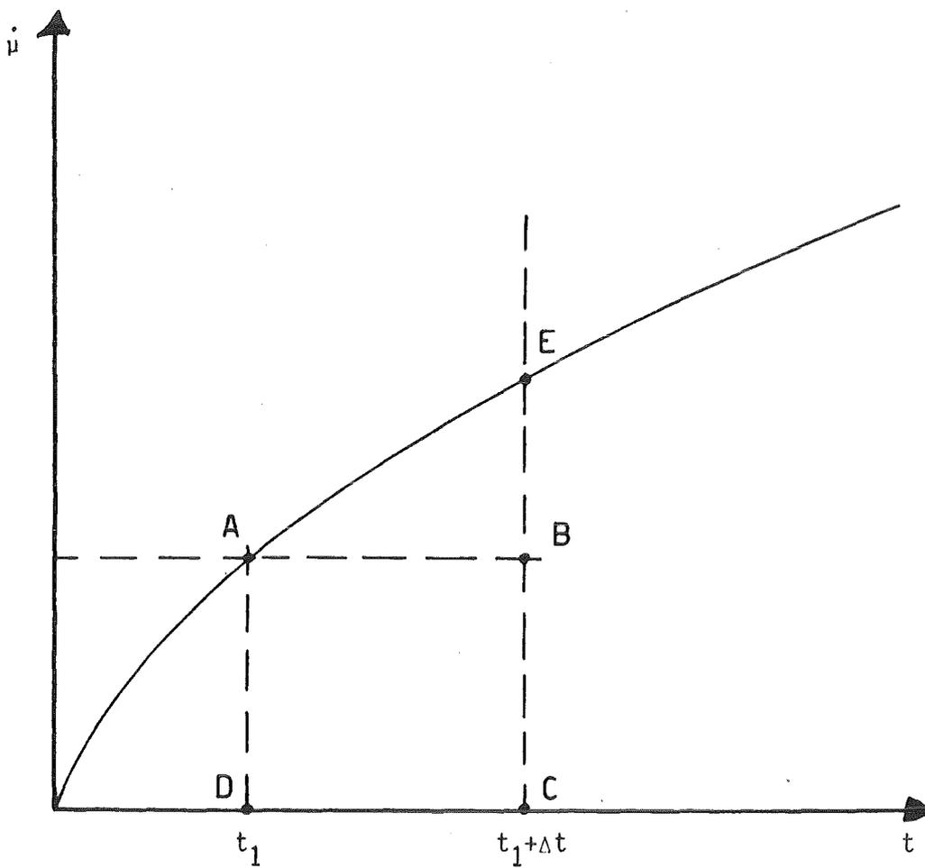
Fig. 1.1 Mass transfer rate for bubble growth
