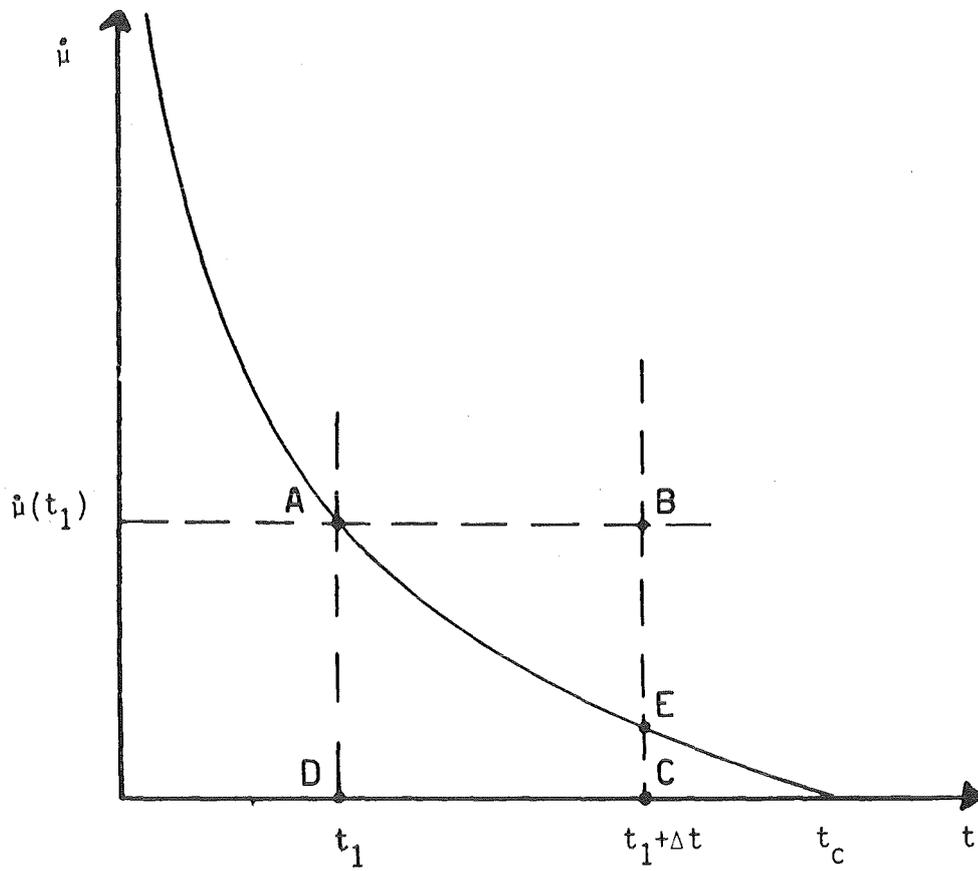
Fig. 1.2 Mass transfer rate for bubble collapse
