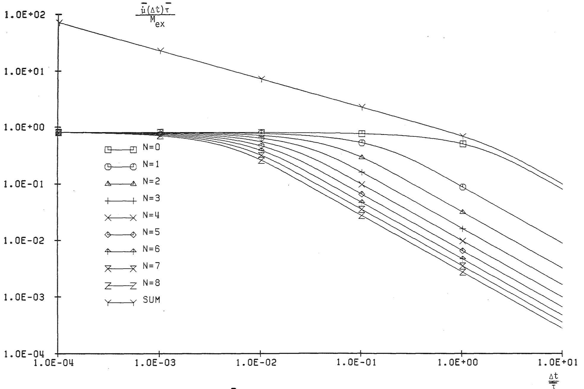
Fig. 4.6 Average mass transfer rate  $\bar{u}(\Delta t)$ .
