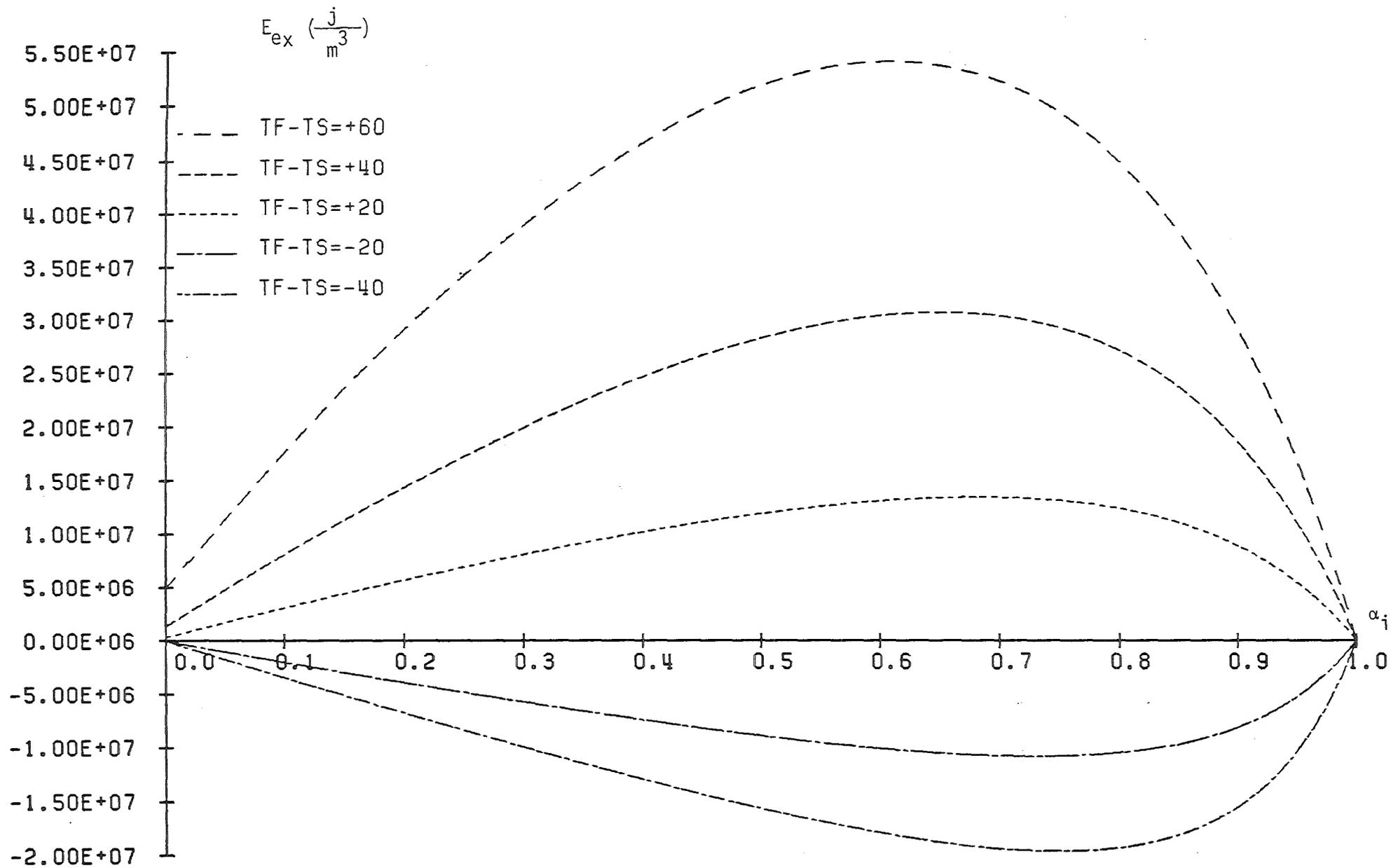
Fig. 2.4 Energy exchange at  $5.E6$  PA ( $T_g - T_s = 0$ )
