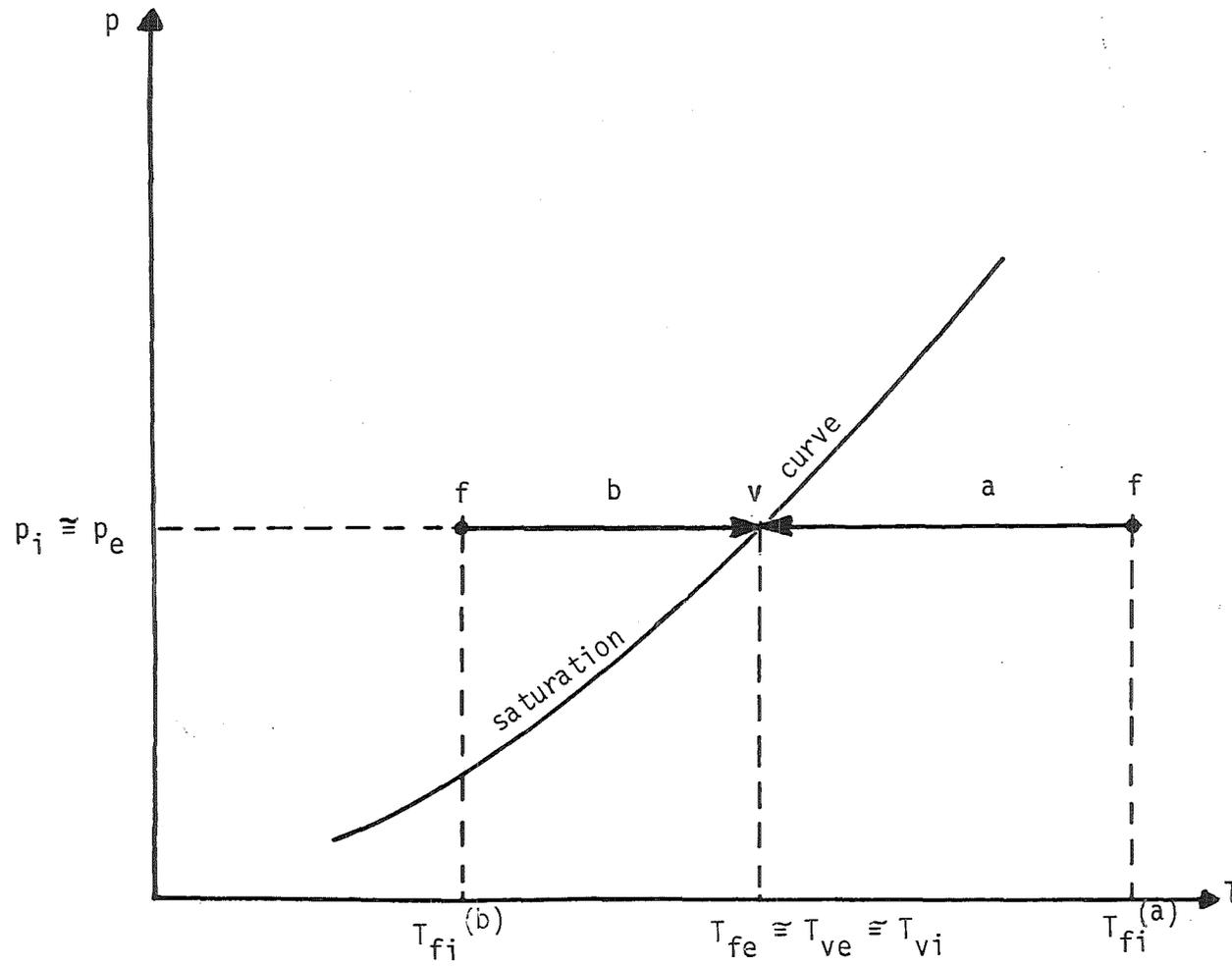
Fig. 4.1 Models for evaporation (a) and condensation (b)
