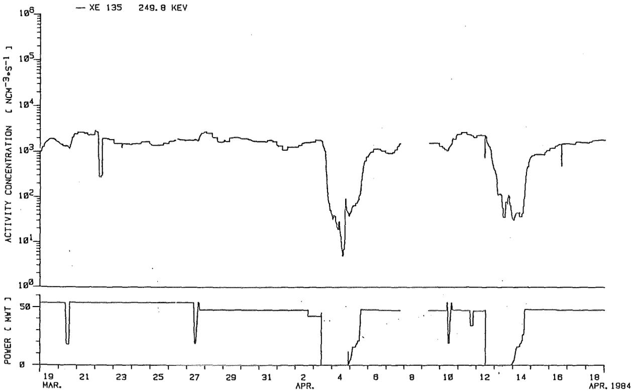
KNK II/2 EXPERIMENT: YE 705-511/8 BORE HOLE .1 MM\*\*2 UPPER PLENUM 12 PELLETS
