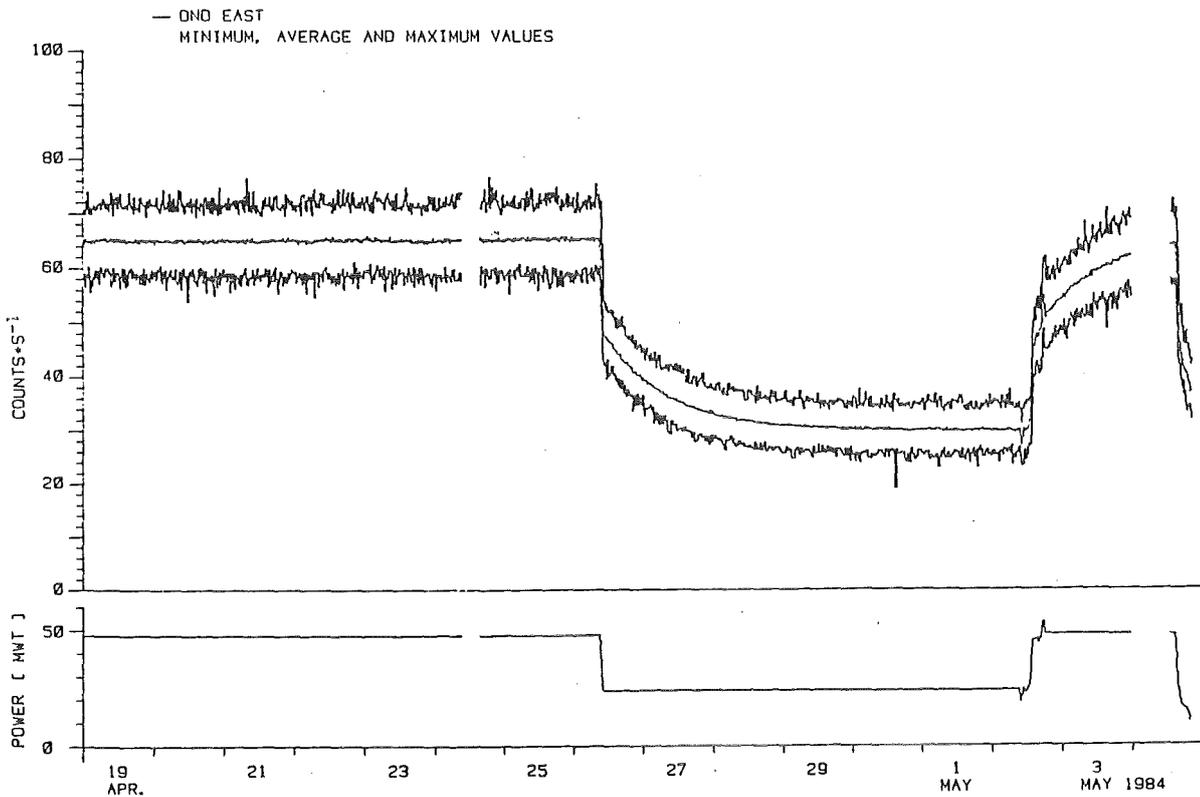
KNK II/2 EXPERIMENT: YE 705-511/8 BORE HOLE .1 MM\*\*2 UPPER PLENUM 12 PELLETS
