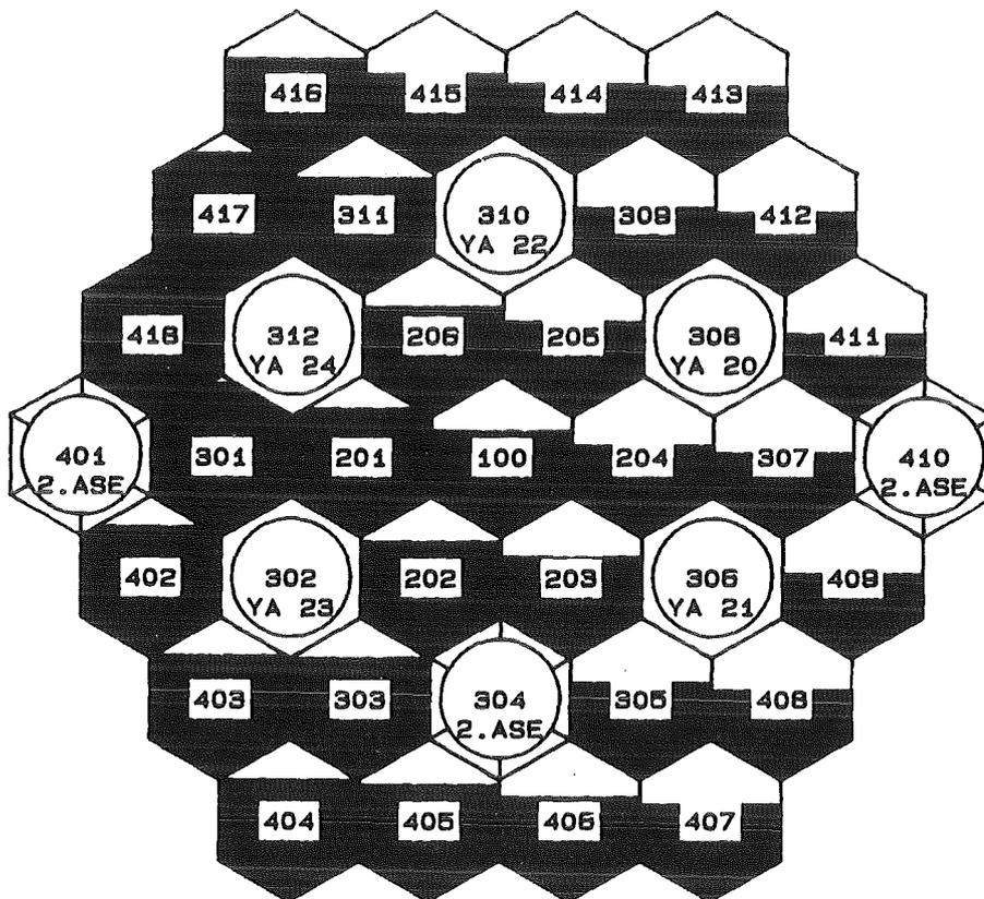
Fig. 10: Core Cross Section KNK II, Flux Tilting Result
