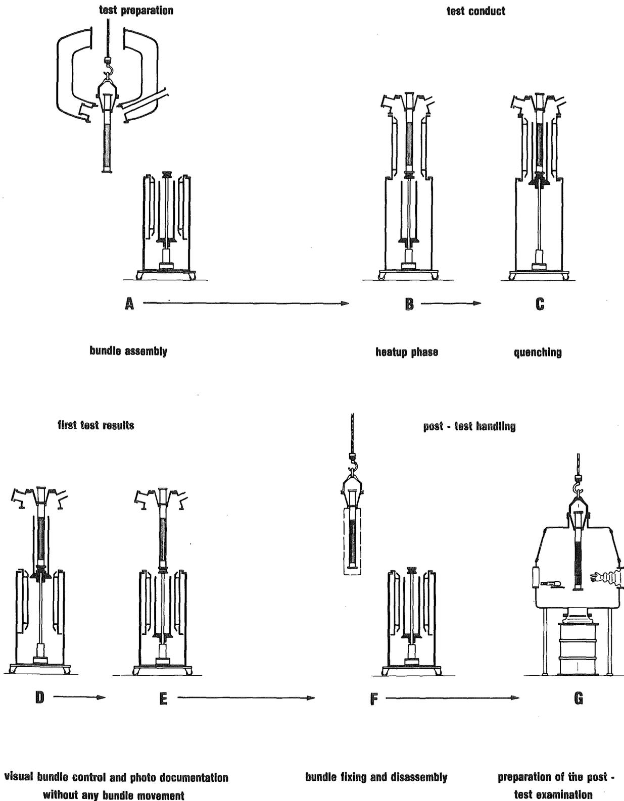
**Fig. 3: SFD Test facility CORA, Testing sequence**
