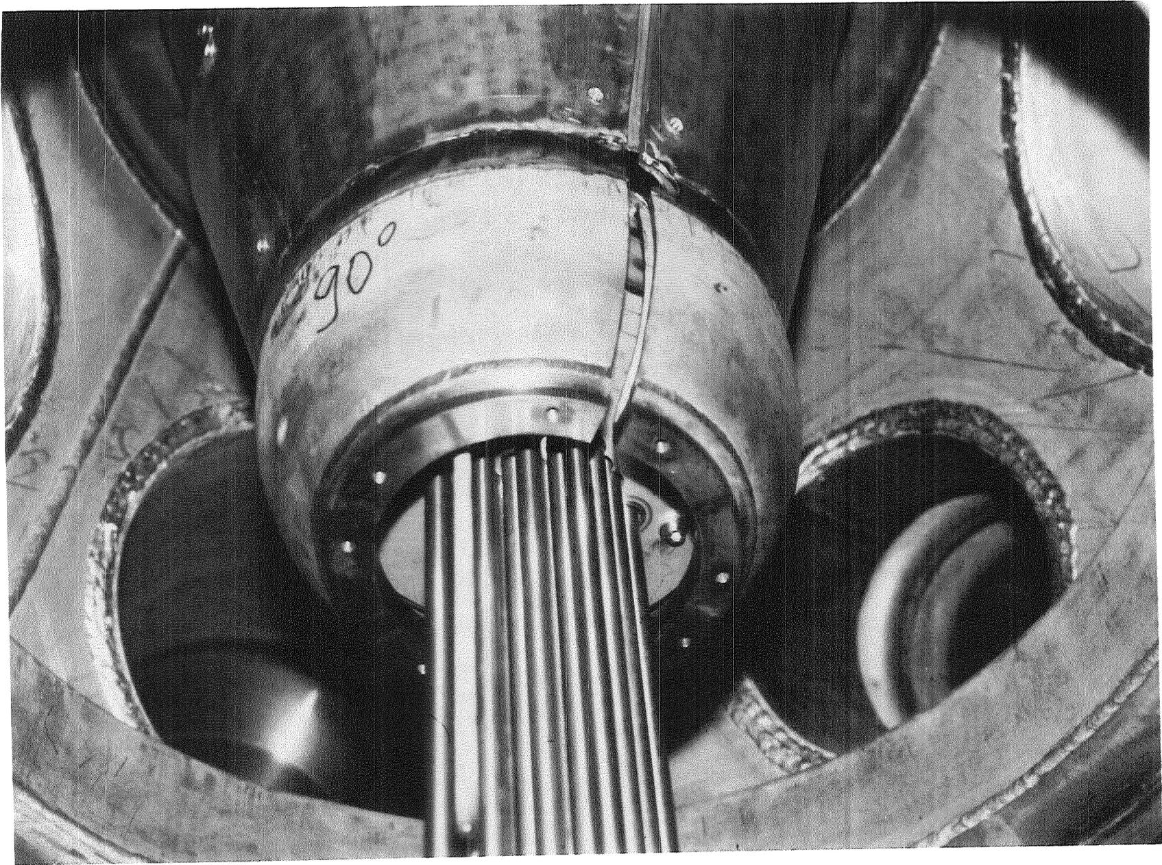
Fig. 14: BUNDLE UPPER END WITH RADIATION SHIELDS FOR HEAD PLATE
