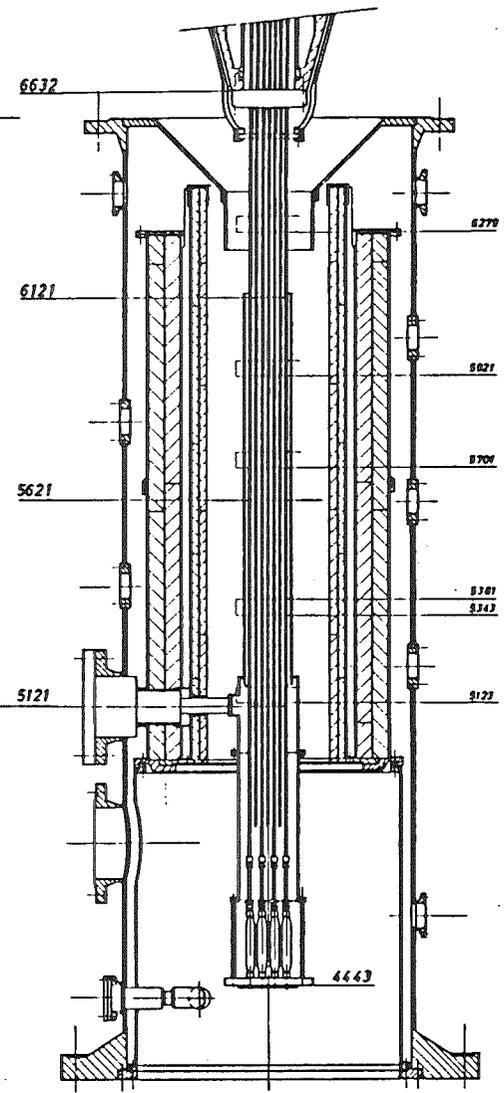
Fig. 8: CORA Bundle and High Temperature Shield Assembly
