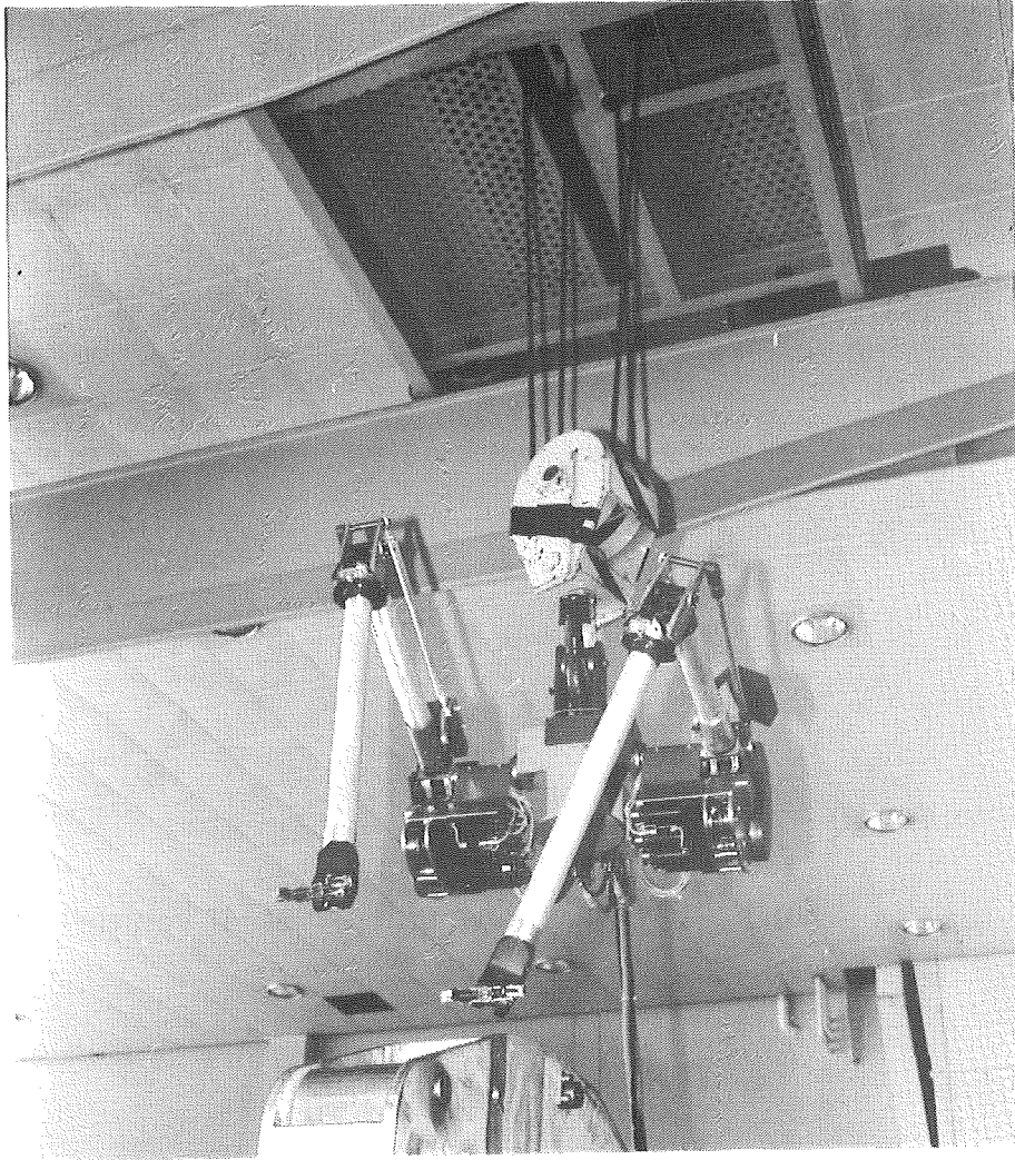
Fig. 10 "EMSM 2" slave unit on a bridge crane
