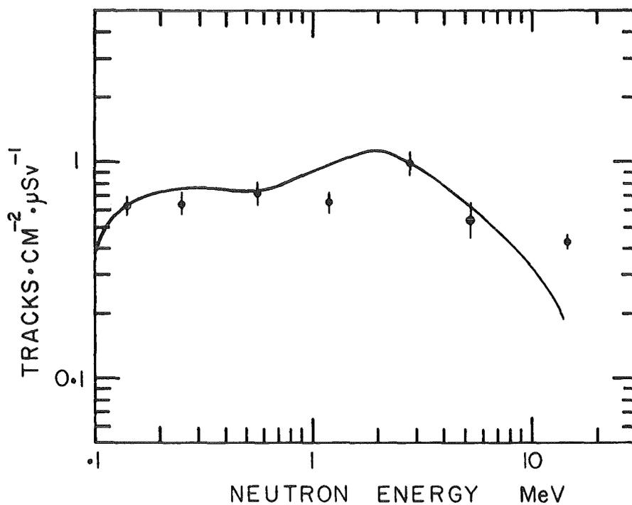
Fig. 1. Measured and calculated response of CR-39. The curve is calculated on the assumptions that only recoil protons of energies between 0.08 and 2.75 MeV produce visible tracks.
