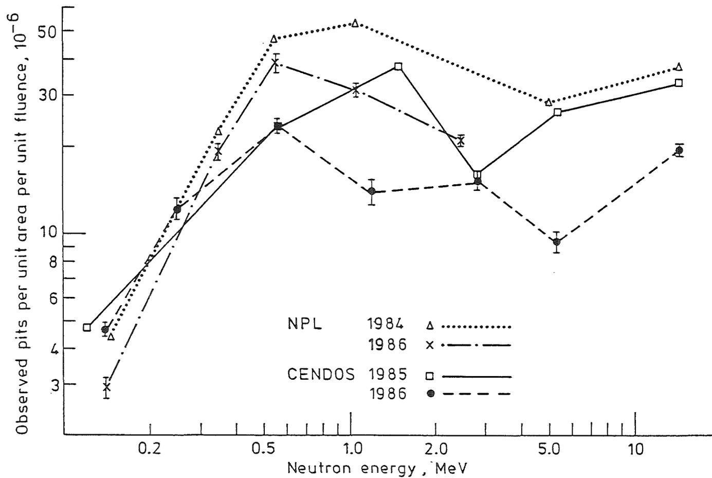
Figure 1 : Dosimeter Response per Unit Fluence
