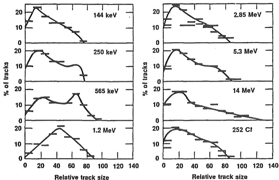
Fig. 2 The track-size distribution obtained from the CR-39 foils exposed in this study.
