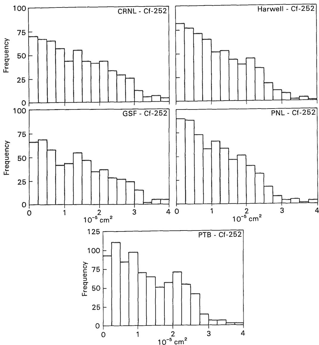
FIGURE 1. Track Size Distributions of CR-39 Exposed to Cf-252 Sources from Various Irradiation Facilities (not normalized for fluence)
