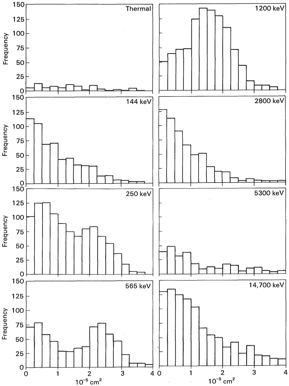
FIGURE 2. Track Size Distributions for the Indicated Neutron Energies (not normalized for fluence)
