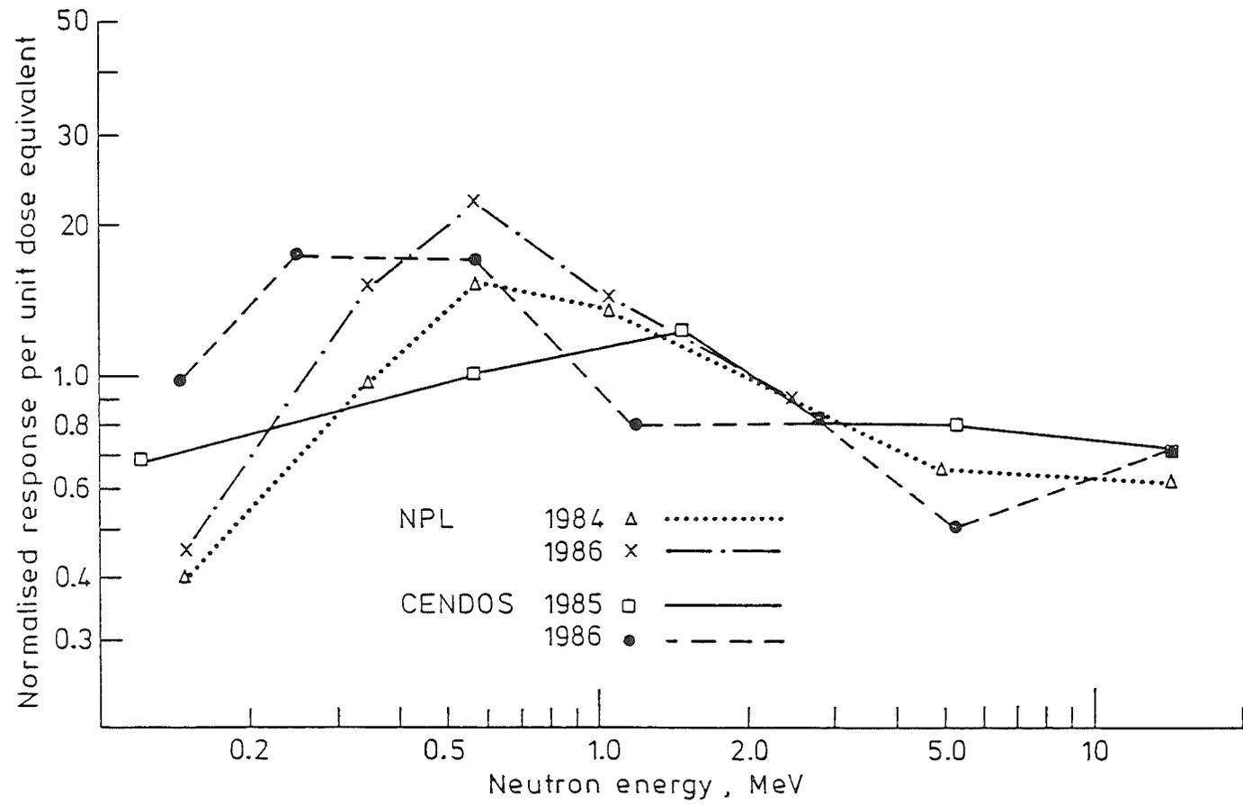
Figure 2 : Dosimeter Response per Unit Dose Equivalent (ICRP 51 H\*(10))
