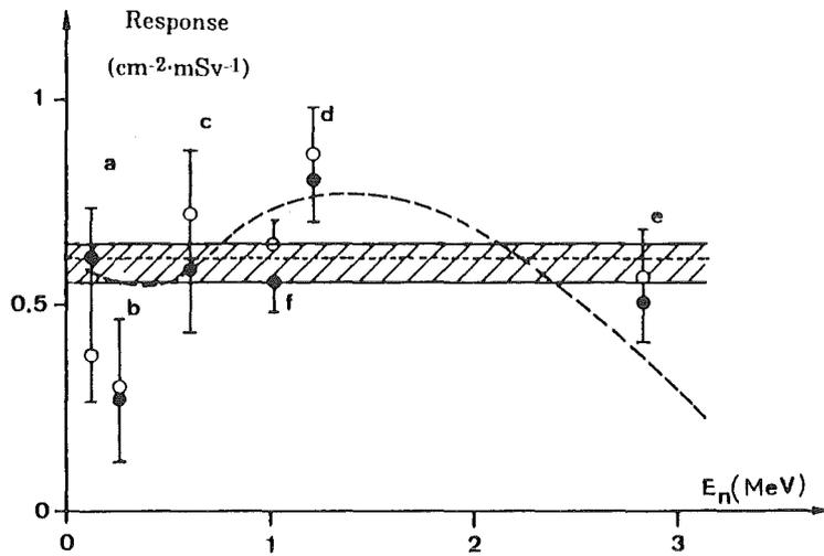
Figure n°2 : Response (-effective efficiency) as a function of neutron energy for normal incidence - radiator thickness : 35  $\mu\text{m}$
