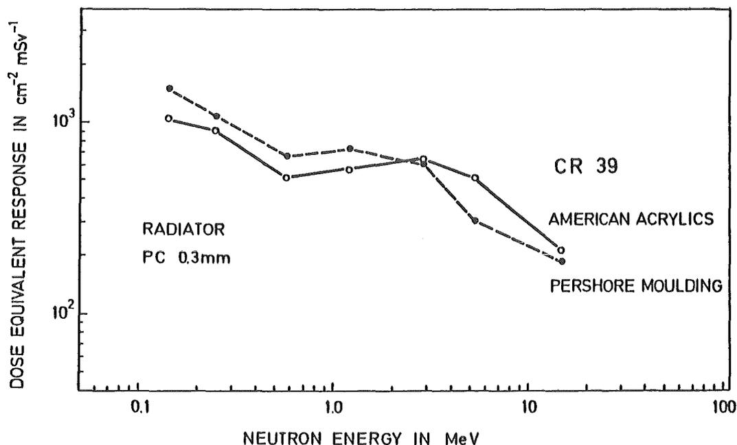
Fig. 1 Energy response of ECE etched CR 39 manufactured by American Acrylics and Pershore Moulding Ltd. with 0.3 mm polycarbonate as radiator
