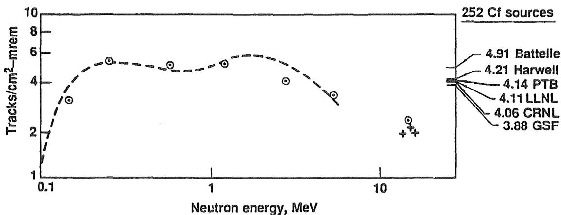
Fig. 1 The results obtained in this study are shown as open circles and the dashed line is the energy dependence curve. The result with the various Cf sources are also shown.
