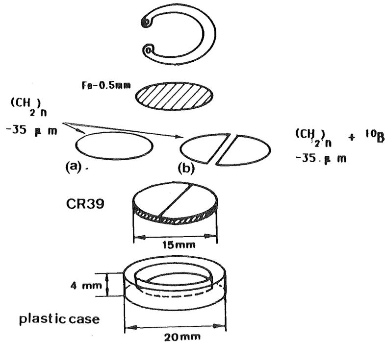
Figure n°1: Dosemeter used for -a) fast neutron detection with or without polyethylene (35μm) radiator - b) thermal neutron detection
