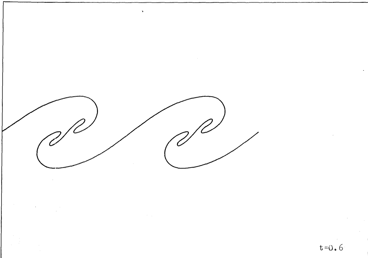
Fig. 6.9: Numerical simulation of a Kelvin-Helmholtz instability with a large amplitude at time t = 0.4, 0.6
