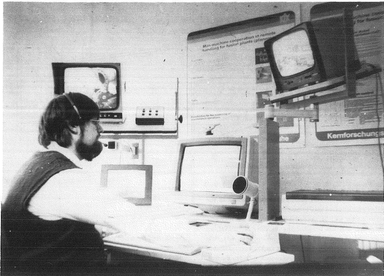
Fig. 63: Experimental man-machine interface set-up: graphics, TV (graphics controlled camera) touch screen, sensor ball, mouse, loudspeaker, microphone
