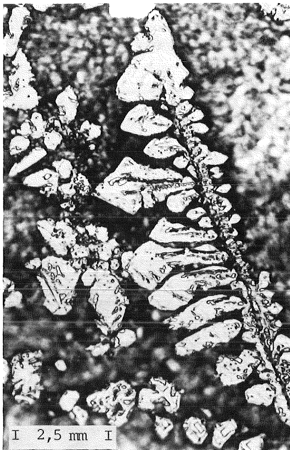
Fig. 9: Appearance of deposited crystals in the magnetic trap of PICOLO
