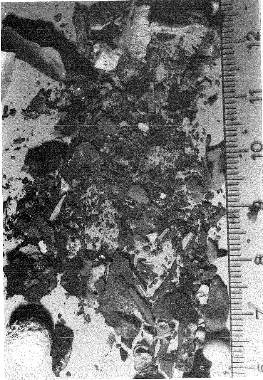
Fig. 113: Rubble from lower plates of CORA bundle B
