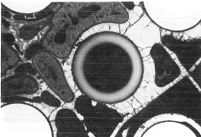
Fig.156: Enlarged cross sections in region of unheated rods at -55 mm elevation (CORA bundle B)
