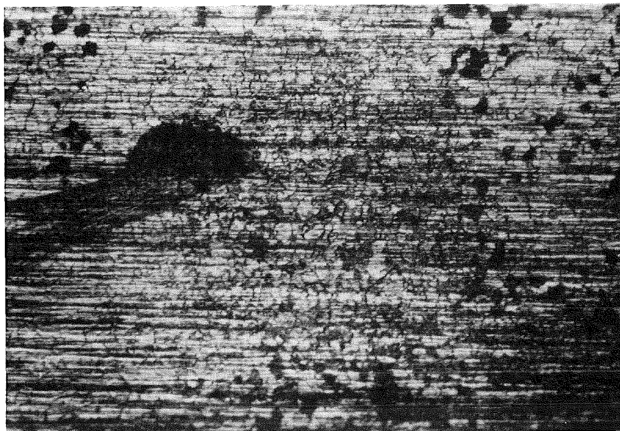
Fig. 7 Light microscopic photograph of the ion bombarded area of sample No. 2 after measurement of the AES depth profile. The slightly brighter square in the center of the photograph represents the sputtered part of the surface. The dark spot in the upper left of the photograph corresponds to a mechanical damage of the surface which occurred after the depth profile measurement (magnification x 50).
