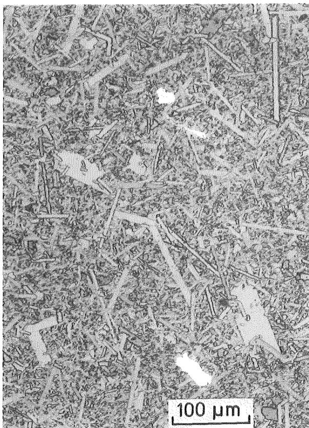
Fig. 44: Microstructure of hot-pressed SiC with 0.7 % B.
