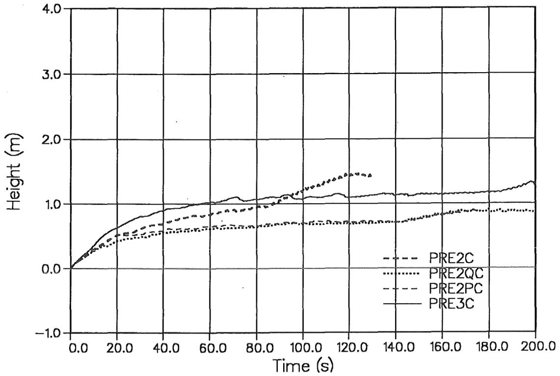
Figure 13. Comparison of Collapsed Water Level.
