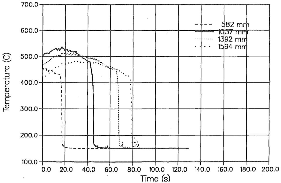
Figure 6. Cladding Temperature versus Time (PRE2C).
