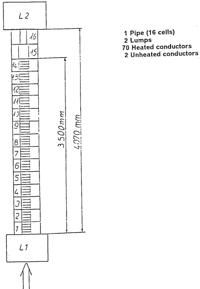
Figure 4. FLUT-Nodalisation of the FLORESTAN 3-Test Section.
