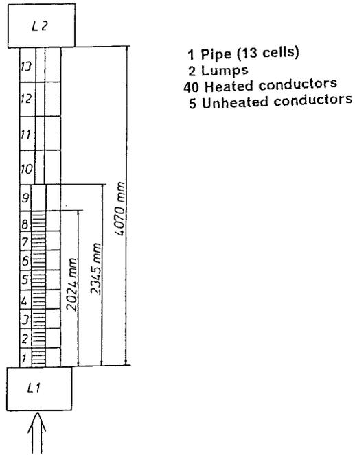
Figure 3. FLUT-Nodalisation of the FLORESTAN 2-Test Section.
