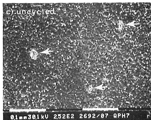
Fig. 38: Zr-precipitates (arrows) near the surface initiate fatigue cracking in MANET 1.
