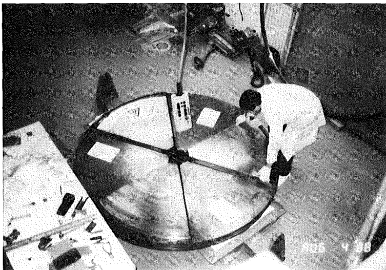
Fig. 2 Installation of the new correction coil base on the lower pole tip.
