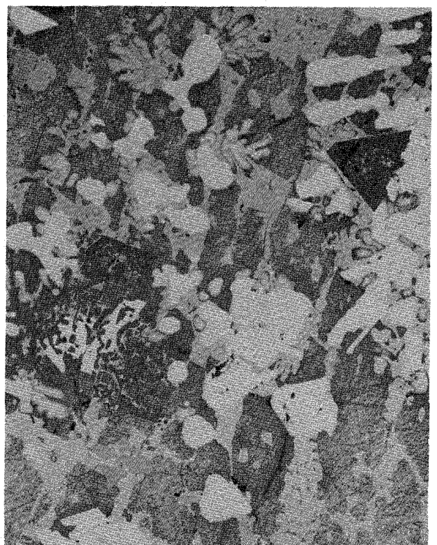
Fig. 76. Mo- and W-rich ("bright") melt, from interference with heater rod electrode, and pellet attack at longitudinal section b of CORA-3
