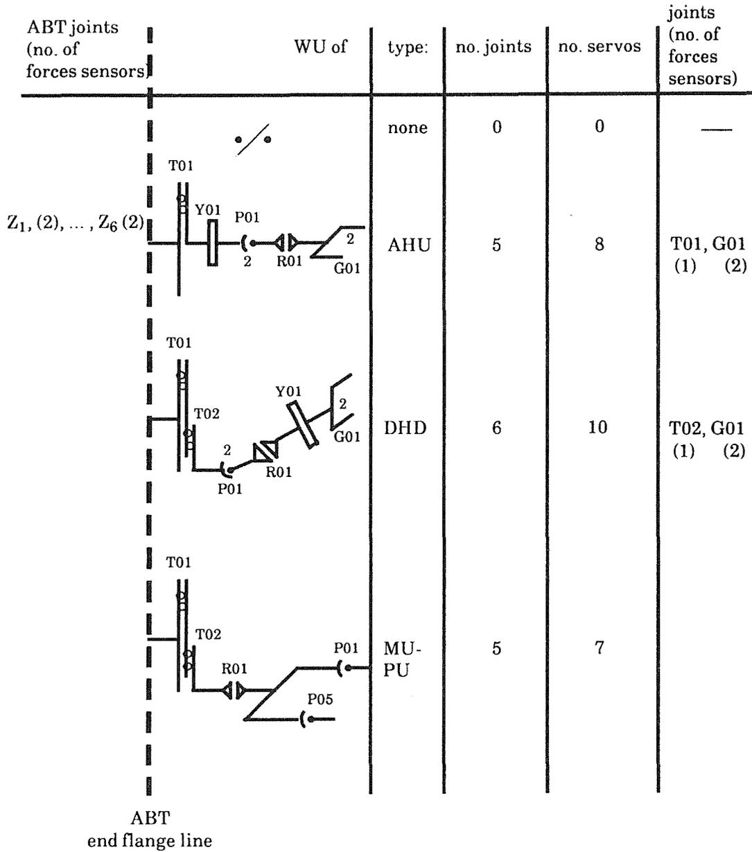
Fig. 3.3 EDITH - Configurations (kinematic structures)
