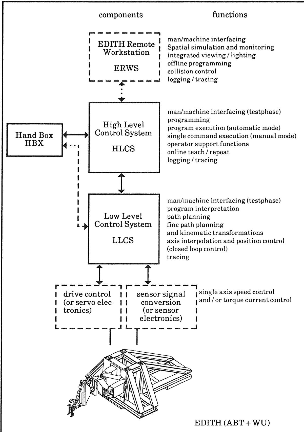
Fig. 4.2 EDITH control system architecture as resulting from the TARM control system
