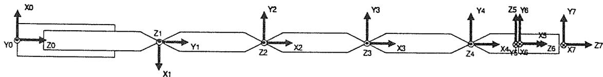
Note 1: Z0 is a virtual prismatic axis; all real rotational axis and their corresponding coordinate systems K1 to K4 have to be attached in such a way, that K0 is taken into account. This measure is taken to allow for an inclusion of the real Z0 axis of the ABS without redefintion of coordinate systems.
