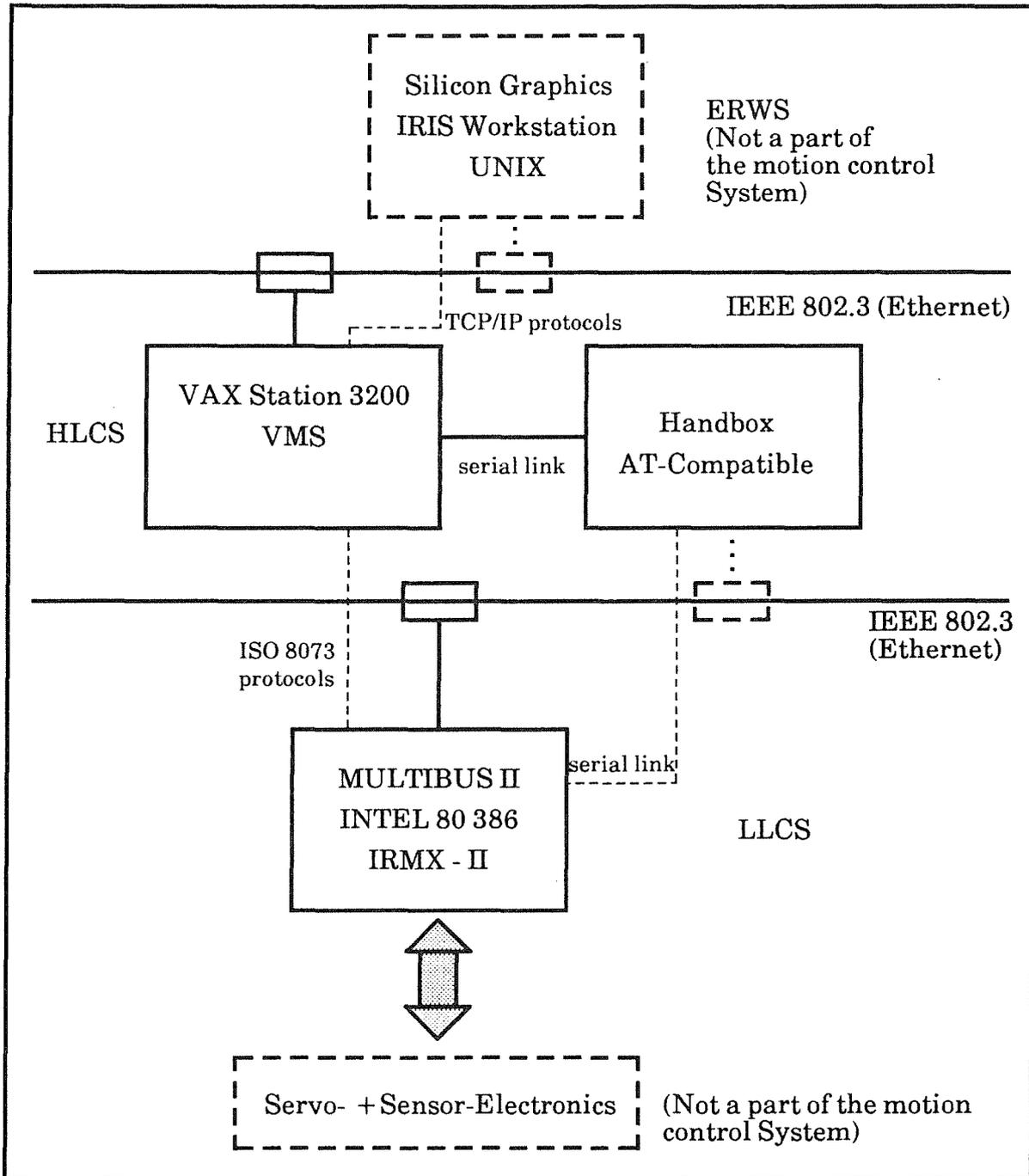
Fig. 4.3 EDITH Control System: Hardware Architecture
