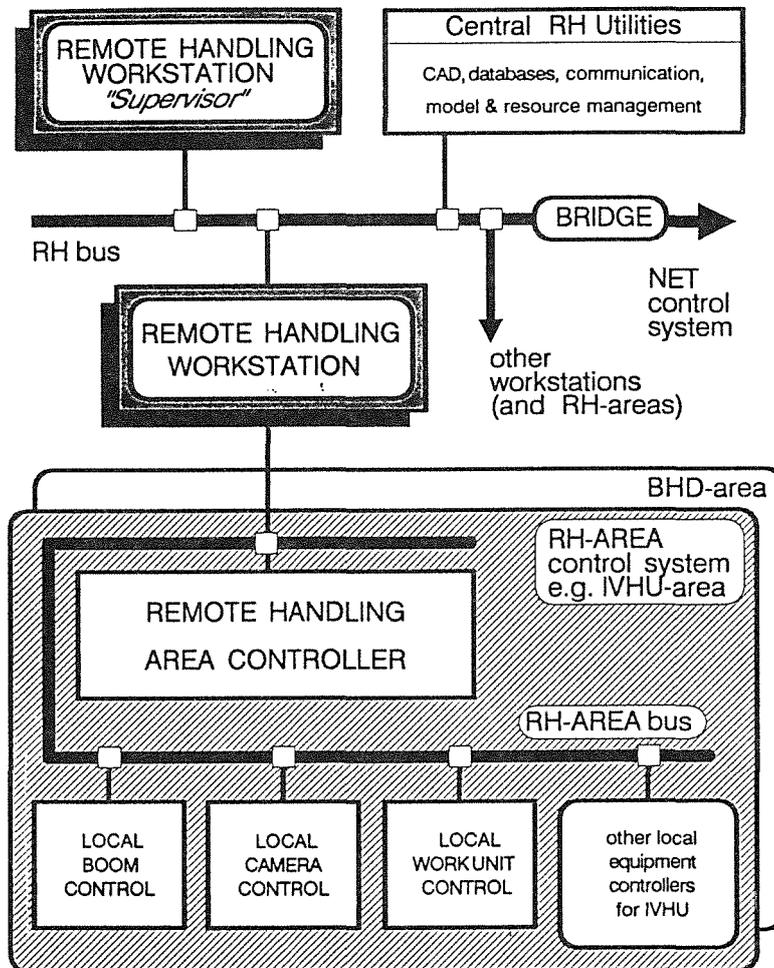
Fig. 4.1 Overall remote handling control system architecture for NET
