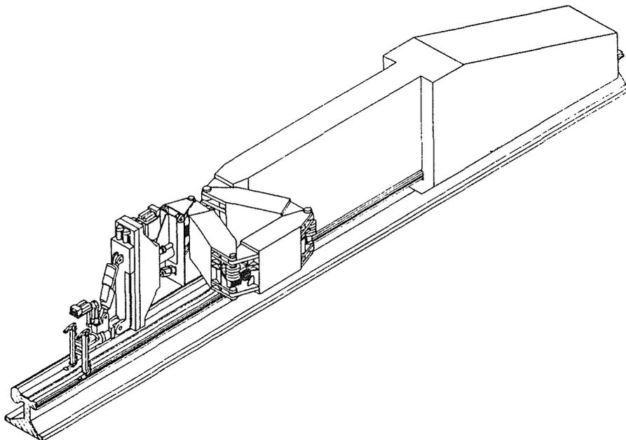
Fig. 1.2 Antenna handling unit (AHU)
