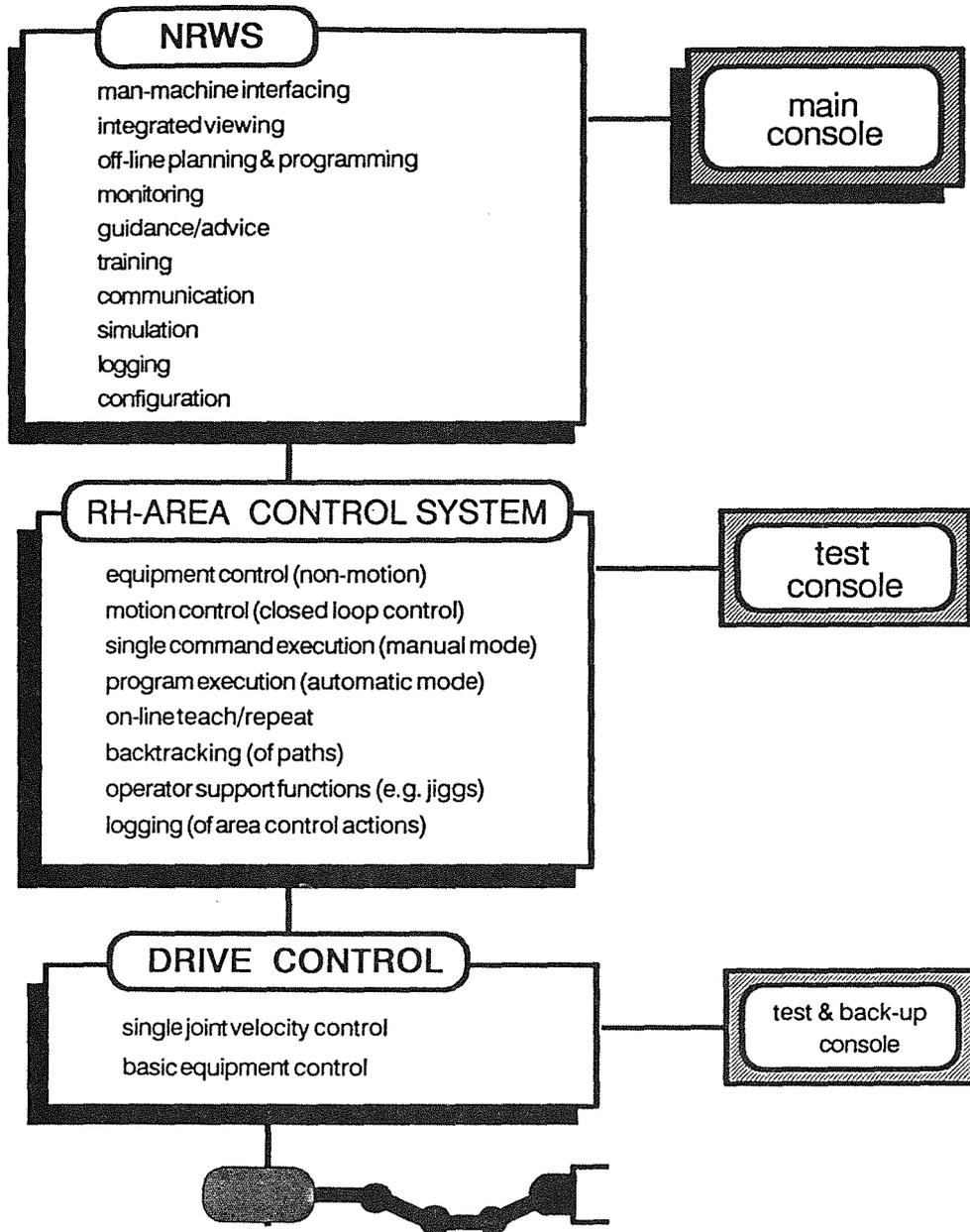
Figure 2.1. Generic functionality of control system levels. The NRWS represents the task level support and the man-machine interface, the RH-area control system represents the motion control level functions.
