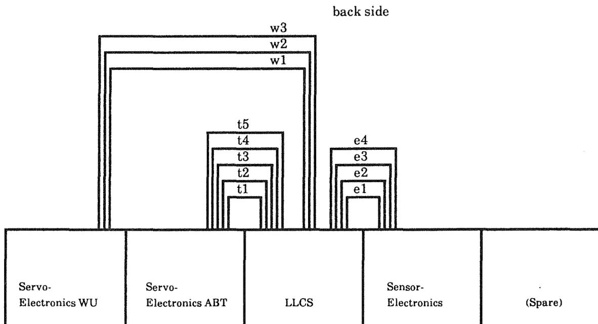
Fig. 6.1: Arrangement of control cabinets for the EDITH-Control-System (top view), Cable Connections
