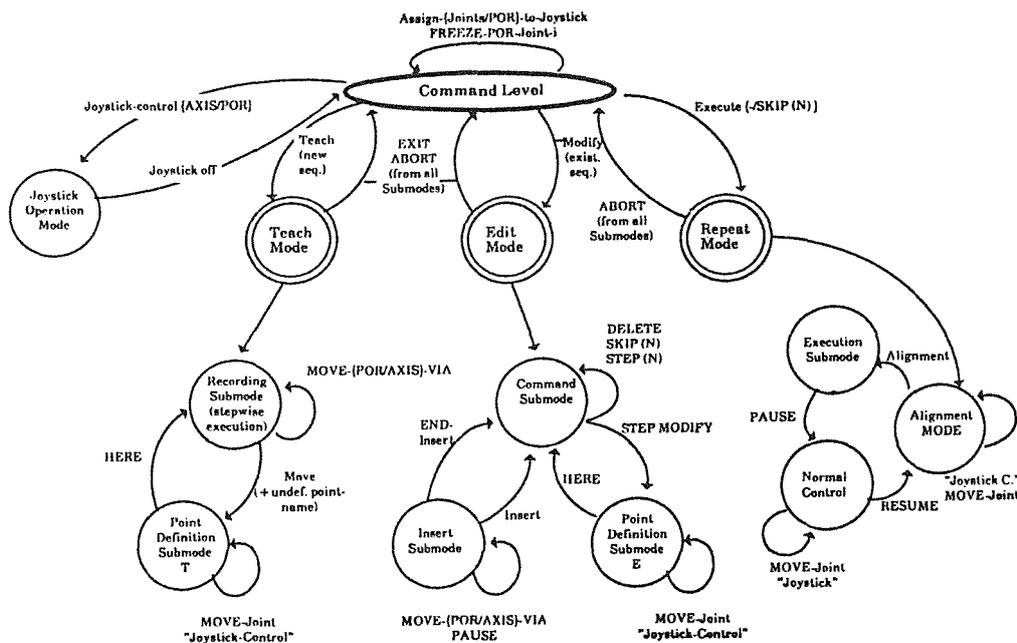
Fig. 8.1 Operational Functionality of the TARM Control System
