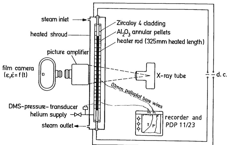
Fig. 3: Single-rod test rig
