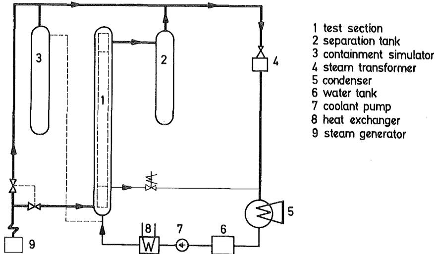
Fig. 4: Bundle test loop
