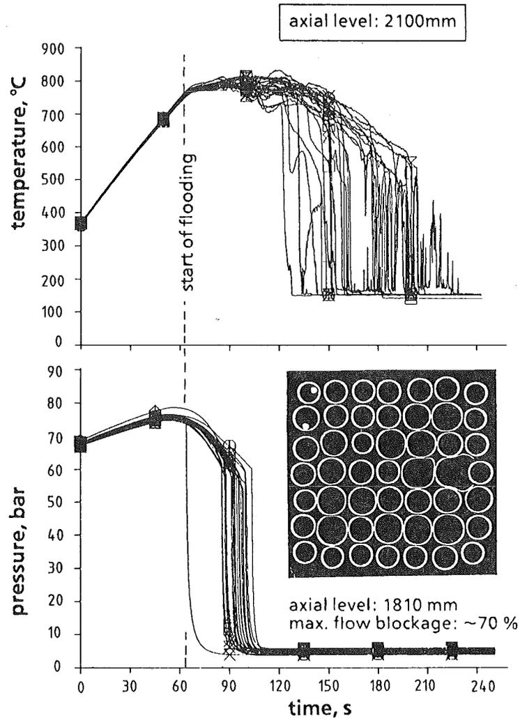
Fig. 13: Temperature and pressure transients of a 70 % blocked rod bundle (REBEKA 7)
