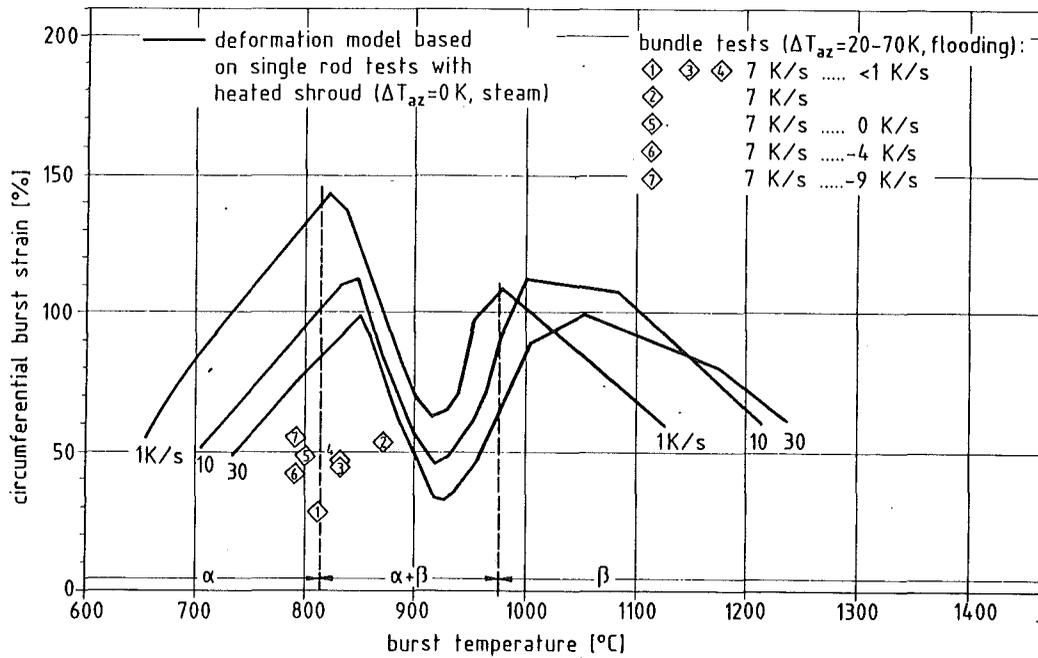
Fig. 8: Burst strain vs. burst temperature
