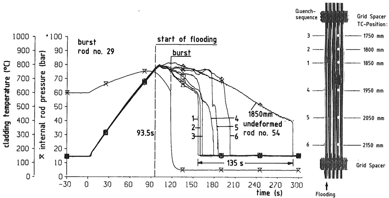
Fig. 14: Temperature transients and quenching behavior of a burst rod (REBEKA 6)
