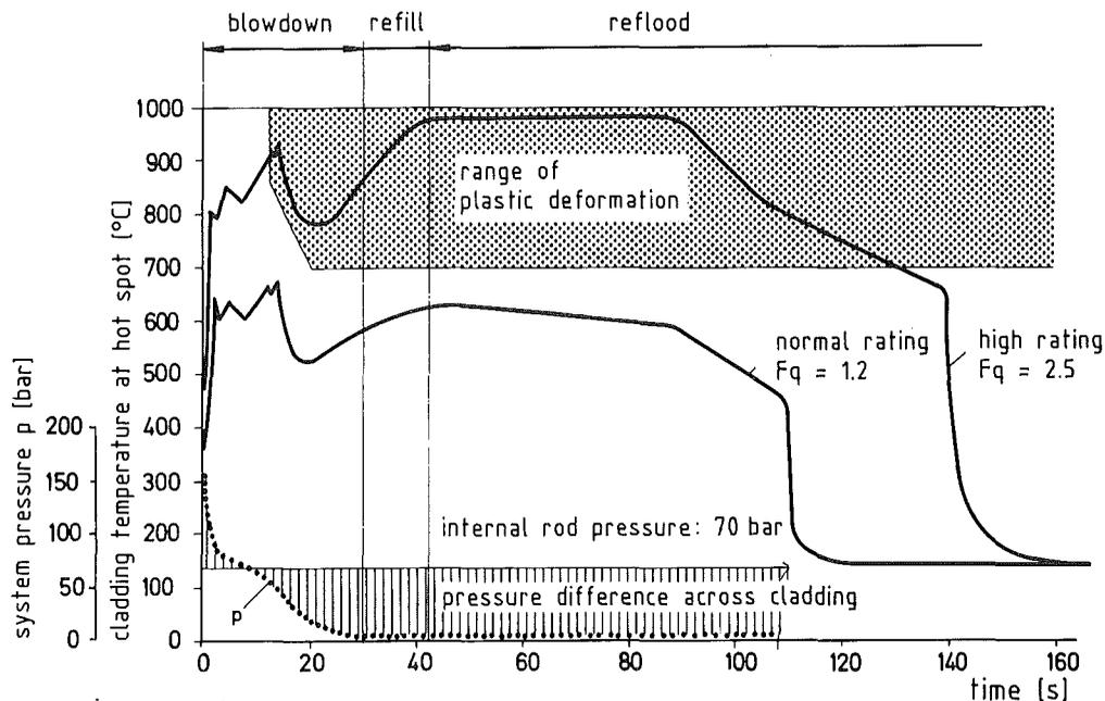
Fig. 1: Fuel rod cladding load in a double-ended cold leg break LOCA
