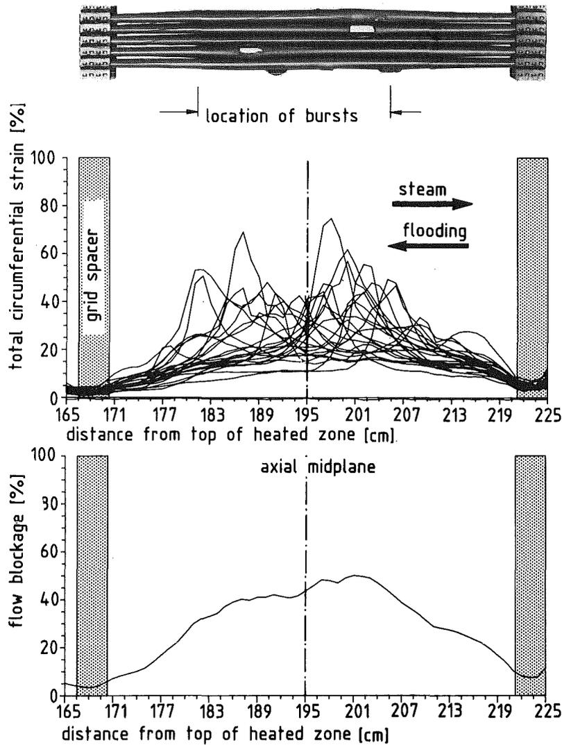
Fig. 11: Cladding deformation and flow blockage under reversed flow (REBEKA 5)
