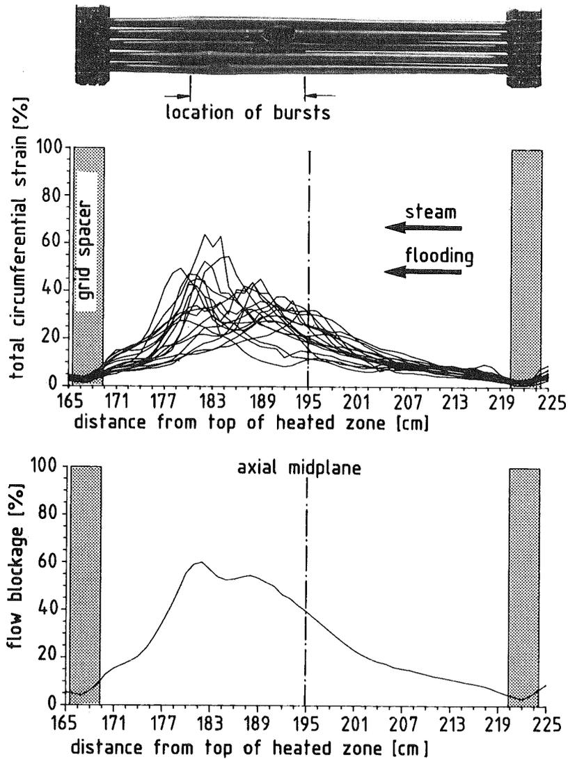
Fig. 12: Cladding deformation and flow blockage under unidirectional flow (REBEKA 6)
