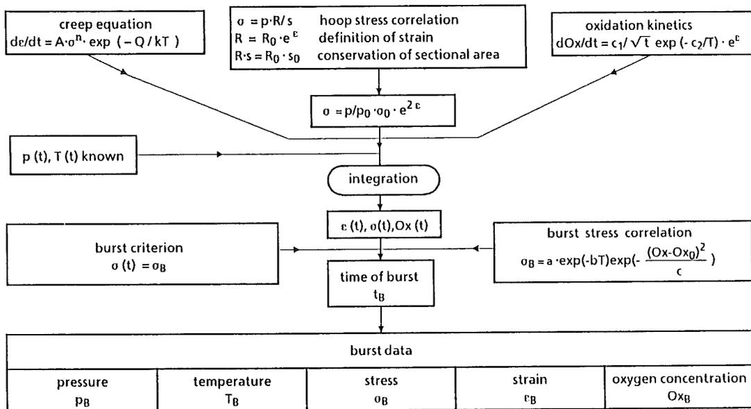
Fig. 6: REBEKA deformation model and burst criterion
