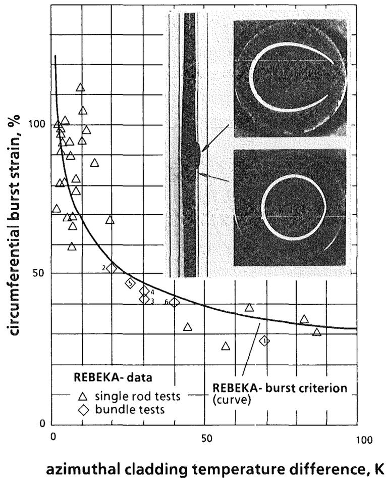
Fig. 9: Burst strain vs. azimuthal temperature difference
