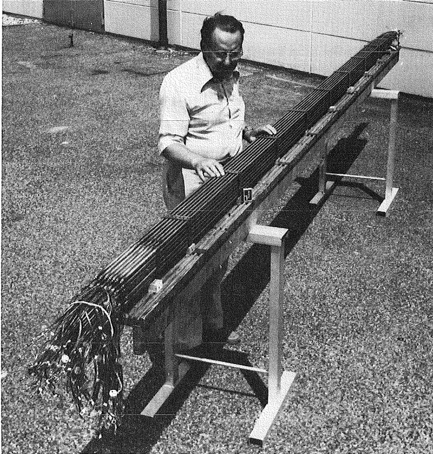
**Fig. 5: 49-rod test bundle**
