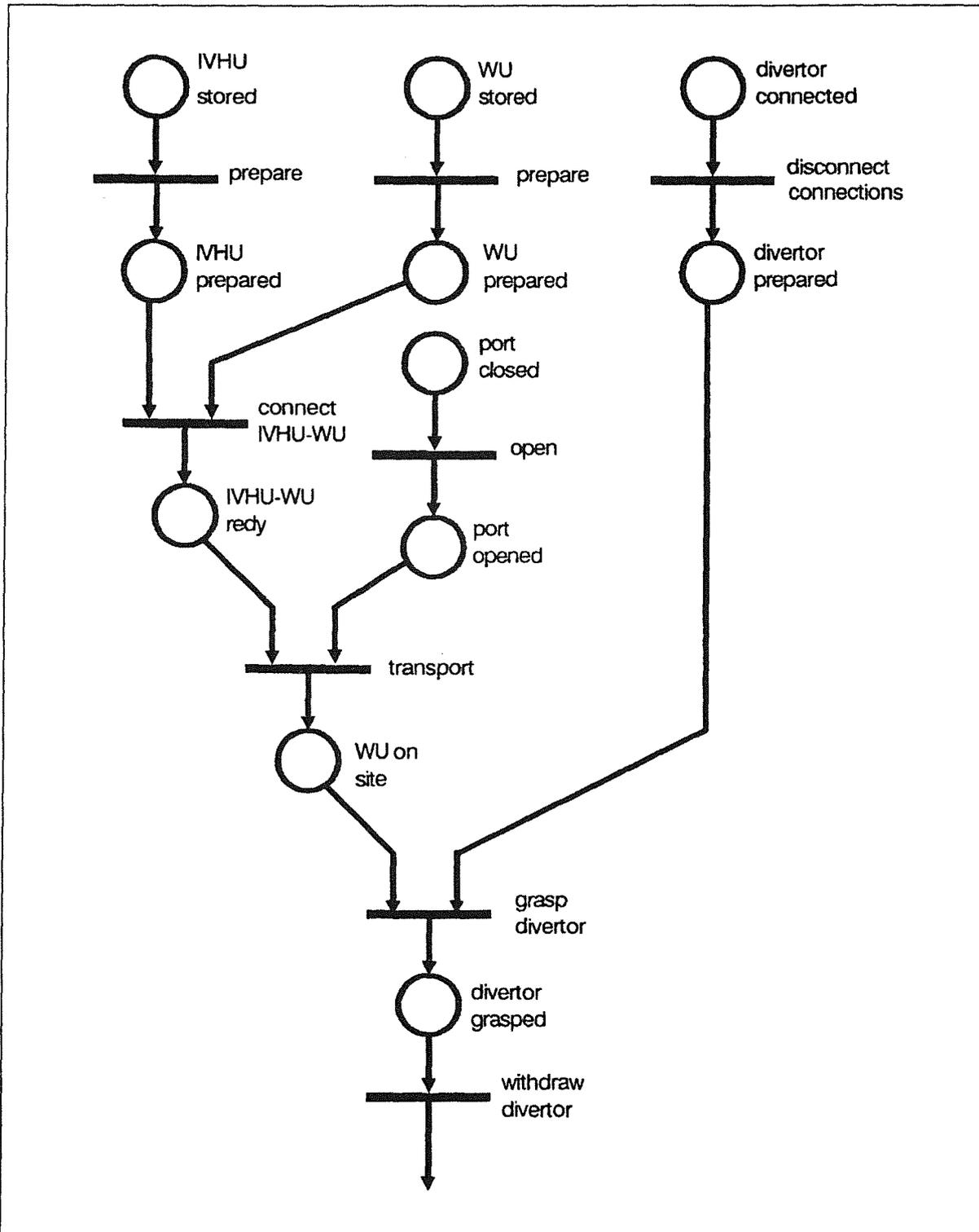
**Figure 28. Example of an action net.** These nets are used for high level planning and programming including especially the actions of the operator and the whole functionality of the control system. True state descriptions will be marked by a point in a circle ( by tokens). The token flow through the structure represents the progress of work.
