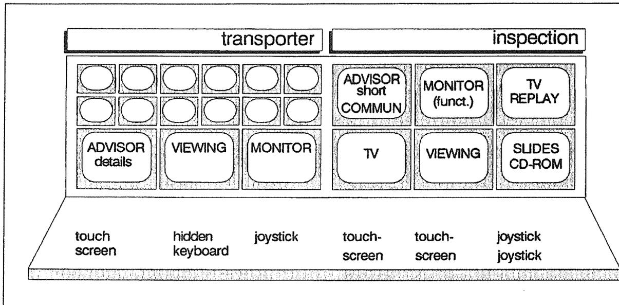
**Figure 39. NRWS-panel for inspection.** This is a two operator place (inspector and transporter driver) because both activities are needed more or less at the same time.
