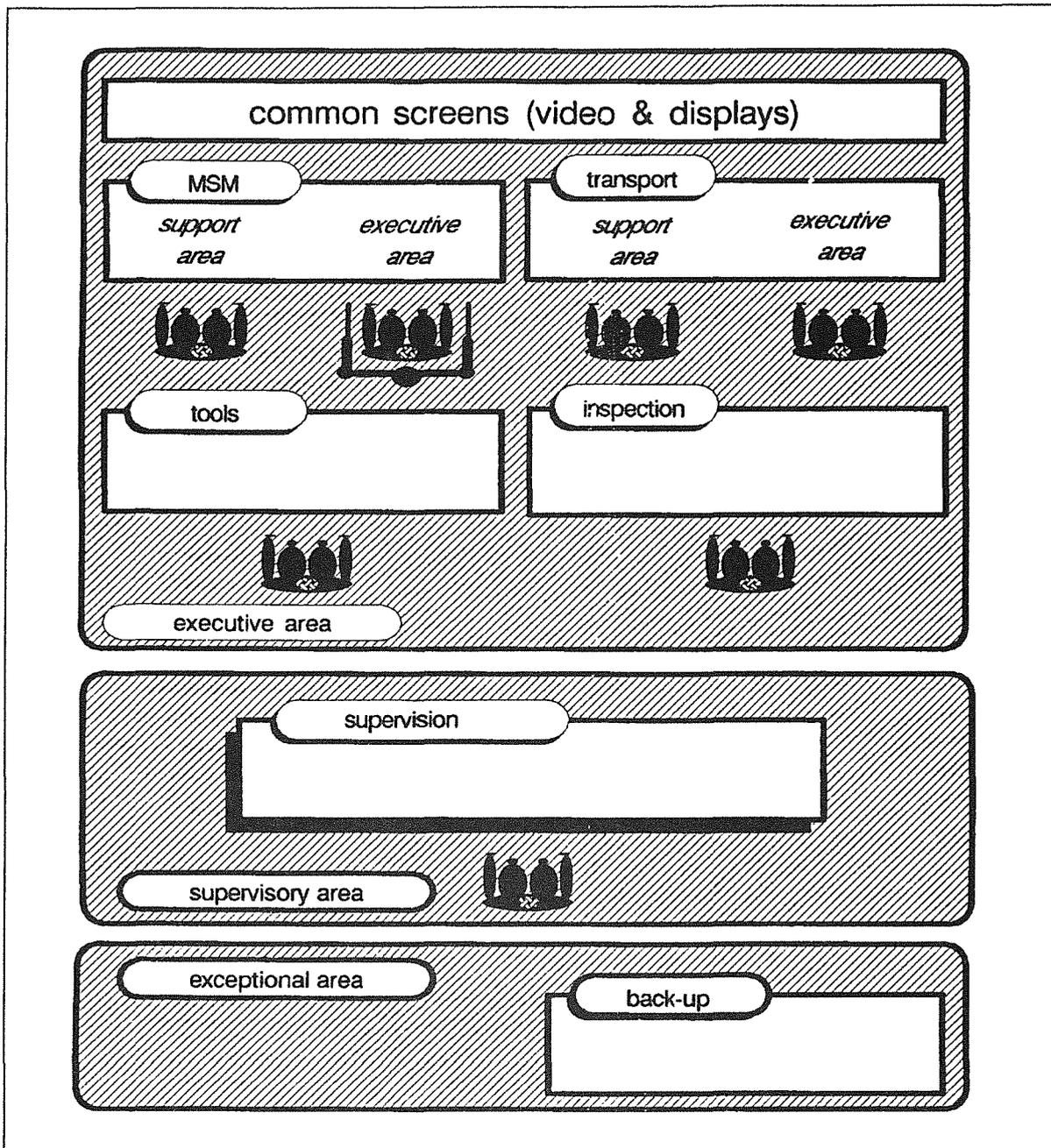
Figure 21. Remote handling control room layout (functional). This functional layout only shows the different components and working areas which have to be considered in a spatial layout. At least one workstation of each type has to be provided.
