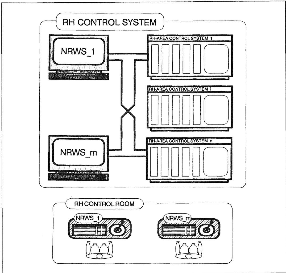
**Figure 15. General Purpose NRWS.** The links between the NRWSs and the control systems show the possible connections between two General Purpose NRWSs and two control systems.
