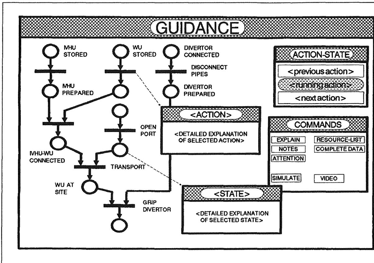
**Figure 42. Guidance window.** As basic information the window shows the procedure as an action net. Subwindows allow for displaying of detailed information about the procedure elements, the actual state of the task, and the actually available commands, dedicated to guidance.
