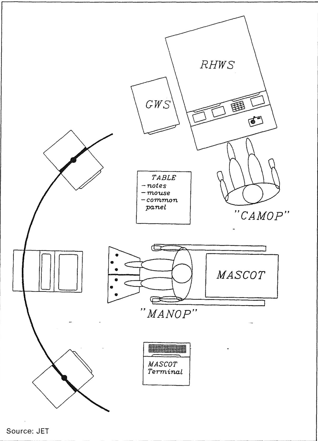
Figure 8. Servo Manipulator Master Station. Layout
