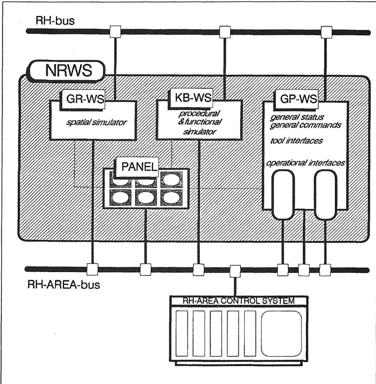
**Figure 33. NRWS hardware architecture.** Integration of workstations to the NRWS is done by using suitable software providing hardware independence (X-windows). GR-WS: Graphic Workstation, GP-WS: General Purpose Engineering Workstation, KB-WS: Knowledge-based Workstation, PANEL: Input devices and display screens integrated by X-window technique (Client). This integration of a panel is not state of the art.
