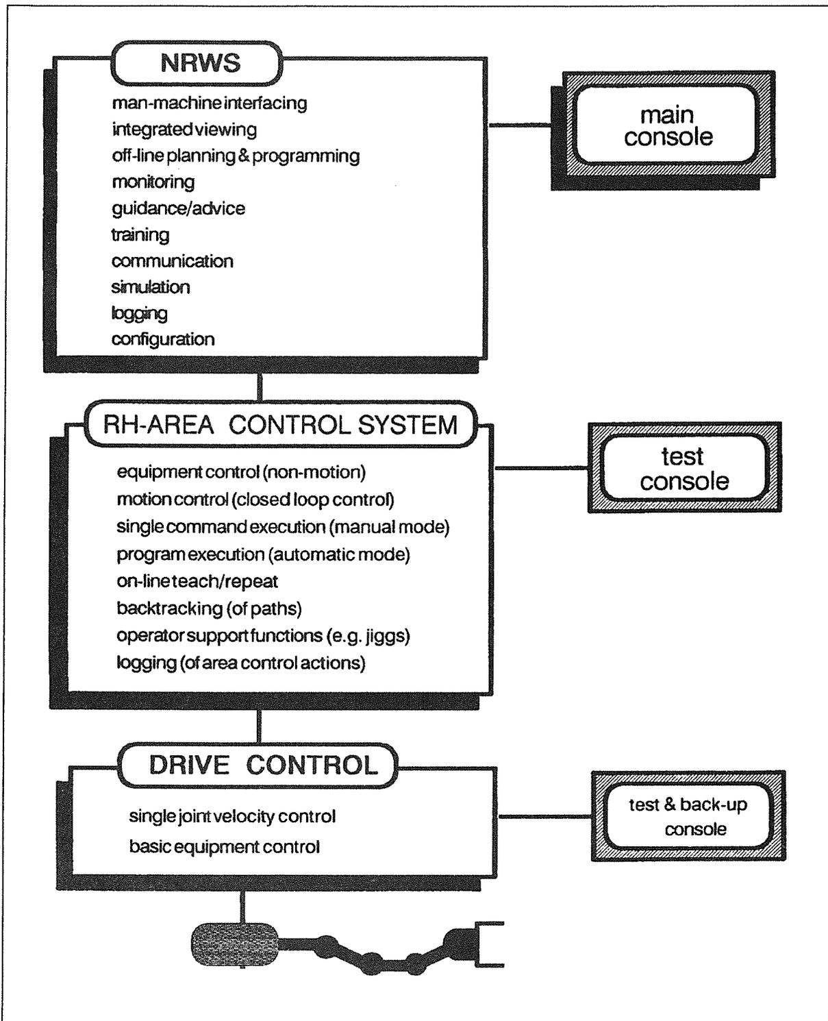
**Figure 23. Functionality of control system levels.** The NRWS represents the task level support and the man-machine interface, the RH-area control system represents the motion control level
