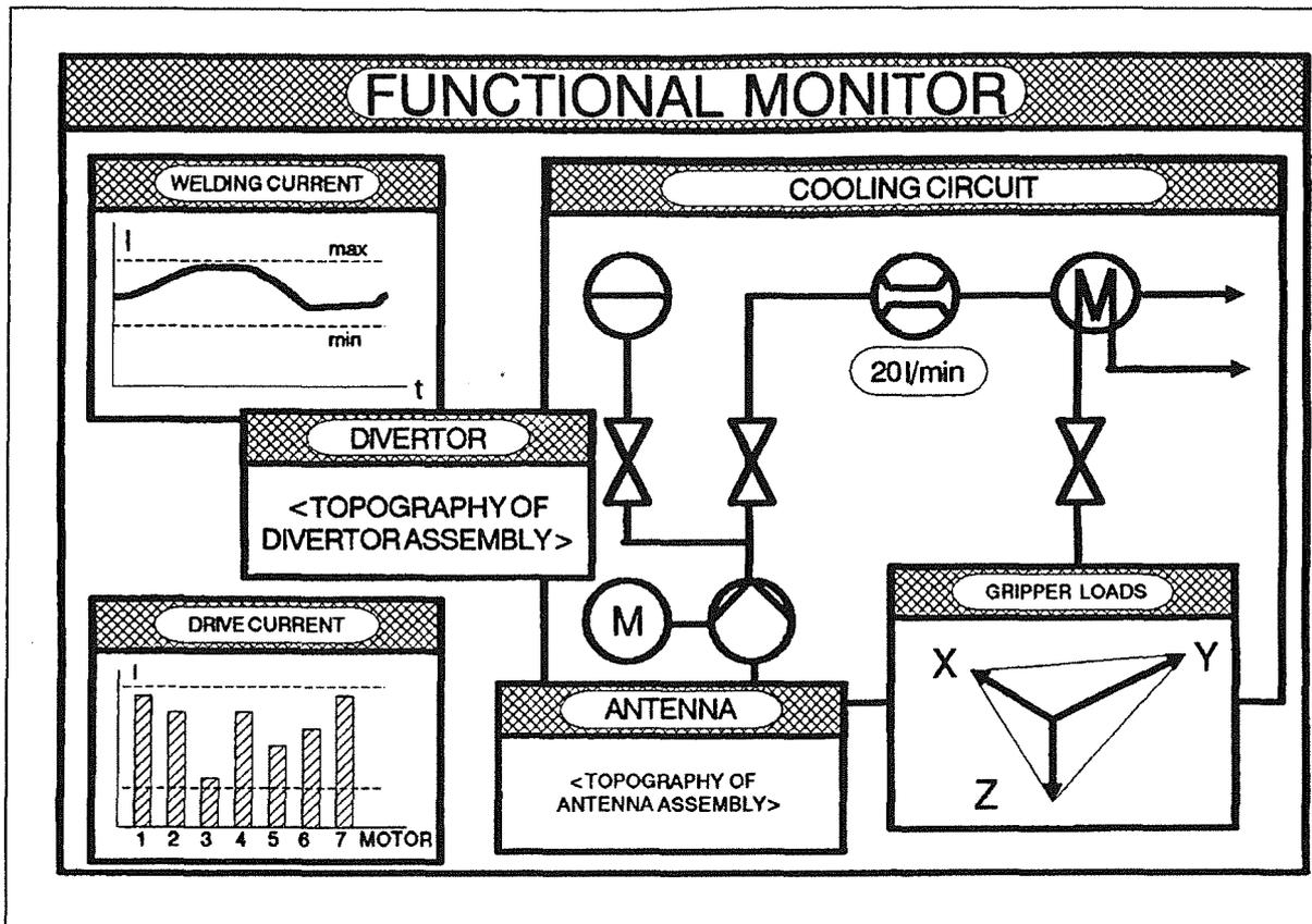
**Figure 44. Functional monitor window.** The examples shown support the operator in monitoring a welding machine, several motors, a cooling circuit, and gripper loads. Further sub-windows provide topographic information (mimics) about the divertor and/or antenna assembly state.
