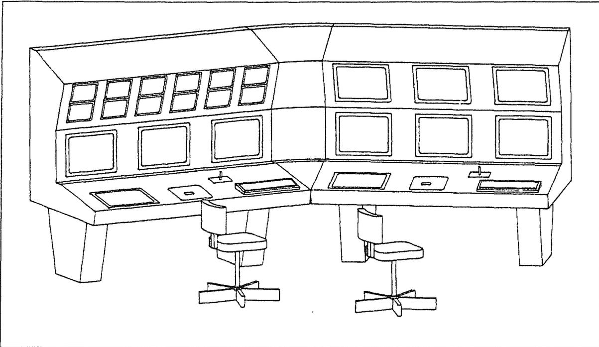
**Figure 35. Standard industrial control room panel.** The functional panel layout for the different types of panels is based on a standard industrially available panel. An ergonomic layout is still needed.
