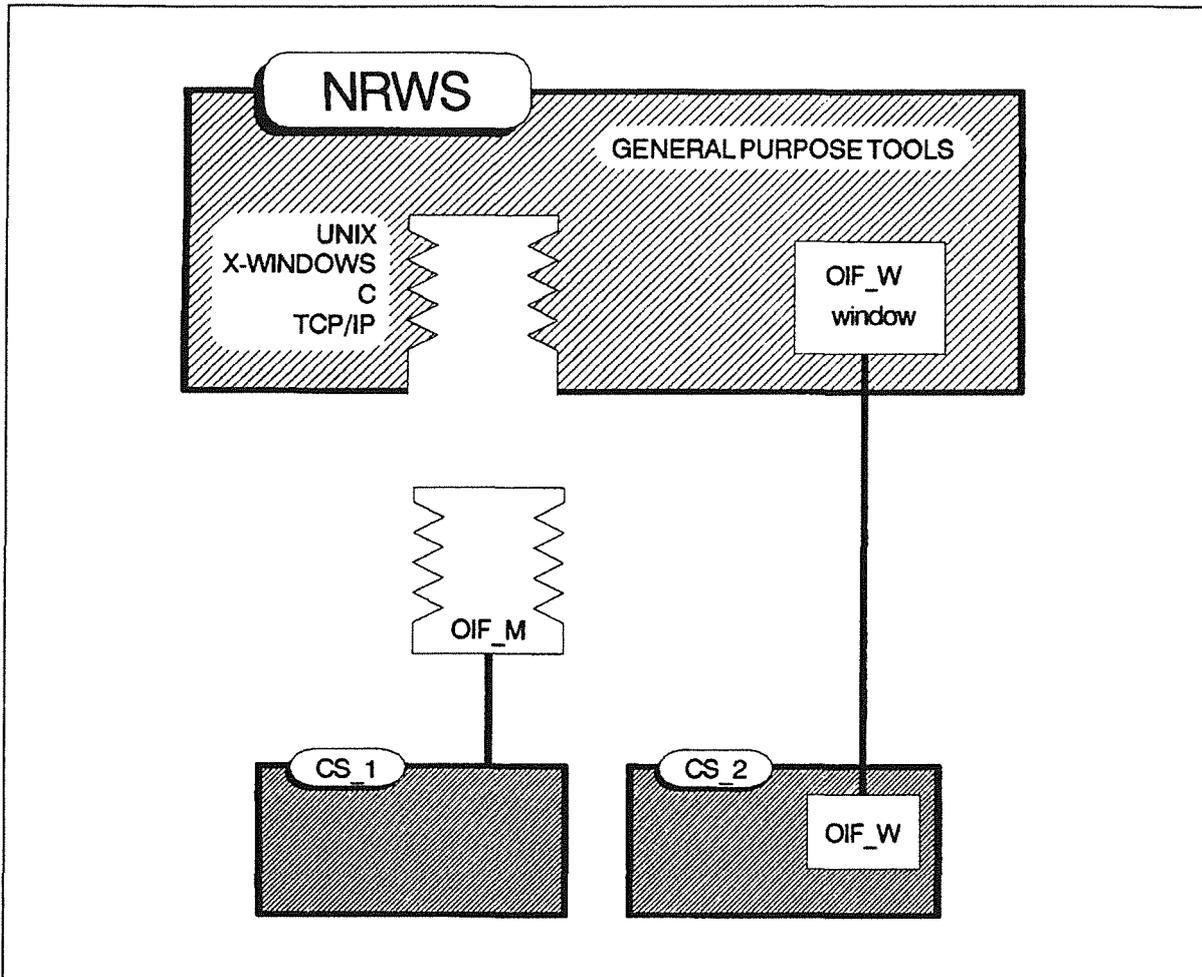
**Figure 46. NRWS and RH-area control system operating interface.** For operating the RH-area control system has to provide an interface module. Two types are possible for integration into the NRWS: (1) a module (OIF\_M) runnable on the NRWS or a general purpose workstation providing the same internal interfaces, or (2) a module (OIF\_W) running on the RH-area control system, accessible via an X-server by opening a X-window (OIF\_W window). CS\_1 may for example be the IVHU area control system.
