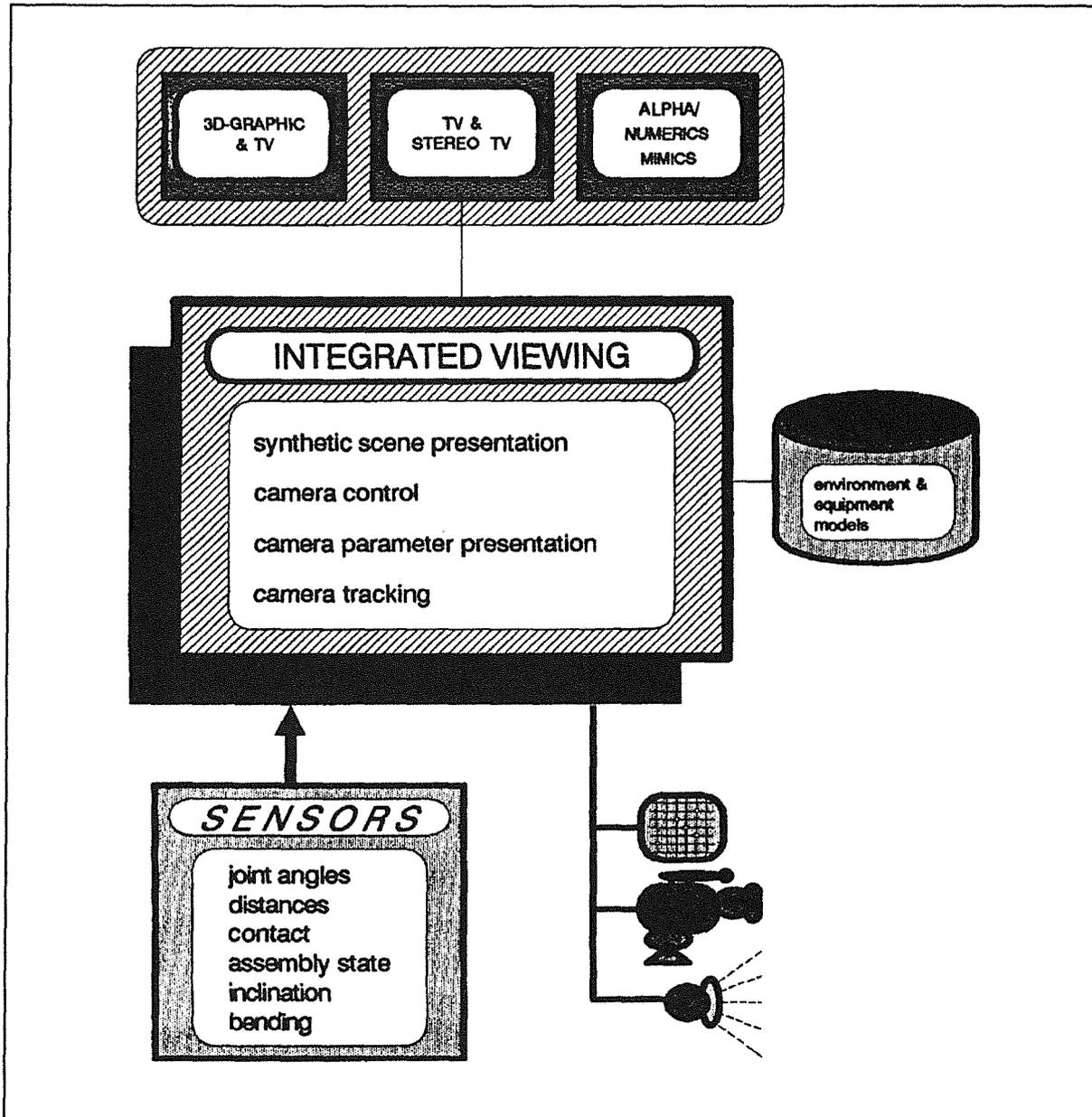
**Figure 25. Concept of integrated viewing.** The integration of artificial viewing using sensor controlled computer graphics with standard TV unifies and simplifies the work of the camera operator. The goal is to provide one tool for one function.
