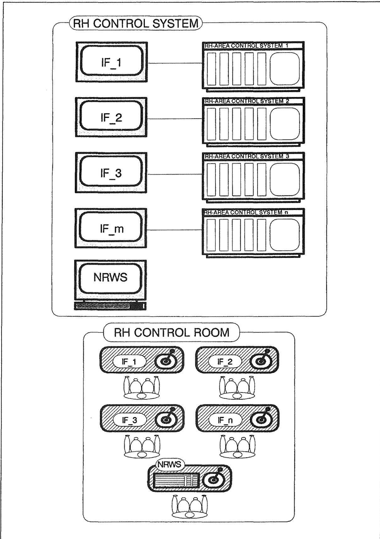
Figure 17. Off-line NRWS. The control system are only directly equipped with a relatively simple operating interface. High level support tools are implemented in the off-line NRWS.
