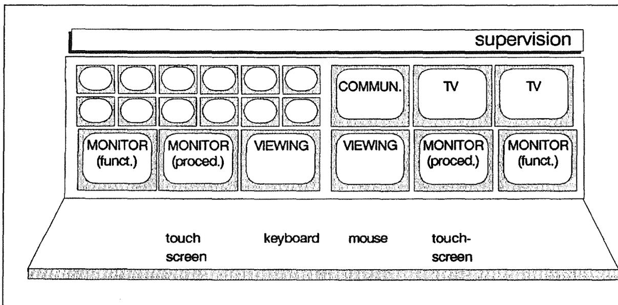
Figure 40. NRWS-panel for supervision. Supervision is mainly VIEWING (overview) and MONITORING
