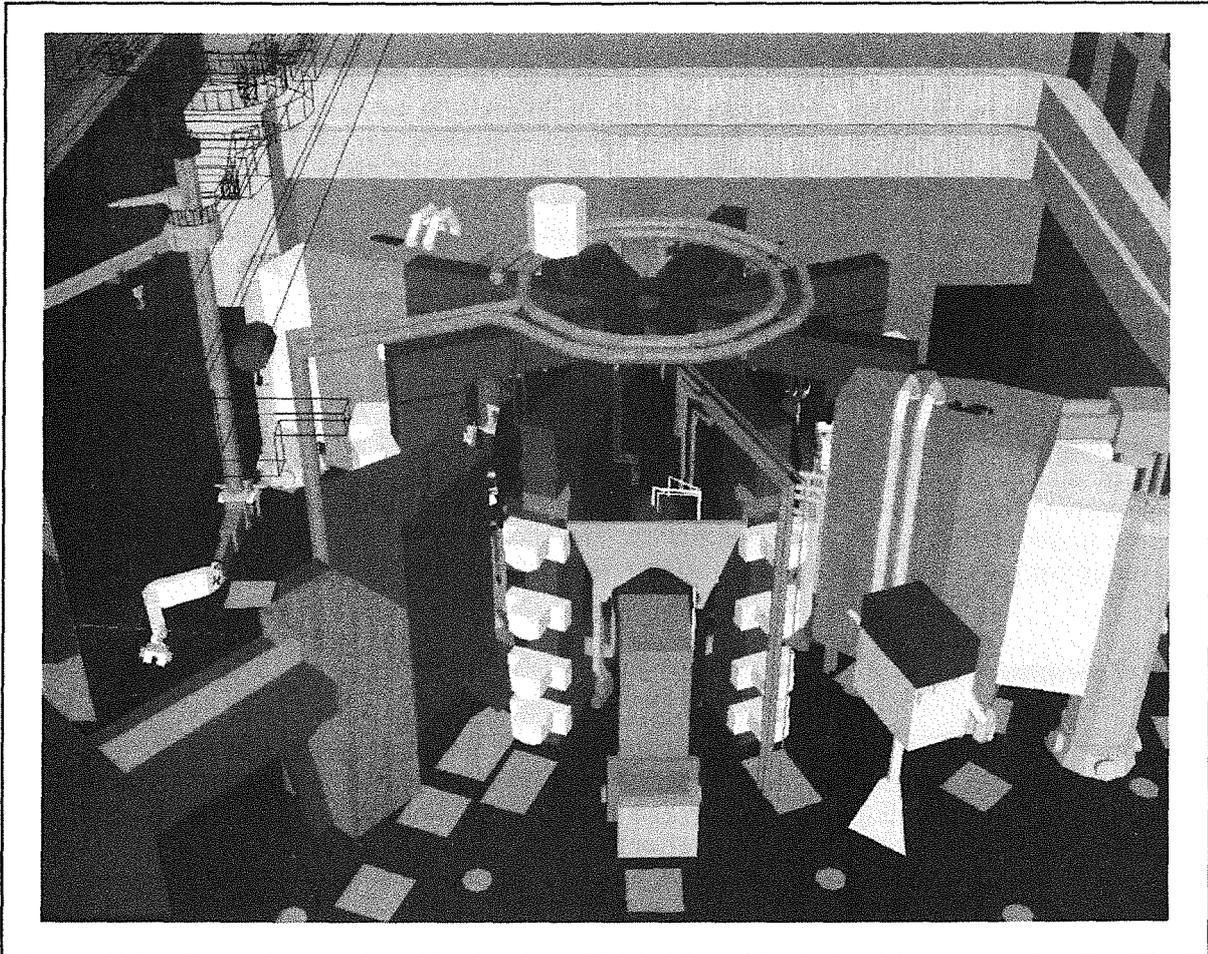
**Figure 27. KISMET display example for JET-TARM control.** The display shows a birds eye view of the JET torus (ex-vessel view) and the TARM (left hand side)
