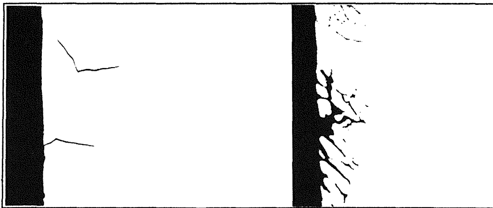
a) Base material 200 X b) Weldment 500 X Figure 3: Selective corrosion in 1.4948 after 1003 hrs exposure at 350 °C in experiment B, magnification: 200 X
