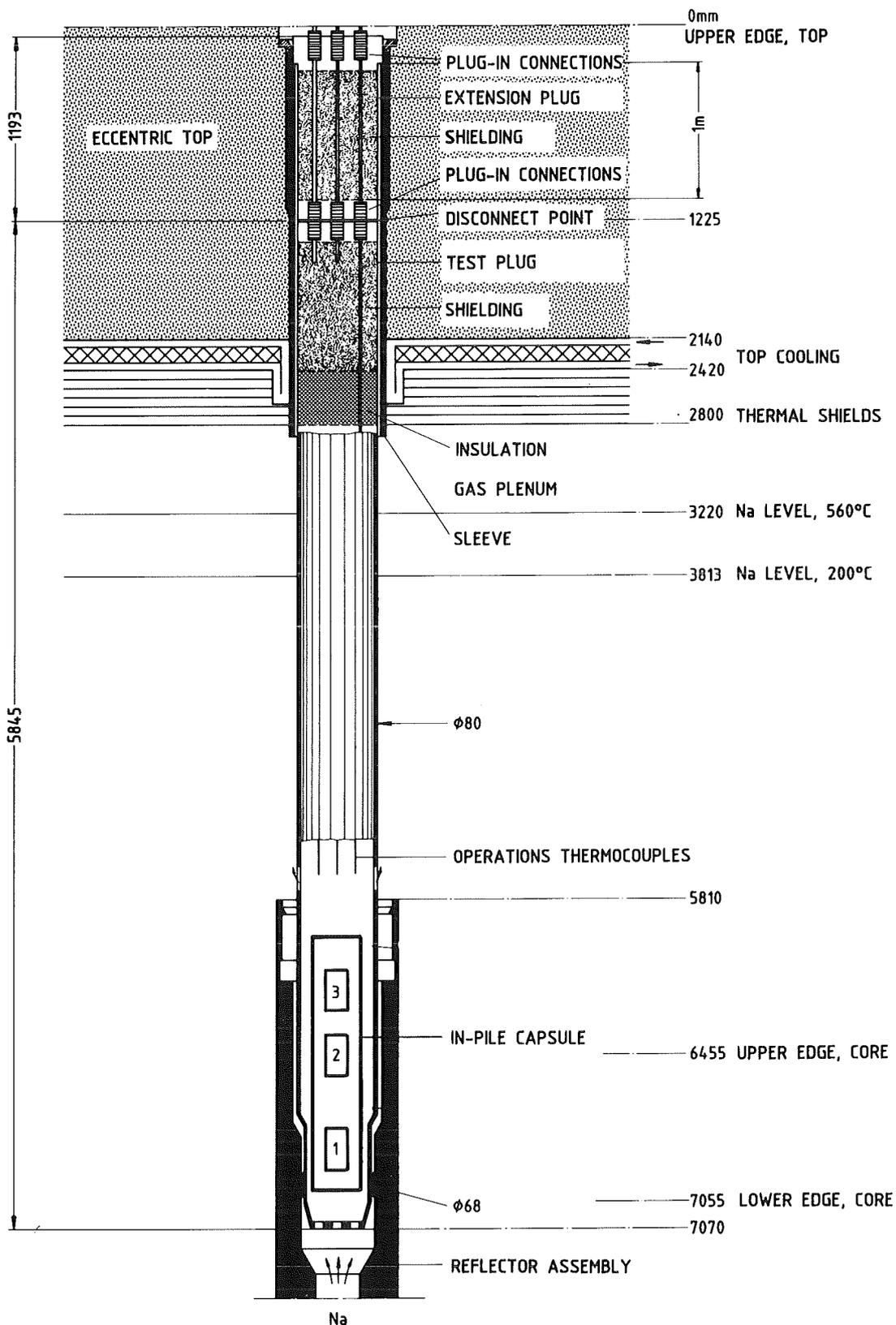
**Fig. 15 : Test plug in the irradiation position**
