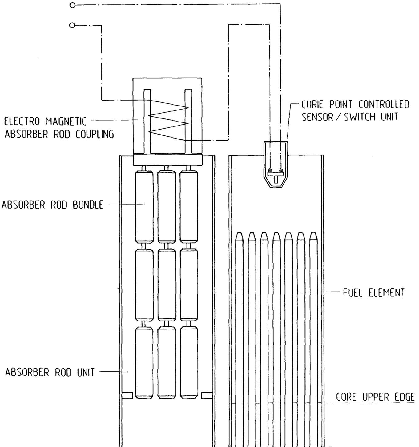
**Fig. 1 : Temperature-sensitive, inherent reactor shutdown system**
