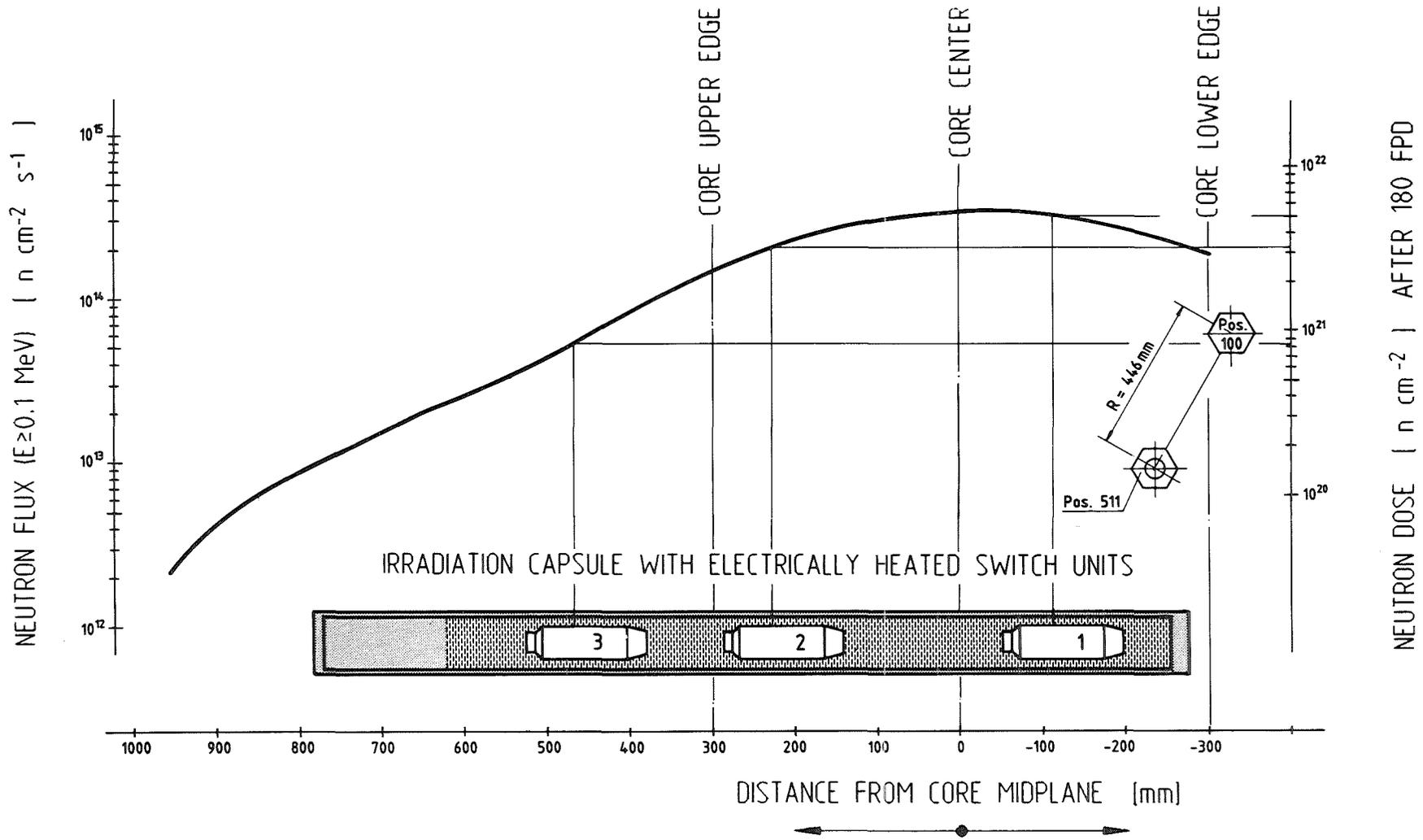
**Fig. 13 : Development of axial neutron flux ( $E \geq 0.1$  MeV) at reflector position 511**
