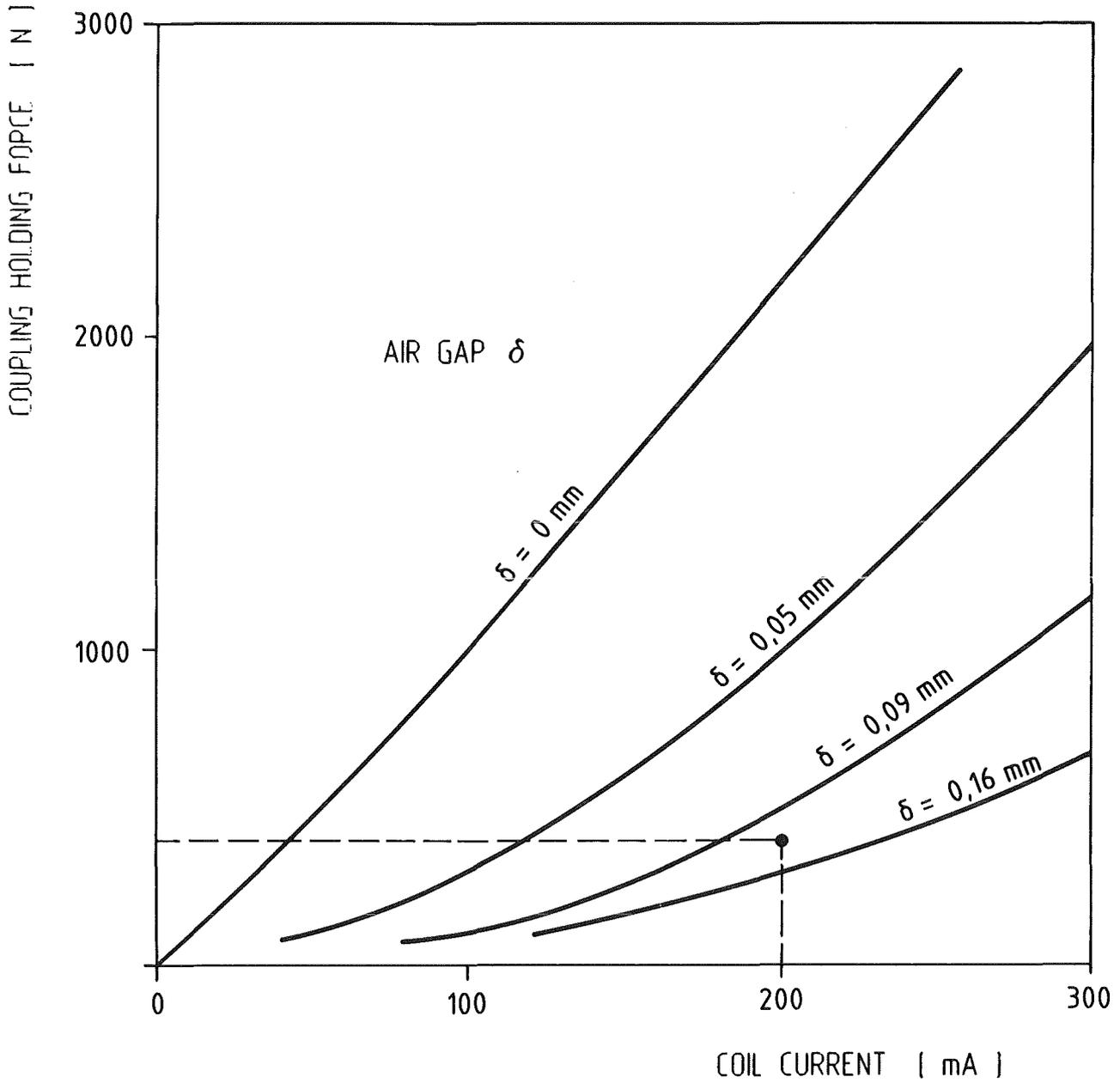
**Fig. 8 : Holding force of the coupling as a function of the coil current**
