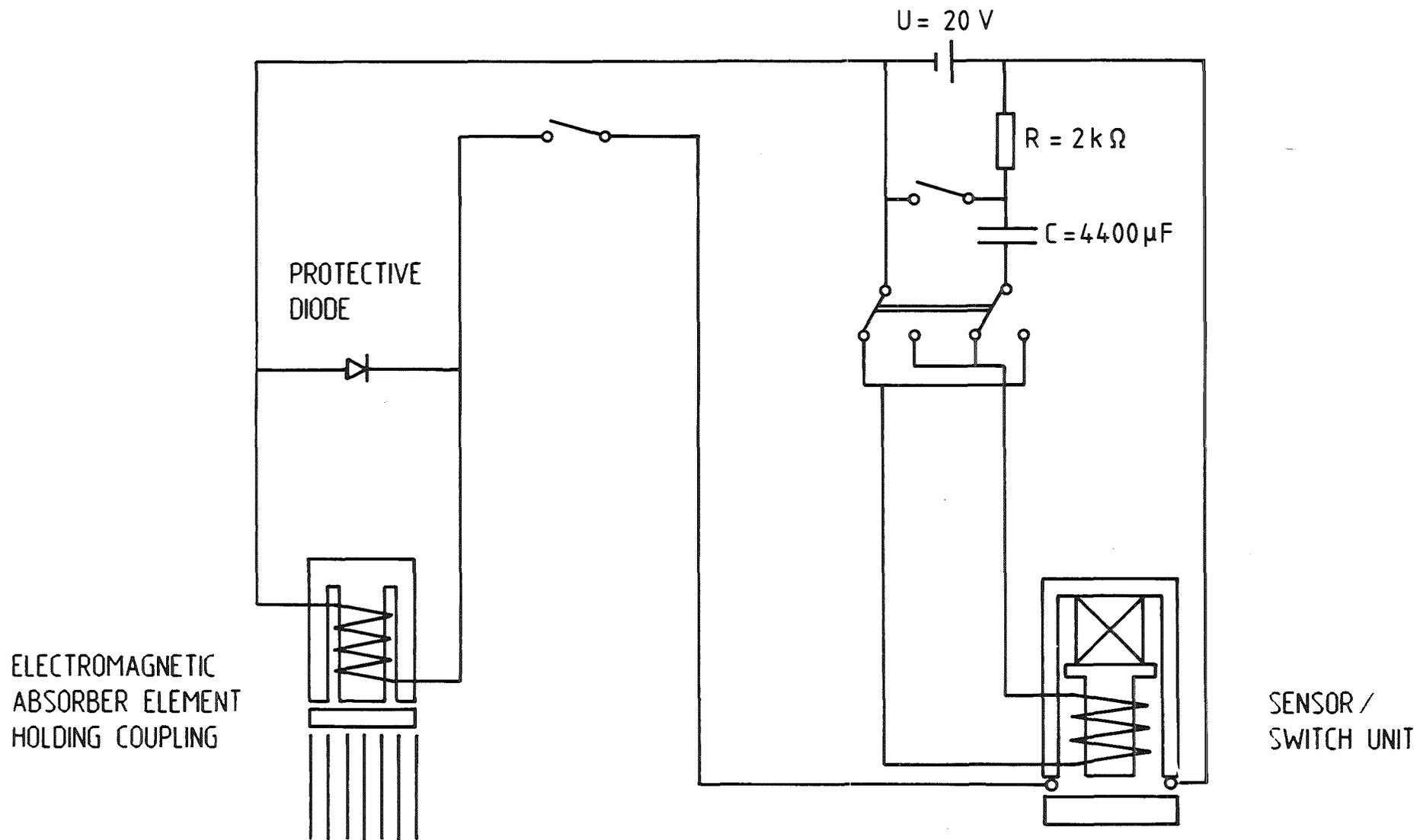
**Fig. 3 : Electric circuit of the shutdown system**
