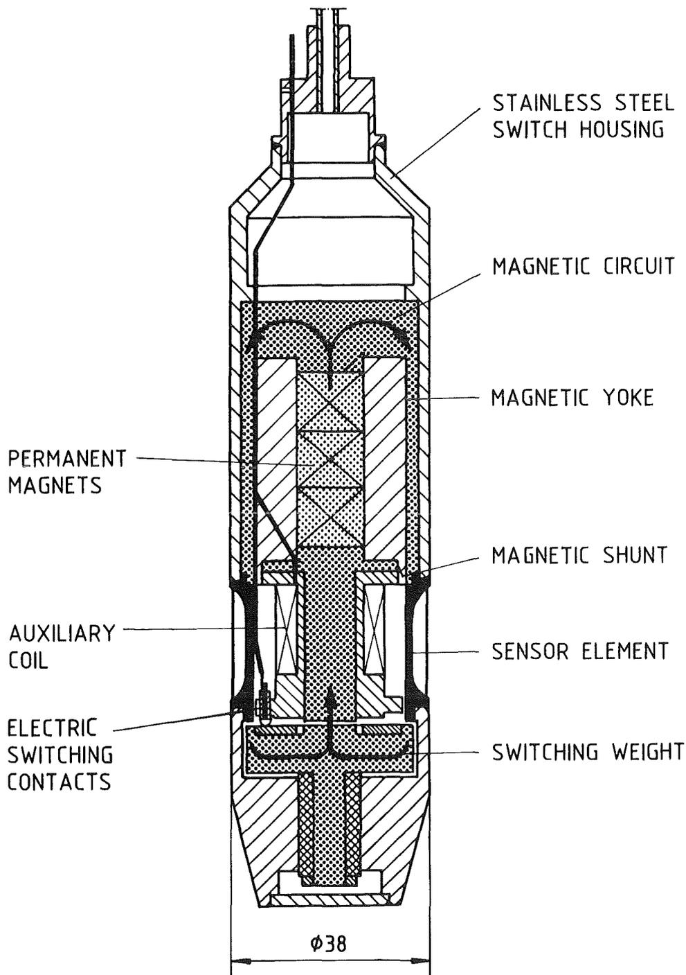
**Fig. 2 : Curie point controlled sensor/switch unit**
