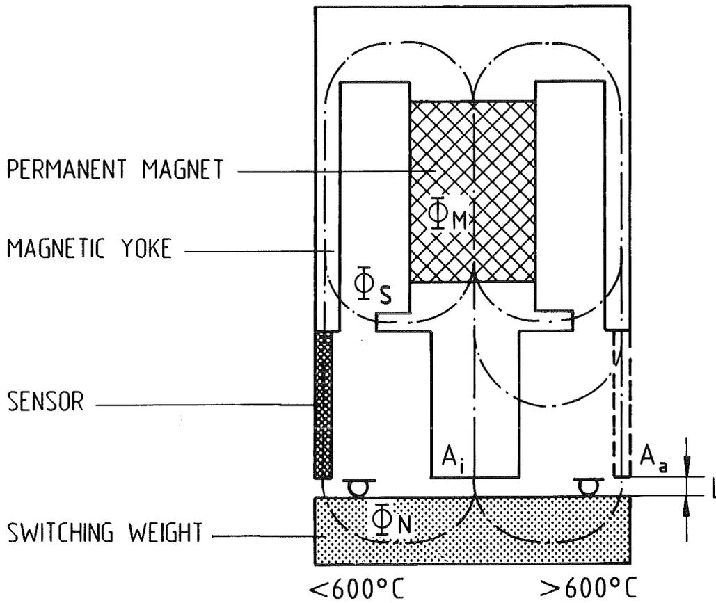
**Fig. 5 : Schematic representation of the magnetic circuit**
