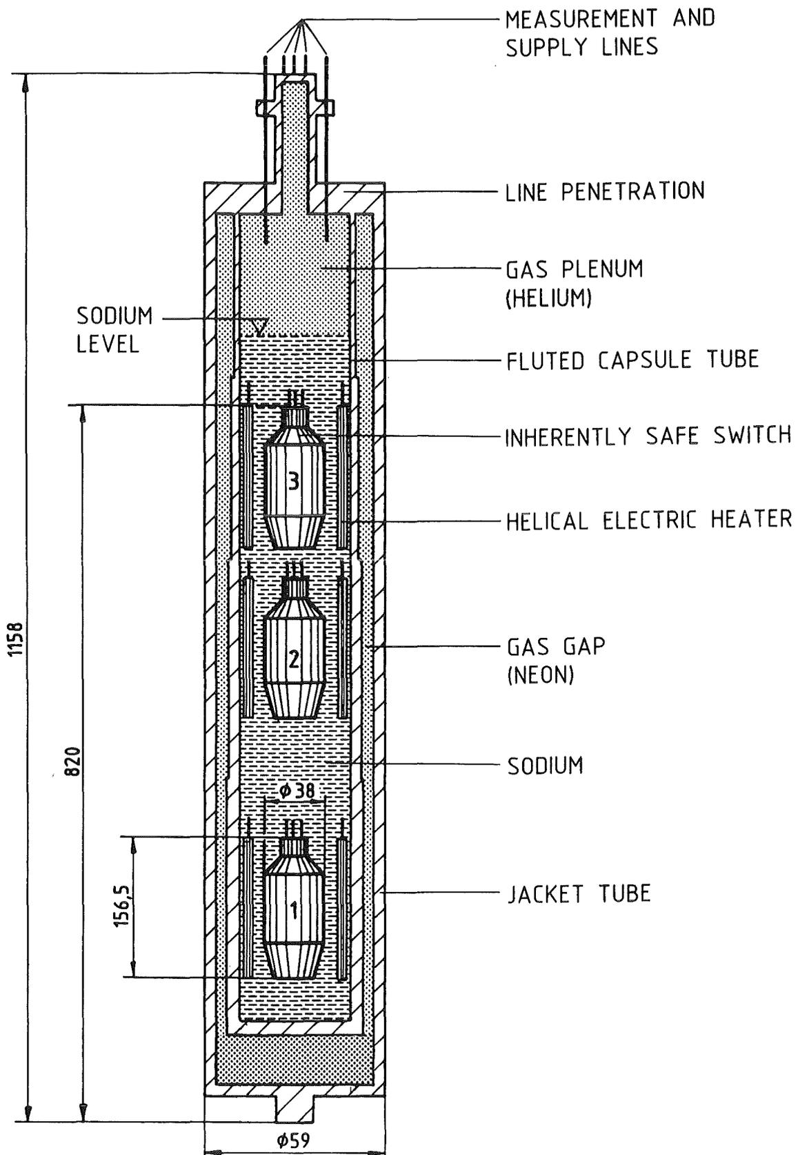
**Fig. 14 : Electrically heated capsule with three switch units**
