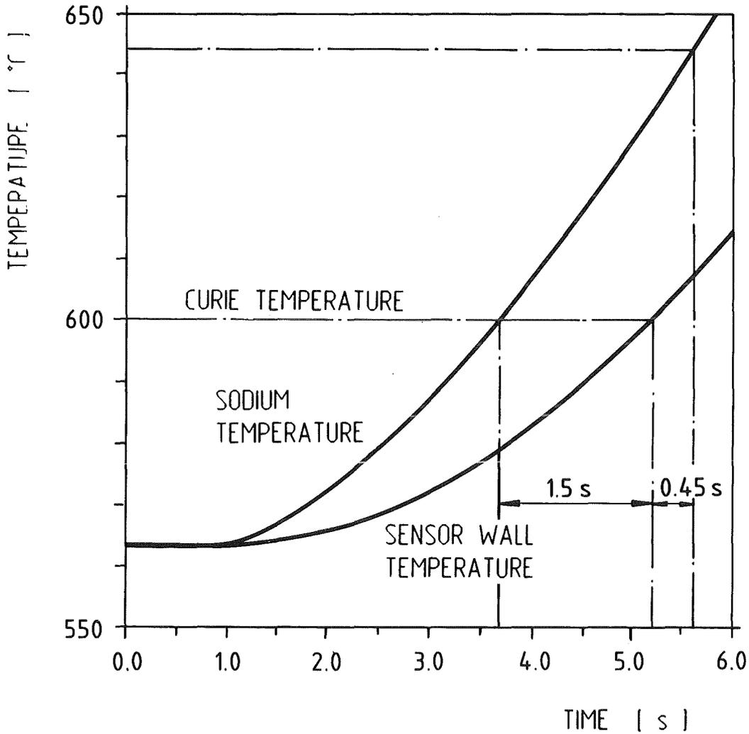
**Fig. 11 : Sensor wall temperature in an SNR LOF-accident**
