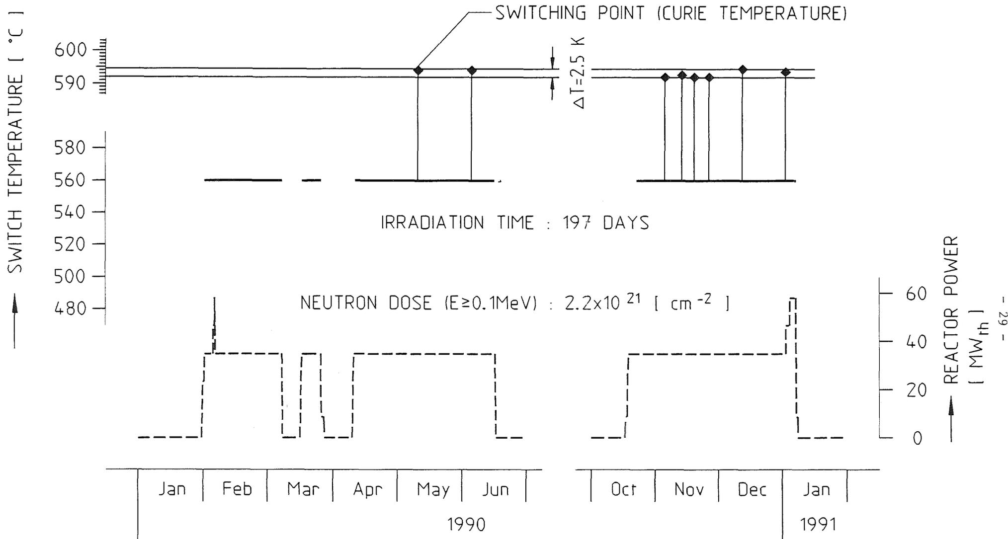
**Fig. 16 : Irradiation diagram for test switch No. 2 (center)**
