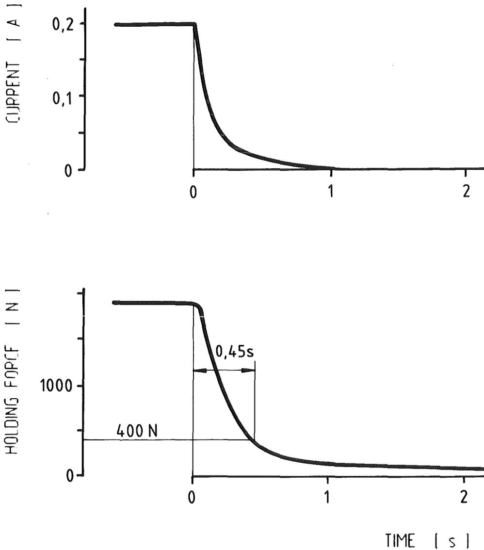
**Fig. 9 : Current and holding force of the coupling after shut down**
