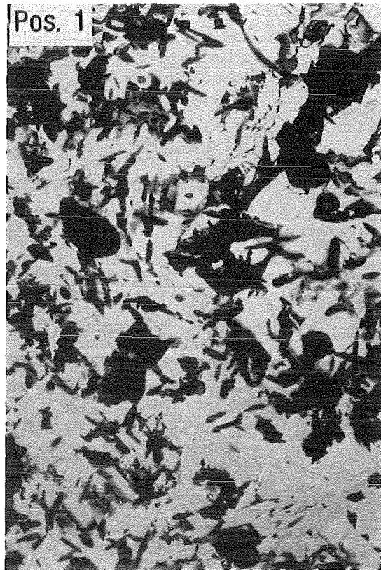
Central melt region with free carbon
