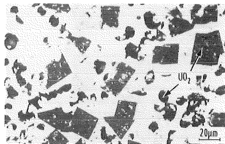
metallic melt with ceramic precipitations
