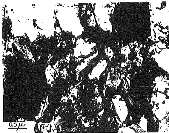
Fig. 5: Equiaxed subgrain structure formed after N_f = 2952 cycles with a temperature change of 473 - 873 K and HTHL condition.
