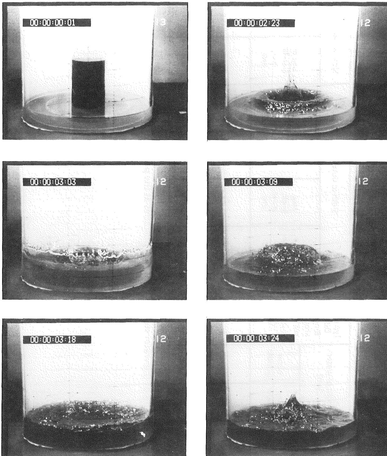
Figure V.3.3: Water step problem SC-D1HX-1 with a 2 cm obstacle at the pool bottom
