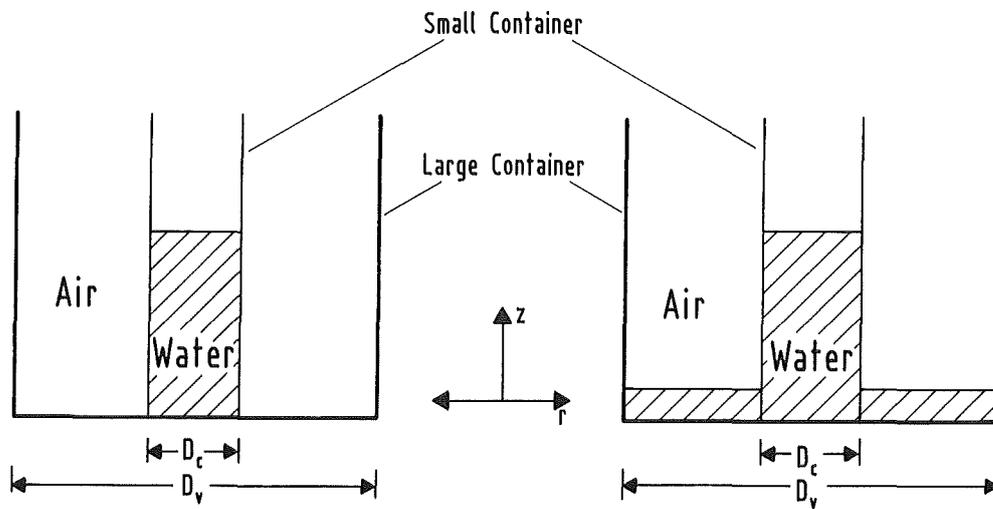
Figure 1.2: Schematic dam break and water step experimental set up in the  $r$ - $z$  plane
