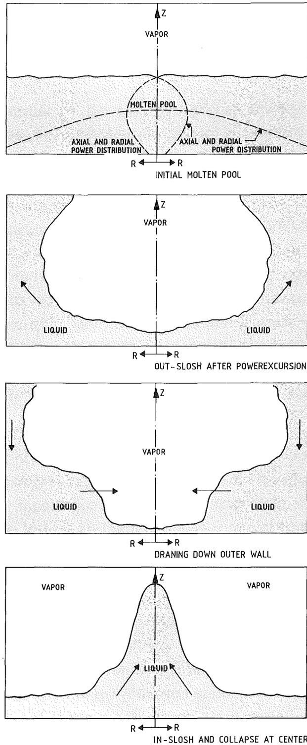
Figure I.1: Schematic representation of liquid fuel sloshing in an ideal cylindrical pool
