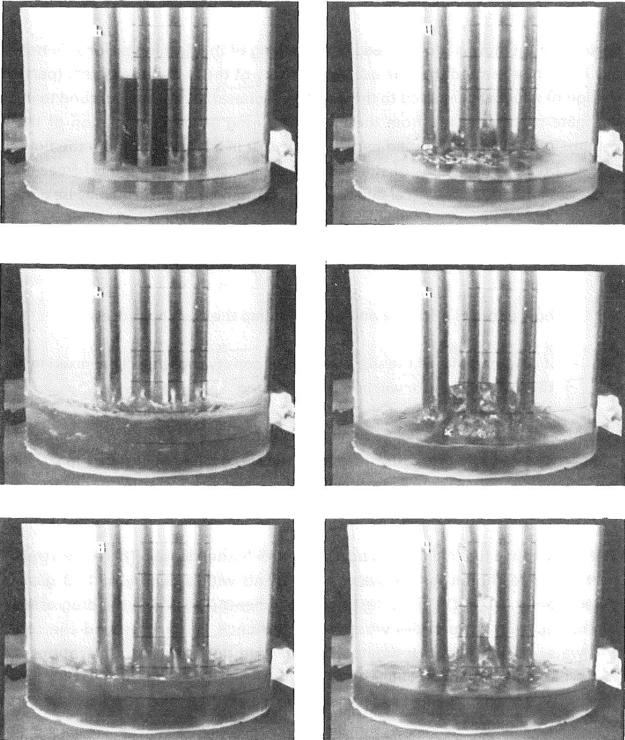
Figure V.4.5: Water step problem SD-D1RX-1 with a central full bank of rods in the flow
