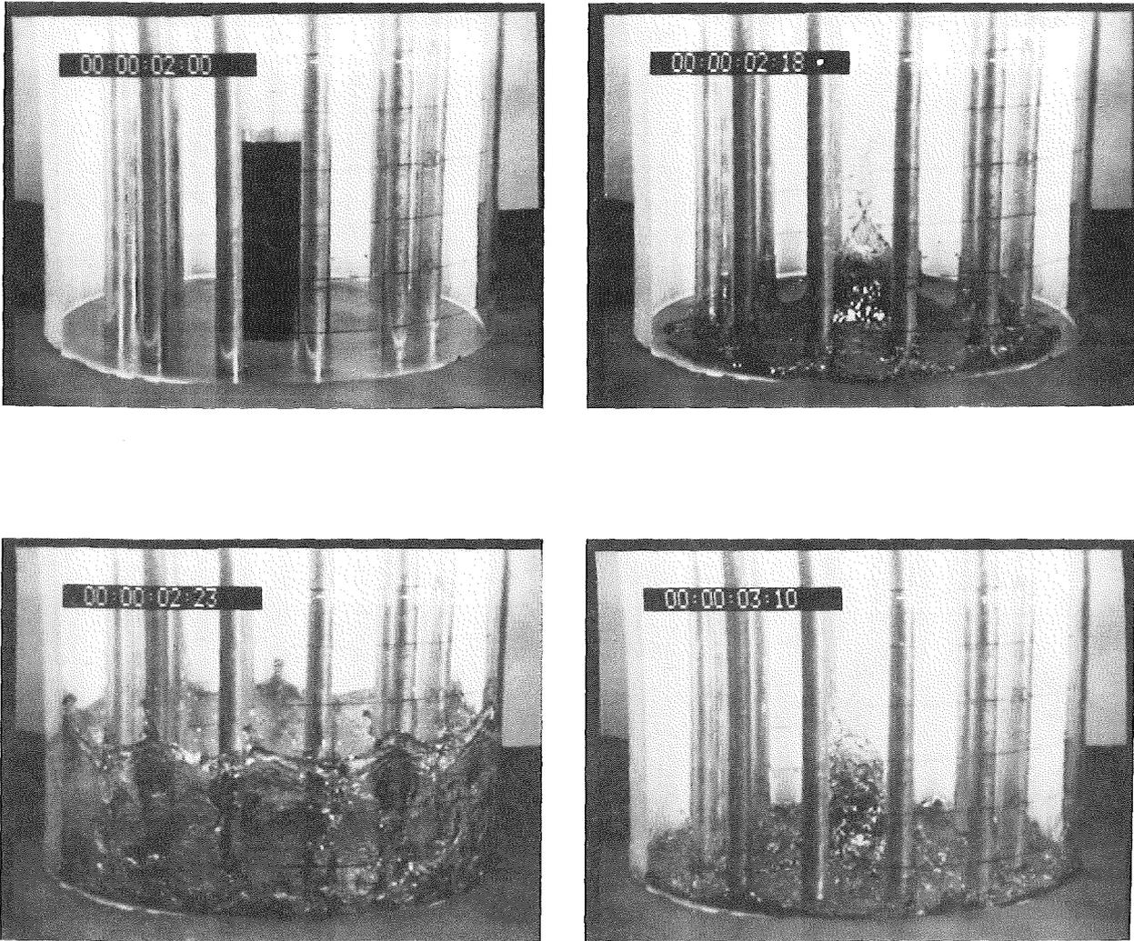
Figure V.4.2: Dam break problem SD-D1R-2 with a peripheral full bank of rods in the flow
