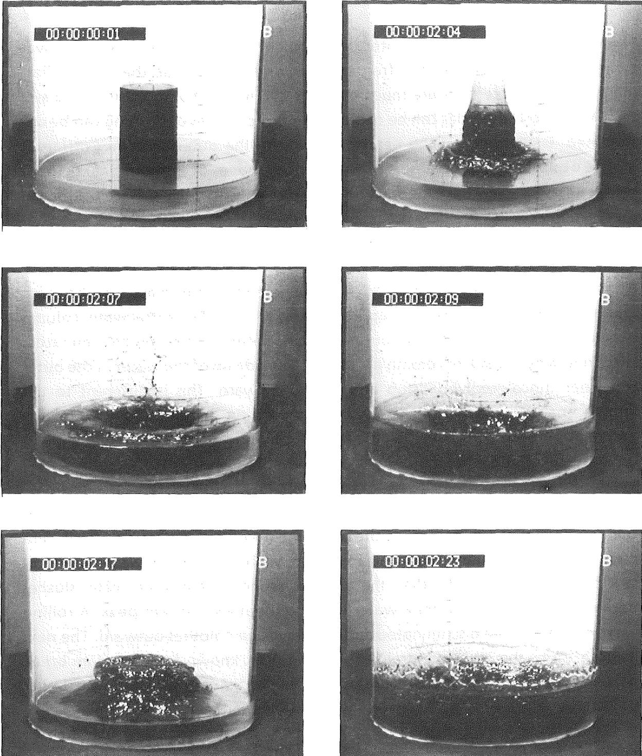
Figure II.2: Sloshing motions seen in a typical water step problem
