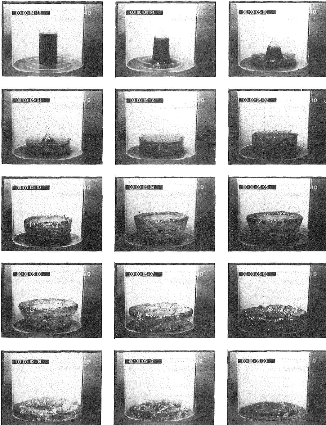
Figure V.3.2 Dam break problem SC-D1H-2 with a 3 cm obstacle at the pool bottom
