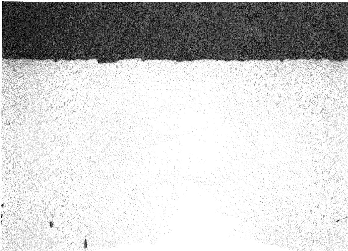
Fig. 13b: Surface roughening of the 1.4914 sample KfK 02-14 in contact with beryllium, magnif. 500 x
