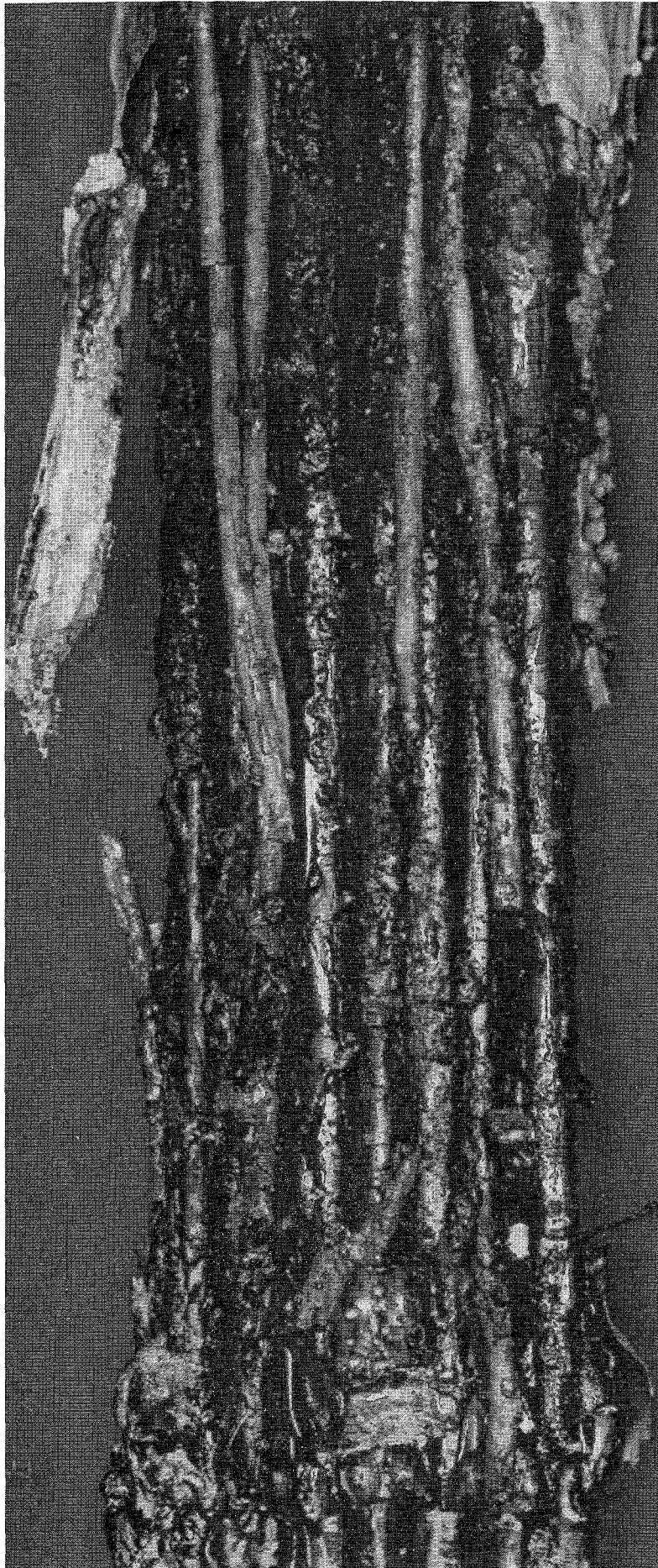
Fig. 99: Posttest view of bundle CORA-13
