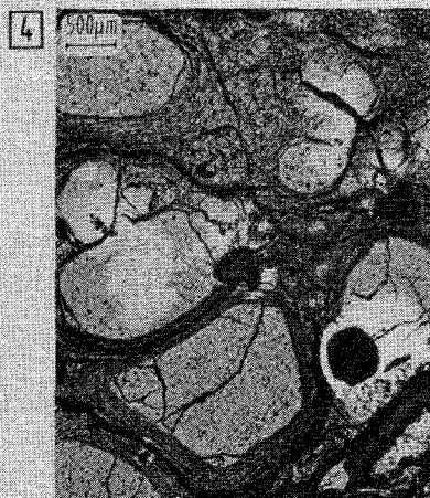
crack pattern in ceramic material
