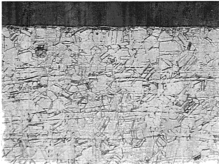
Fig. 14: Optical micrograph of the steel tube plating material Hastelloy C4 after 6.3 years in-situ testing in rock salt plus NaCl-brine at 32°C (x 200)
