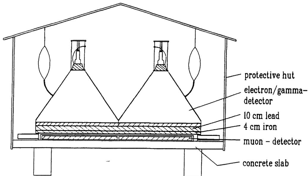
Fig.2. Schematic view of a station of the KASCADE array
