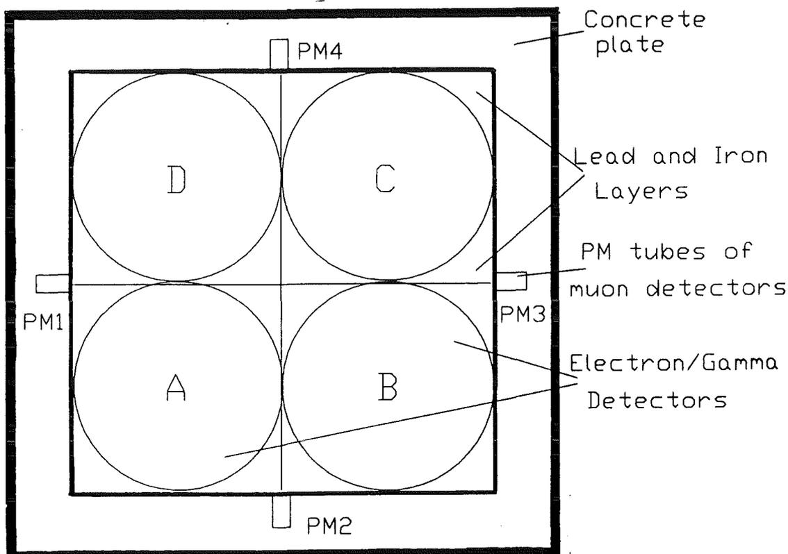
Fig.5. Top view of the detectors in one station
