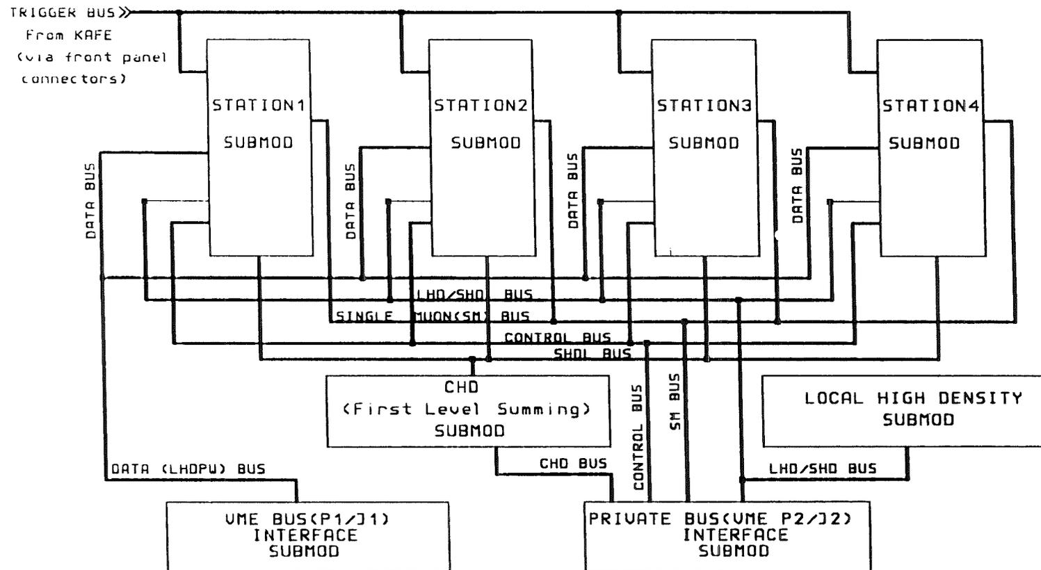
Fig.9. Quadrant Module 1 block diagram
