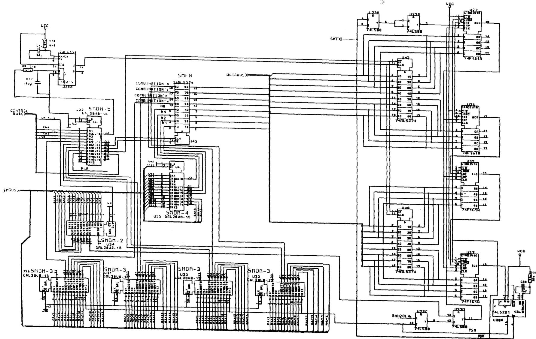
Fig. 12. Single Muon Detection Module
