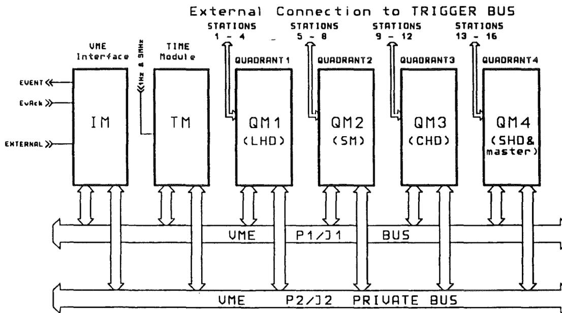
Fig.6. Physical structure of the Trigger Unit
