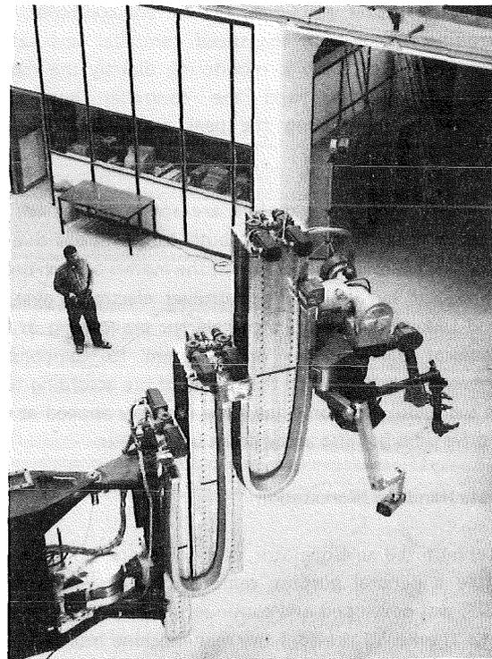
Fig. 3: Interim manipulator handling unit with viewing system
