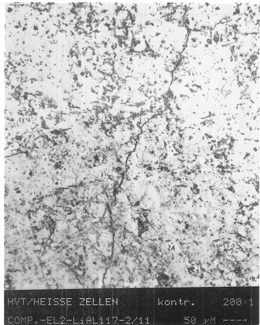
Fig. 5: Microstructure of \text{LiAlO}_2 (ENEA) irradiated in the HFR reactor at 440 °C to 0.28% Li-burnup
