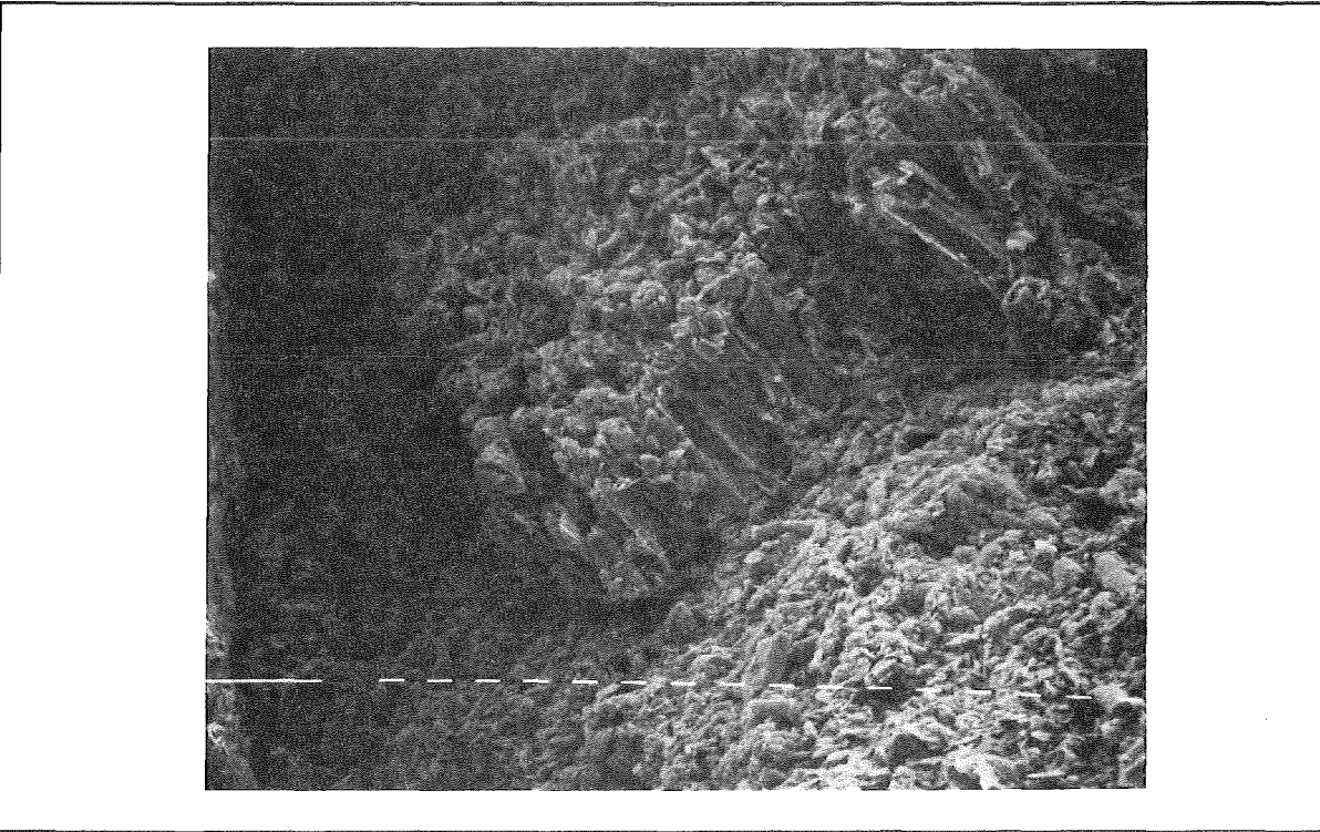
Figure 31. . Fracture surface of material FMI 3333 at a magnification x320.
