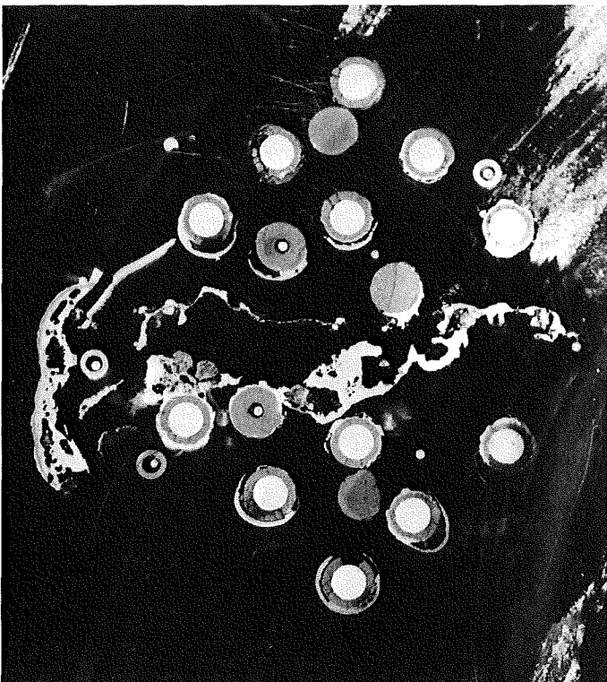
Fig. B2: Horizontal cross sections of bundle CORA-33; 1045, 1043, 993, 991 mm
