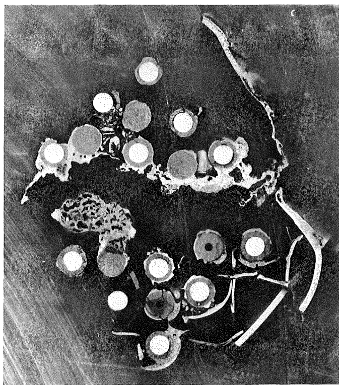
Fig. B7: Horizontal cross sections of bundle CORA-33; 599, 597, 547, 545 mm
