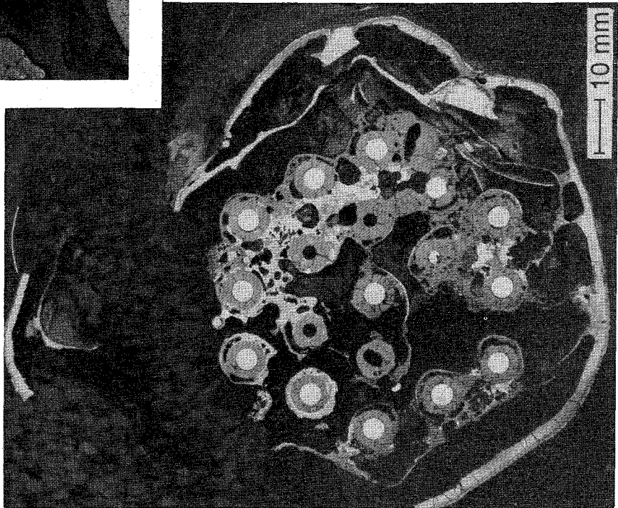
Fig. 22: Cross Section CORA-W2-k (top), Elevation 605 mm Overview
