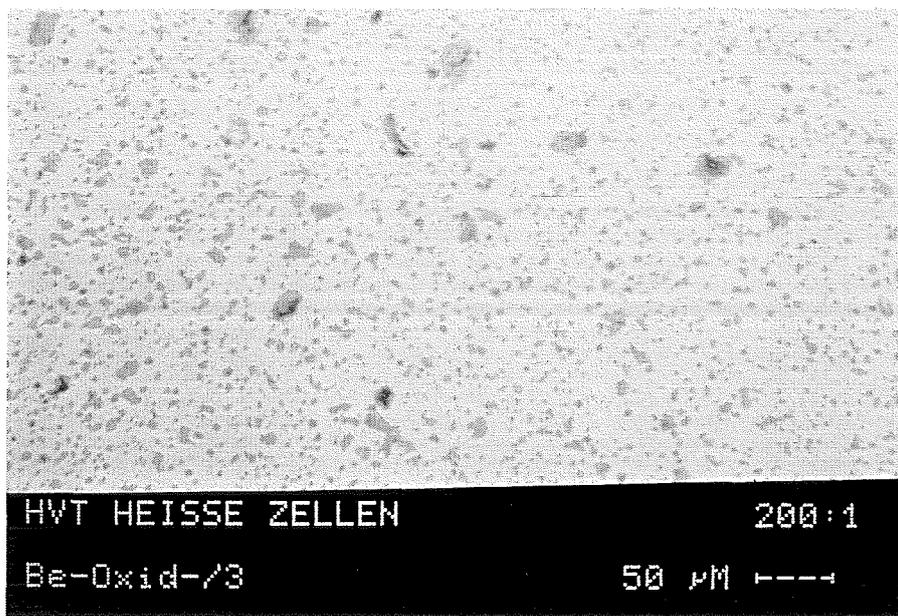
Fig. 5: Micrograph of "BeO", non etched
