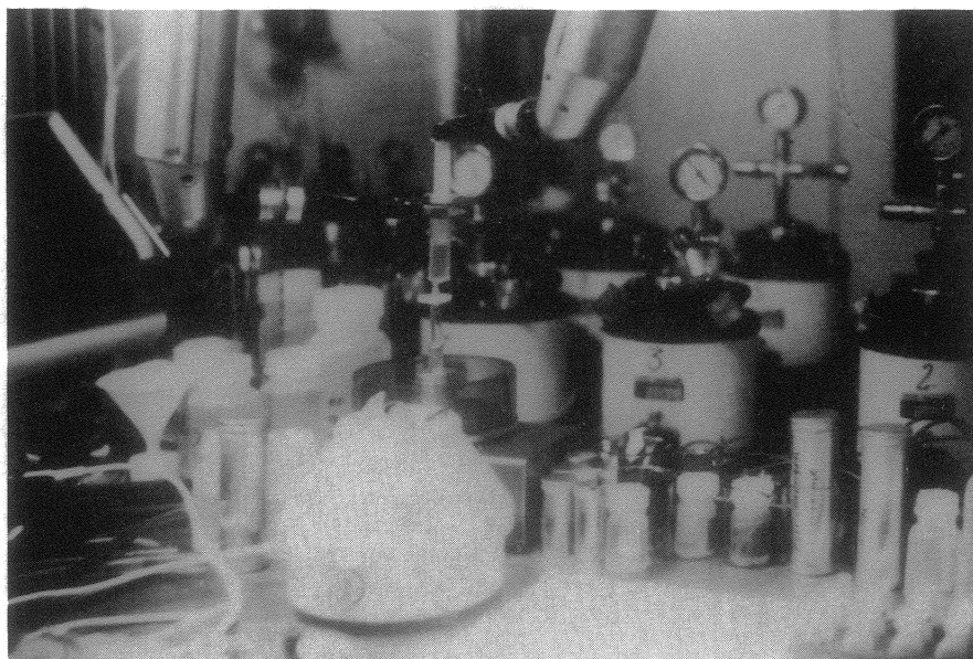
Figure I.9: Sampling methods of leach solutions: Top: Flushing of an autoclave with water saturated Ar during solution sampling. Solution samples are taken by means of a syringe; Bottom: inserting a solution samples filtered by a 0,45 \mu\text{m} micro filter into a vial with an 1,8 nm ultra filtration membrane, prior to centrifugation.
