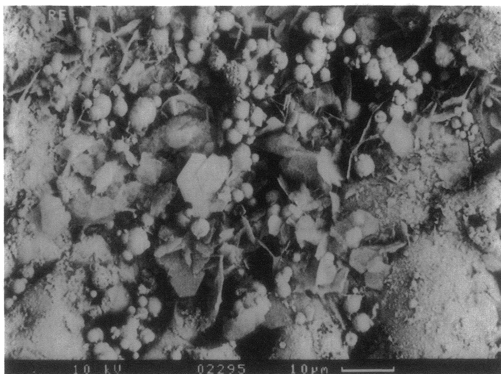
Figure II.10: SEM micrographs of the Ti/Pd plates from experiment K3 after two years of corrosion at room temperature in 95% saturated NaCl solution in presence of Fe
