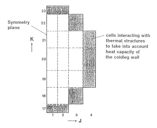
Figure 3. Input Sample Detail. Section across the Cold Leg.
