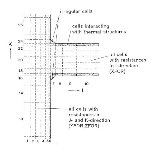
Figure 2. Input Sample Detail. Junction of Cold Leg and Downcomer.
