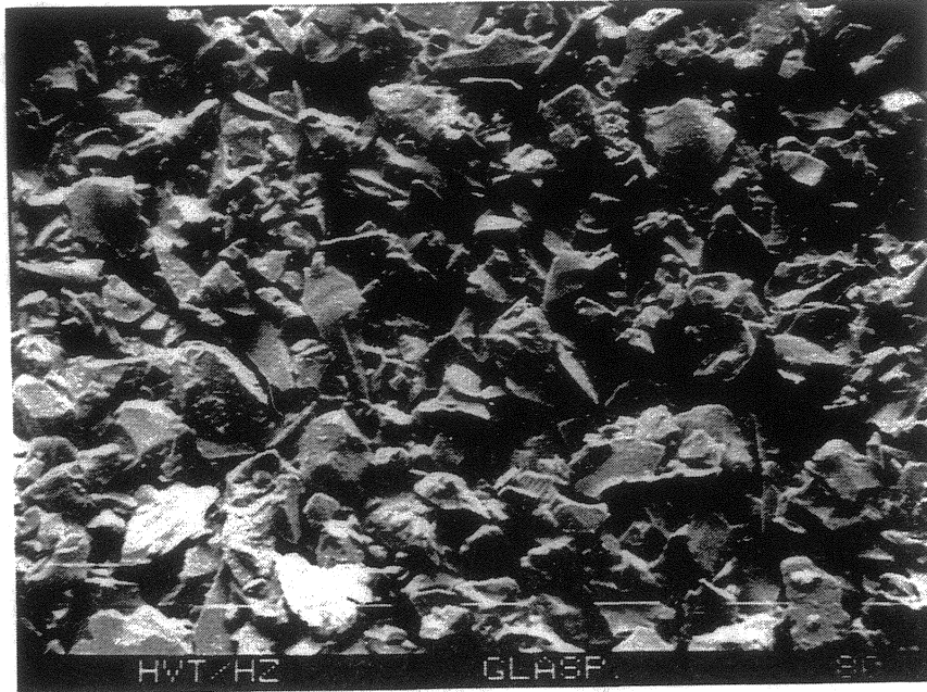
Figure 8: Glass powder for glass corrosion tests (average grain size 86 \mu\text{m} )
