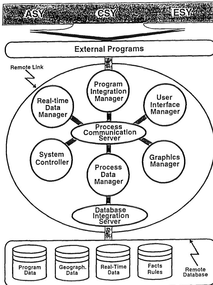
Fig. 21: Modular design of the operating subsystem OSY
