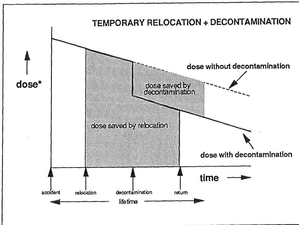
Fig. 18: Doses saved by decontaminating after temporary relocation
