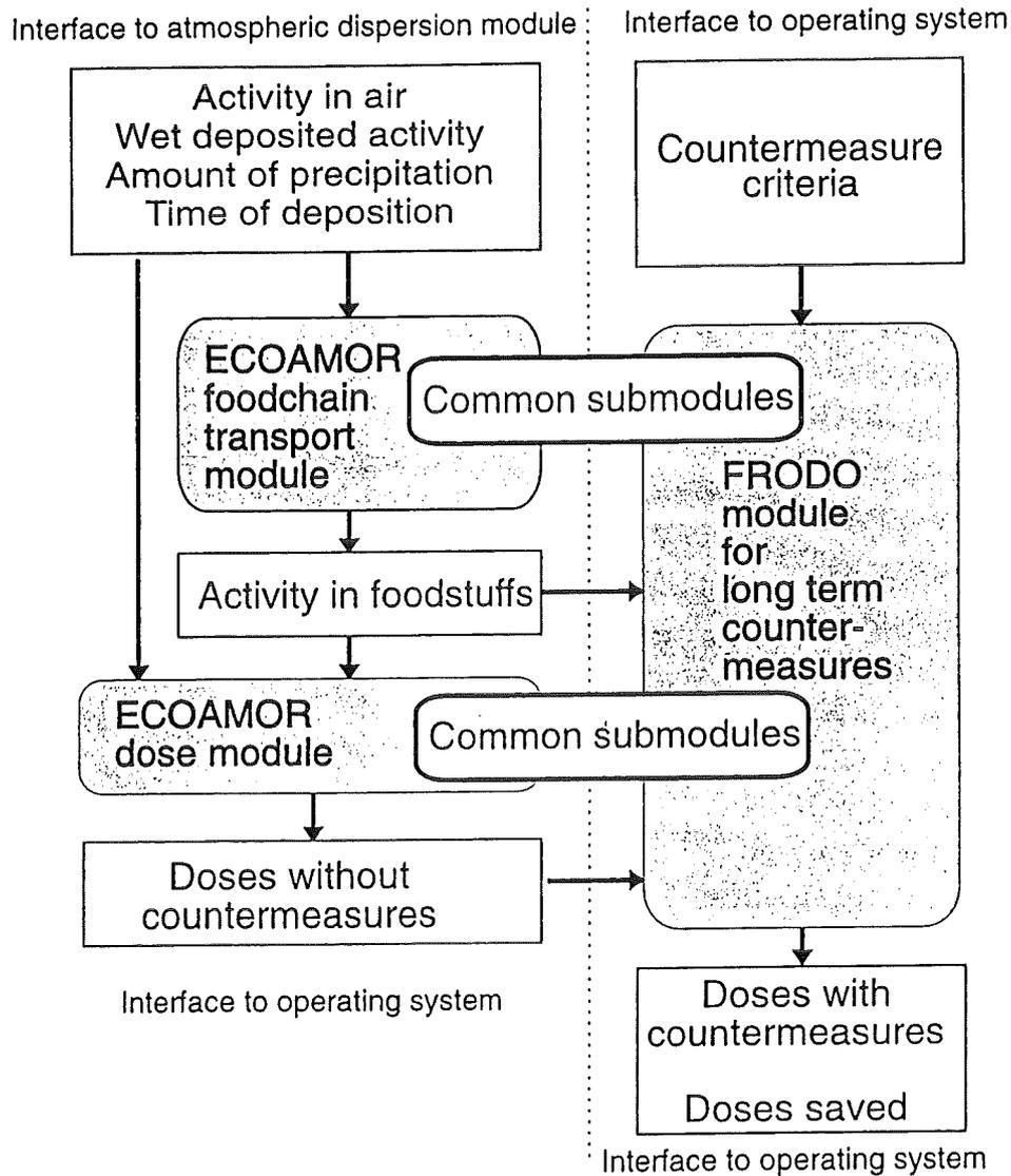
Fig. 11: Data flow in the food chain transfer and dose module ECOAMOR and the long term countermeasure module FRODO within the RODOS system
