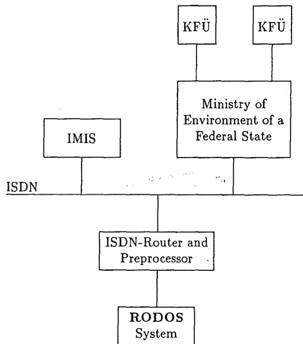
Fig. 24: Example on-line connection of the RODOS System
