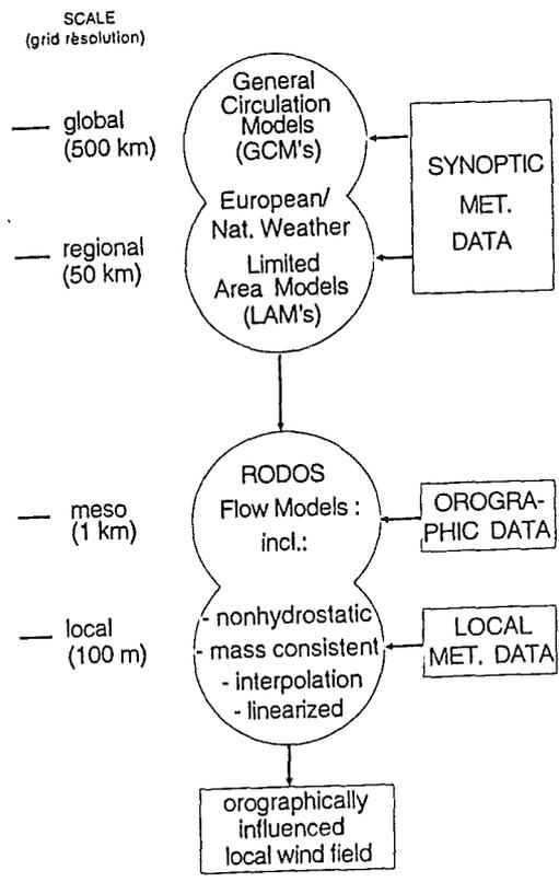
Fig. 3: Chain of meteorological flow models
