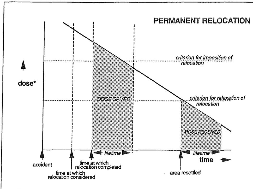
Fig. 17: Modelling of permanent relocation
