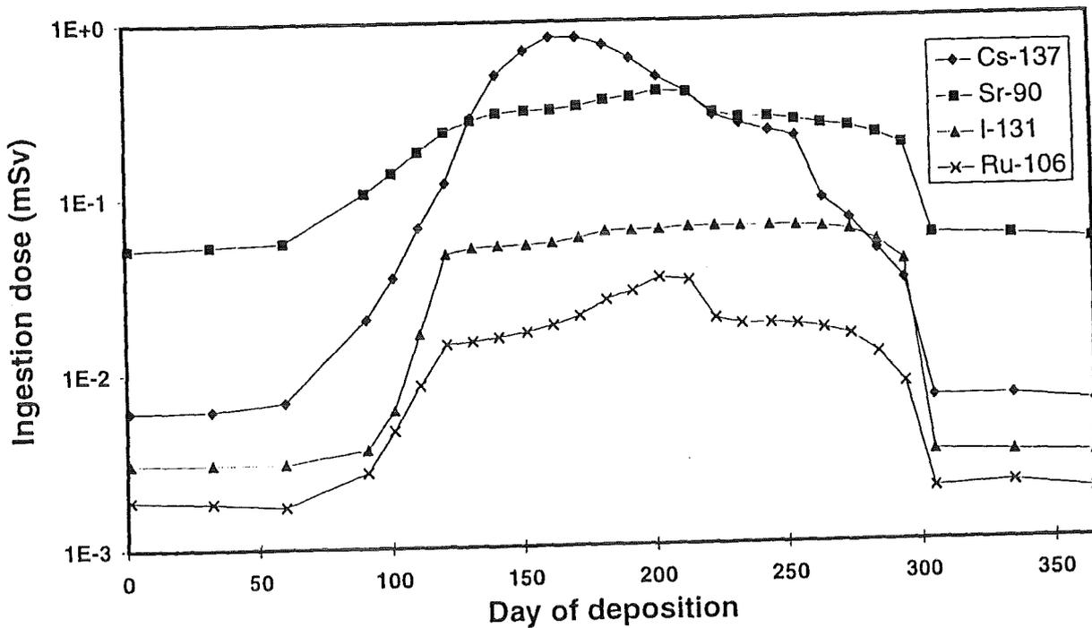
Figure 13: Dependency of lifetime ingestion dose of a 20 year old (at time of deposition) person on the time of deposition. A time-integrated activity concentration in air of  $10^6 \text{ Bq} \cdot \text{s}/\text{m}^3$  and dry deposition only has been assumed for each radionuclide and time of deposition.
