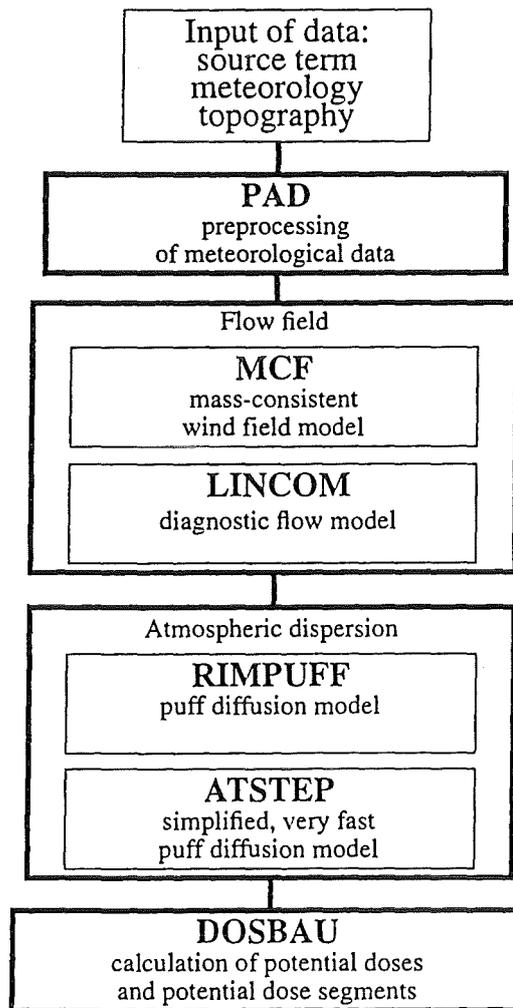
Fig. 10: Sequence of modules in ASY
