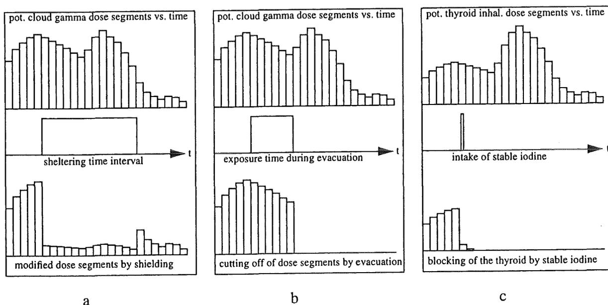
Fig. 14: Modelling of the effect of protective actions on doses
