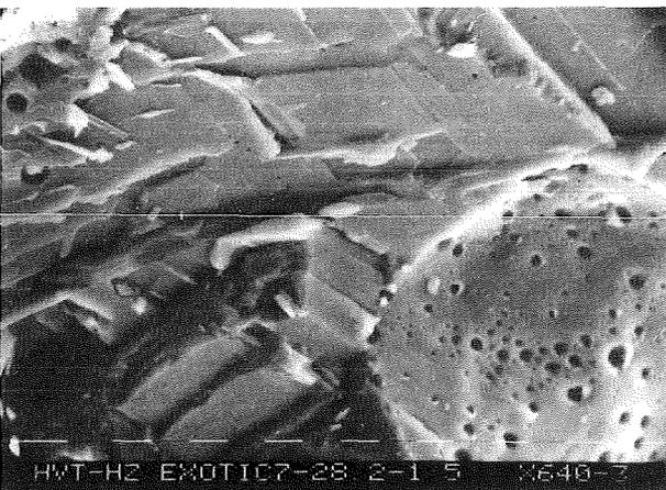
Fig. 2: Be pebble: annealed + broken
