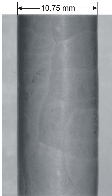
formation of macroscopic cracks
