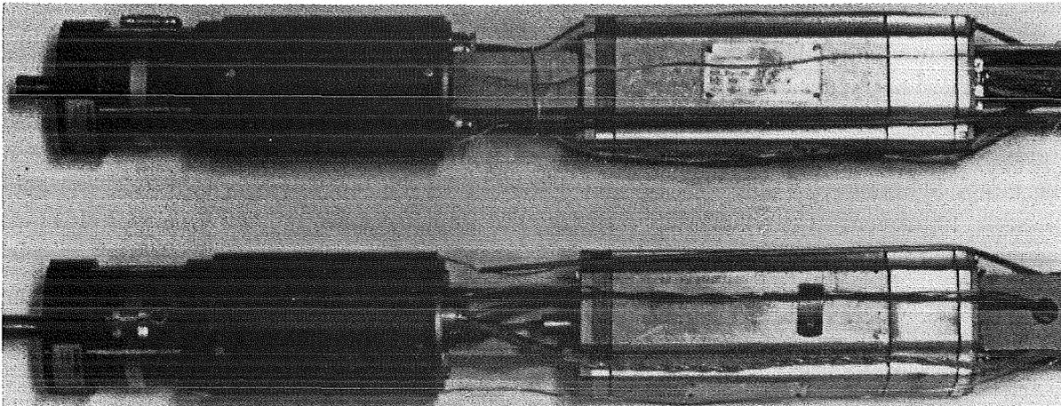
Fig. 7: Arrangement of two motors inside the basket during the irradiation
