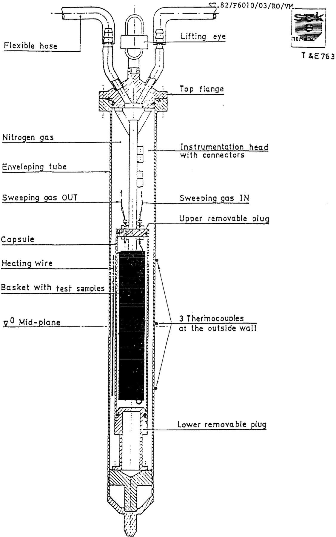
Fig. 5: General lay-out of the test rig for  $\gamma$ -irradiation
