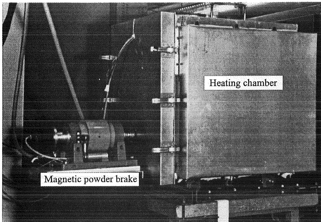
Fig. 2: Arrangement of the equipment for the pre- and post-irradiation tests
