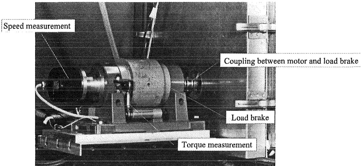
Fig. 1: Magnetic powder brake
