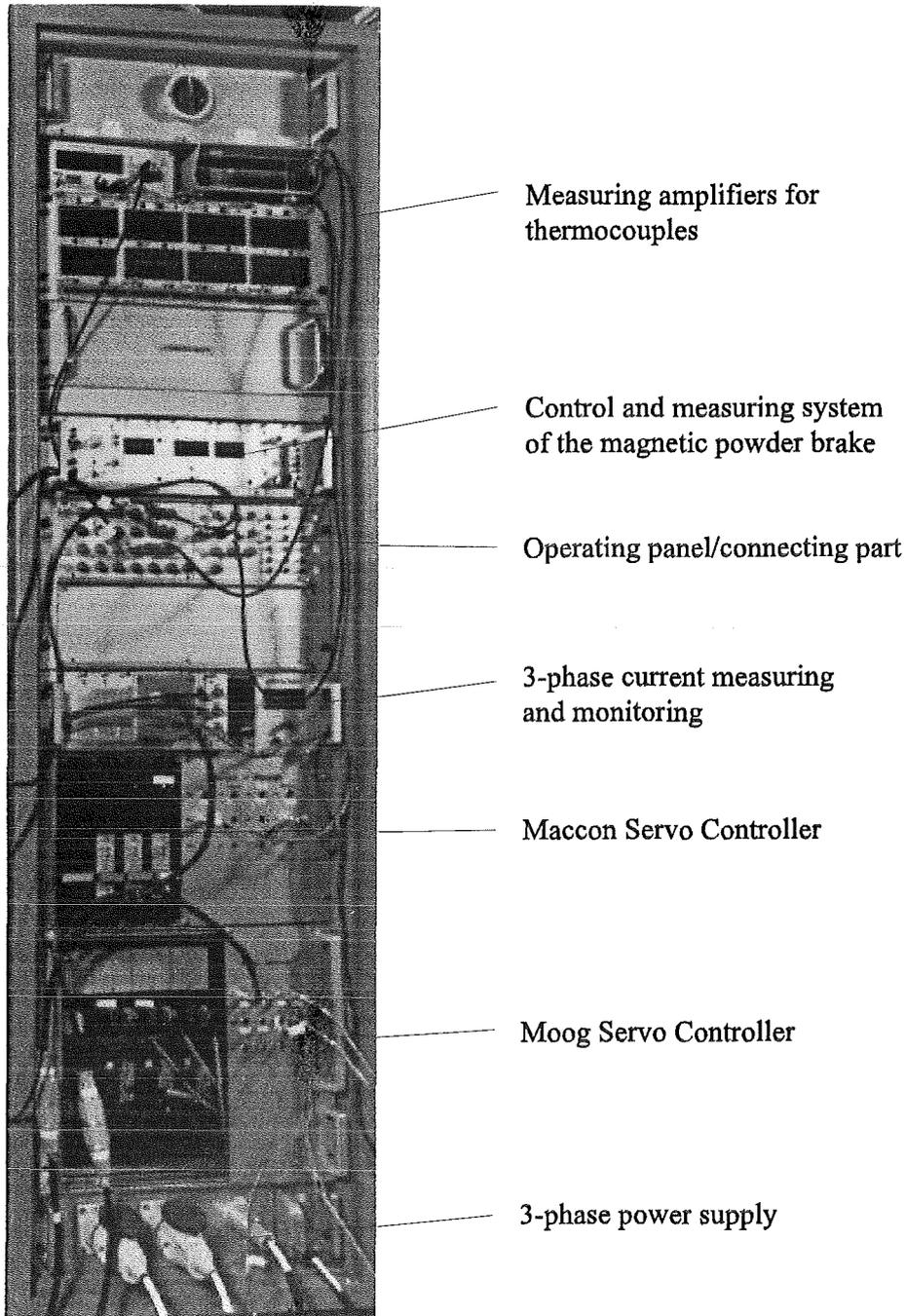
Fig. 3: Control and data acquisition rack
