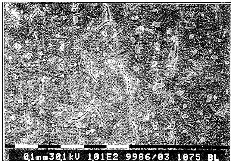
Figure 4d: Surface morphology of the heat treated sample sheet (type B: 1075°C/0.5h, 750°C/2h, x 100)
