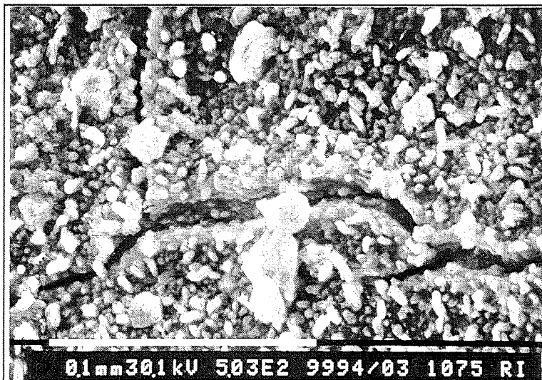
Figure 6f: Surface morphology of the heat treated sample pipe (type B: 1075°C/0.5h, 750°C/2h, inside wall, x 500)
