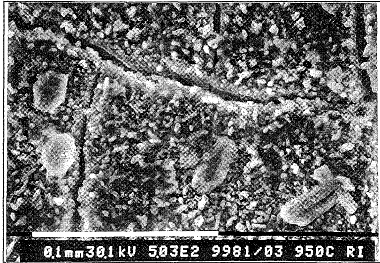
Figure 6c: Surface morphology of the heat treated sample pipe (type A: 950°C/2h, 750°C/2h, inside wall, x 500)
