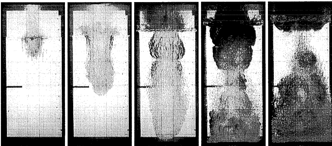
Figure 10. High speed photographs of 20 kg Mo-spheres (4.3 mm), Q-36 ( t = 500-900 ms, 100 ms interval)
