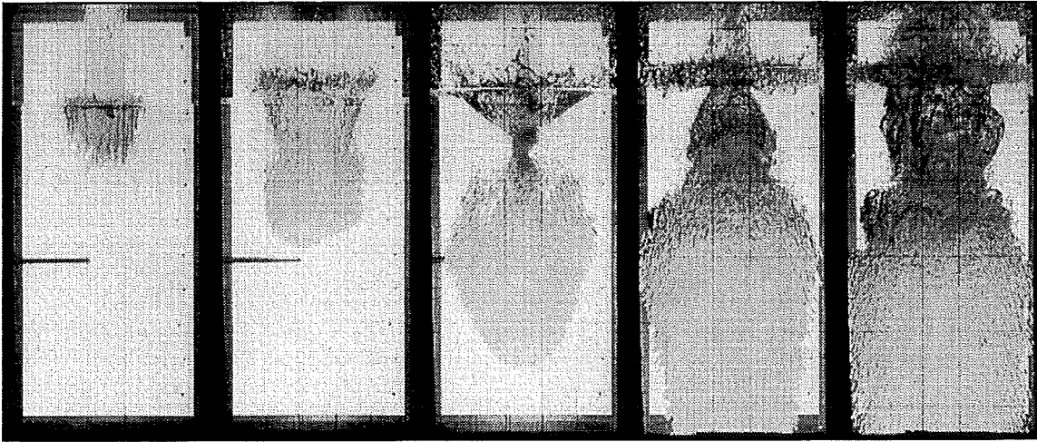
Figure 5. High speed photographs of 7 kg zirconia spheres (5 mm), Q-31. ( t = 500-900 ms, 100 ms interval)
