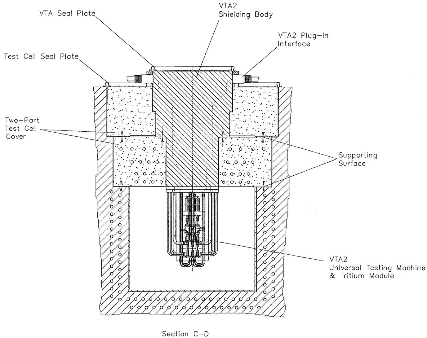
**Fig. 12:** Front view of the VTA2 with the creep-fatigue test module integrated in the test cell; version with gas cooled concrete.
