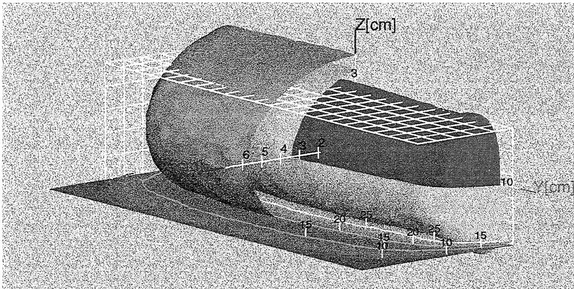
Displacement damage cutout isosurfaces. Each isosurface characterises the available volume for a DPA/FPY limit. Green = 20 DPA/FPY, yellow = 30 DPA/FPY and red = 40 DPA/FPY. The grid structure shows the physical boundary of the helium cooled high flux test module. (MCNP collided, McDeLi data, non-uniform beam profile.)
