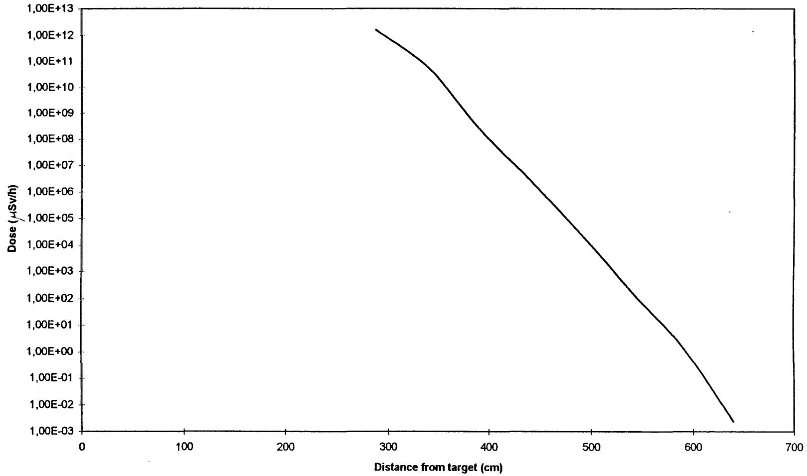
Fig.9 - Test Cell Frontal wall neutron attenuation with Assembly.
