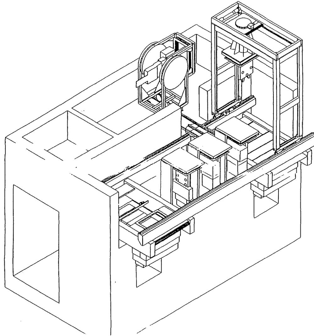
**Fig. 11:** Transfer device moving a Vertical Test Assembly between Access Cell and Service Cell.
