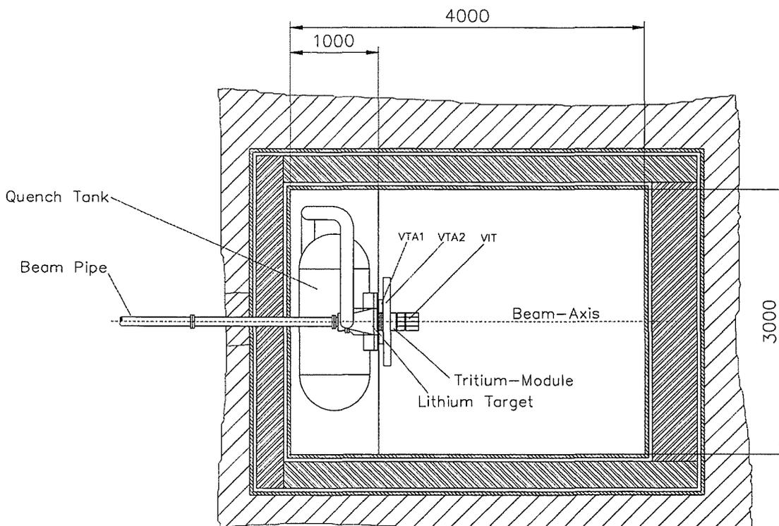
**Fig. 4:** Plan view of the test cell with lifted removable cover; stainless steel heat shield (all dimensions in mm).
