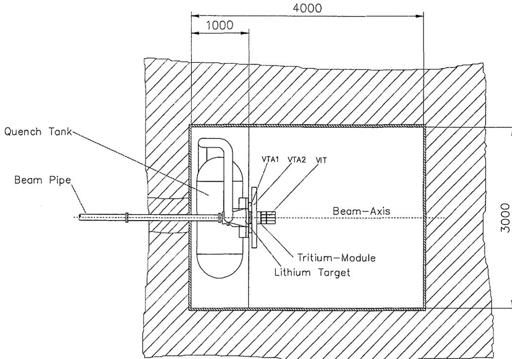
**Fig. 3:** Plan view of the test cell with lifted removable cover; gas cooled concrete walls (all dimensions in mm).
