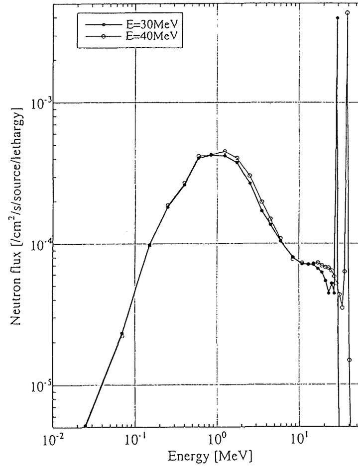
Fig. 3.8 Neutron spectra at radius 10cm in 10cm-radius sphere of  $^{56}\text{Fe}$  for checking the JENDL High-Energy File.
