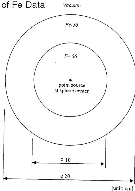
Fig. 3.1 Test calculation model (10 cm-radius sphere) of JENDL high-energy library for the MCNP code.
