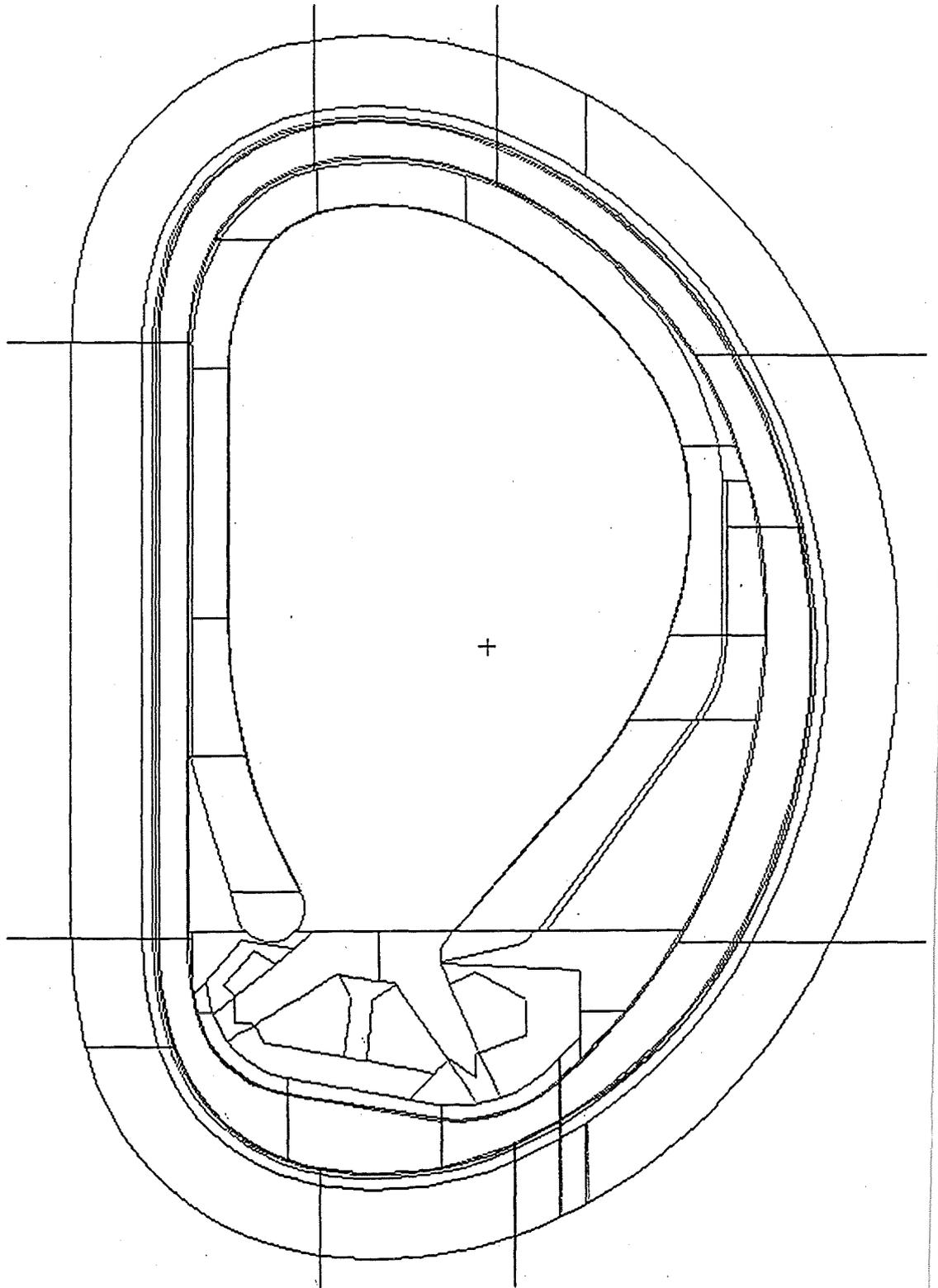
Horizontal cross-section (x-y plane) of the IFMIF helium cooled high flux test module (MCNP model with assigned cell numbers)
