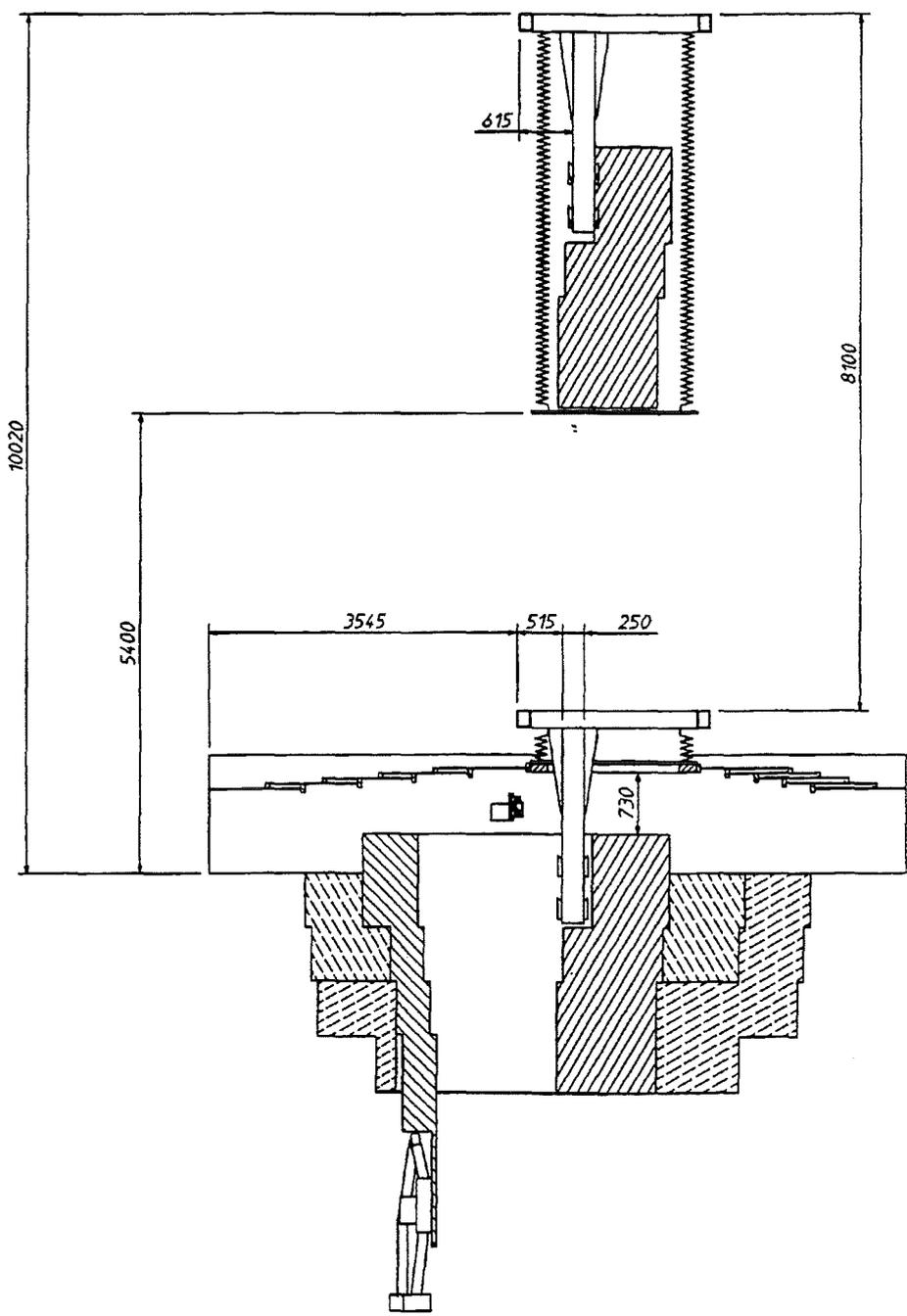
**Fig. 8:** Remote handling procedure; Gripper/bag gripping the test cell removable cover.
