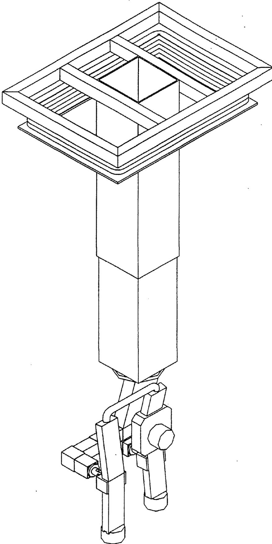
**Fig. 3:** telescopic tool of the Universal robot system.
