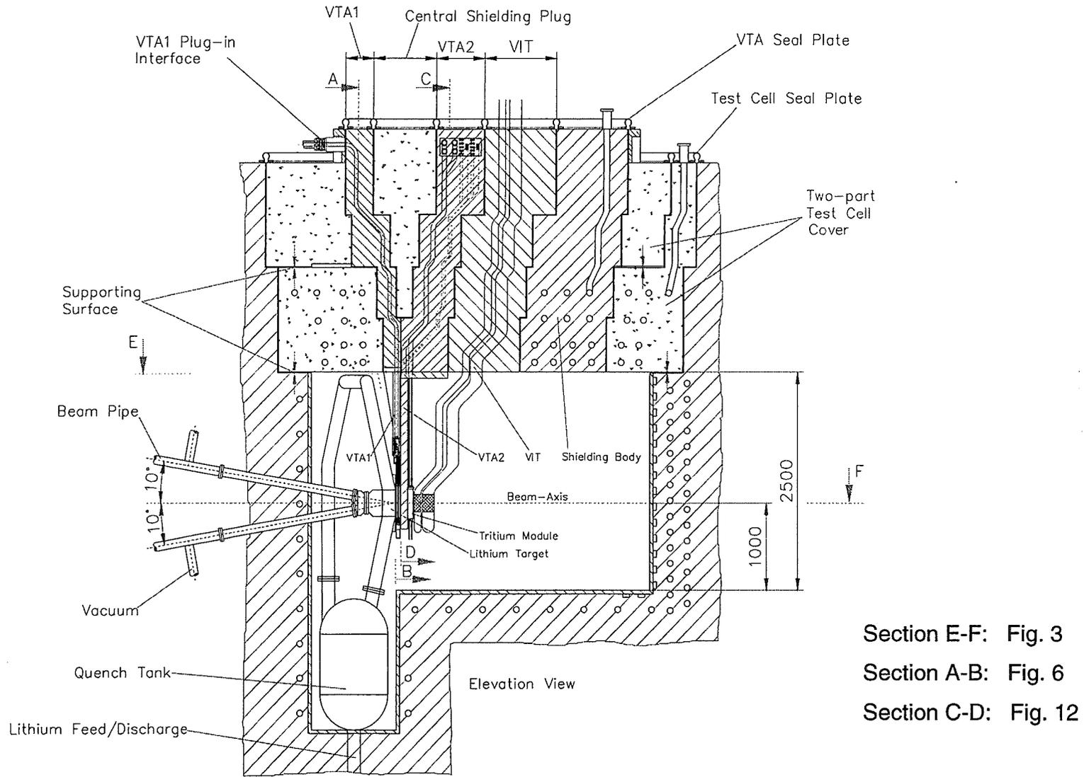
**Fig. 1:** Elevation view of the complete test cell arrangement (all dimensions in mm). In this version the test cell walls are cooled by gas coolant passages inside the concrete.
