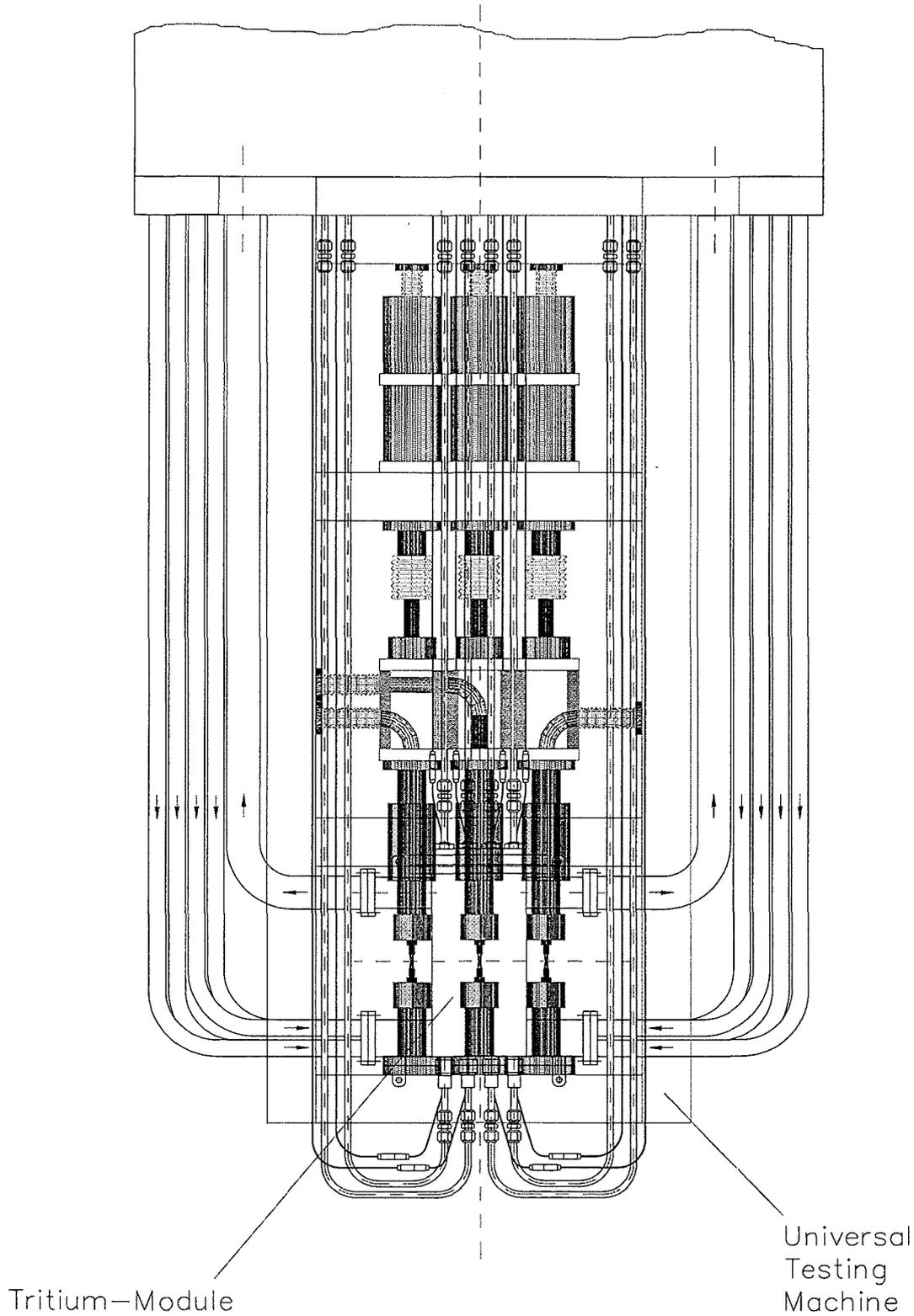
**Fig. 14:** Back view (upstream direction) showing the test module for tritium release experiments (foreground) and the test module for in-situ creep-fatigue tests (background).
