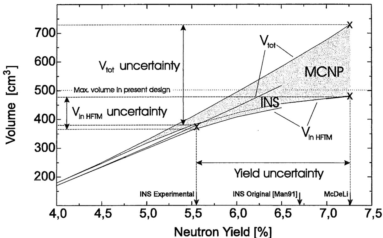
Irradiation volume for displacement damage > 20 DPA/FPY as a function of the total neutron yield (uncollided calculations MCNP and INS 'experimental').
