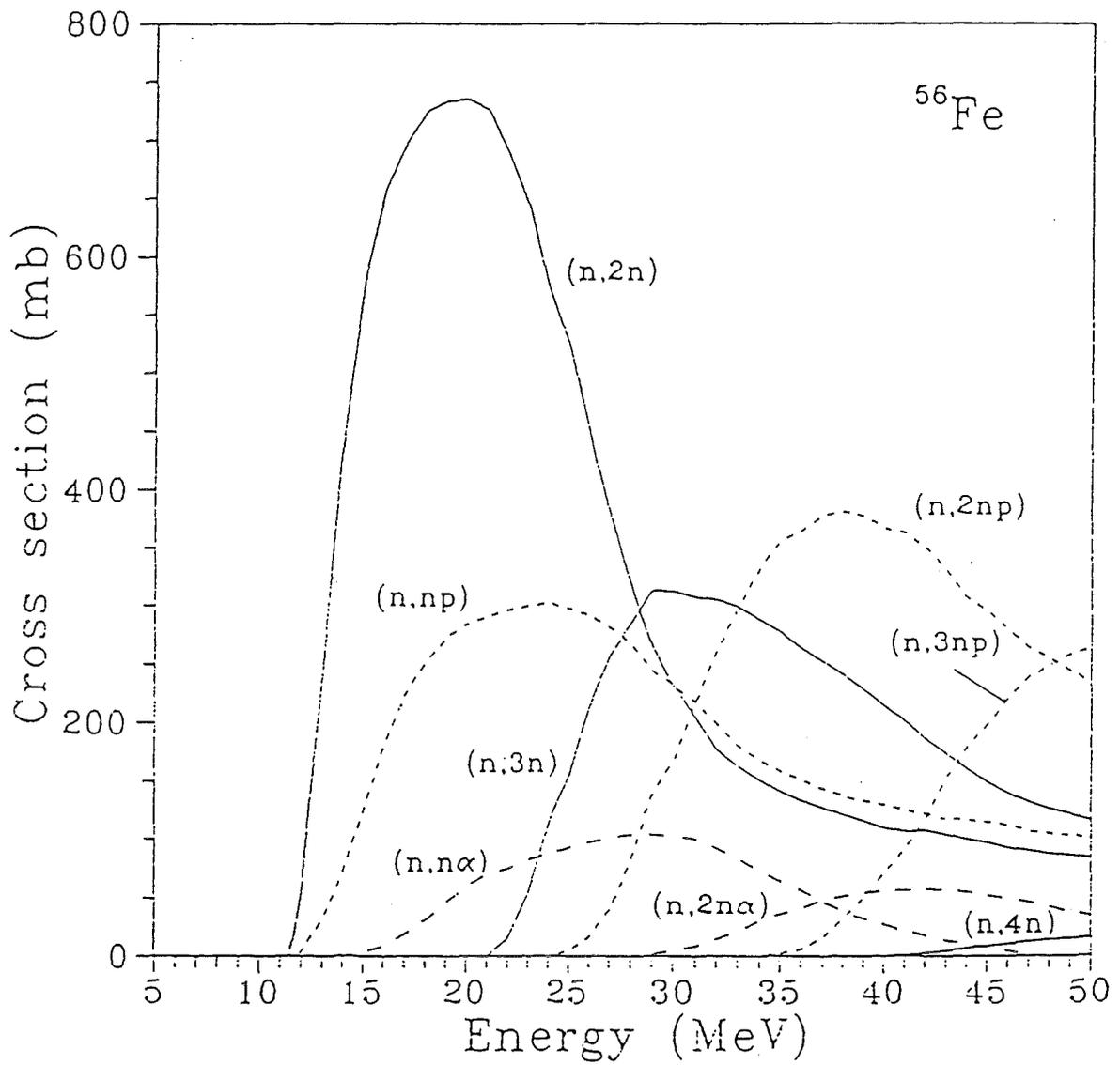
**Fig. 2:** Cross sections of kinematically possible neutron reactions in Fe-56
