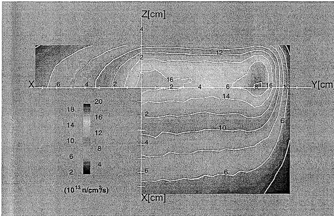
Figure 5. High Energy (> 14.6 MeV) Neutron Flux
