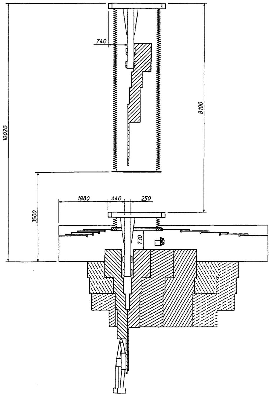
**Fig. 6:** Remote handling procedure; Gripper/bag gripping the VTA2.
