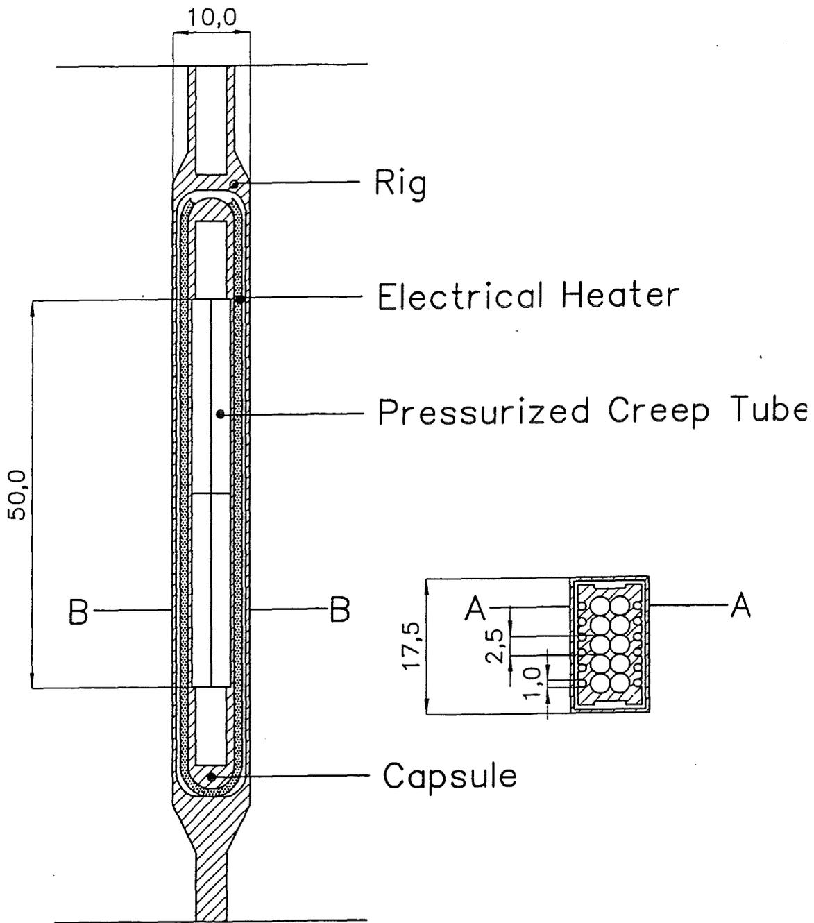
Rig with Pressurized Creep Tubes
