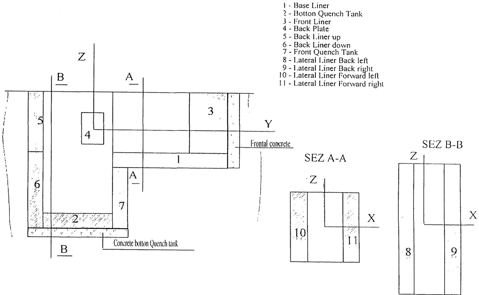
Fig. 30 - SS Liner Activation sources after irradiation
