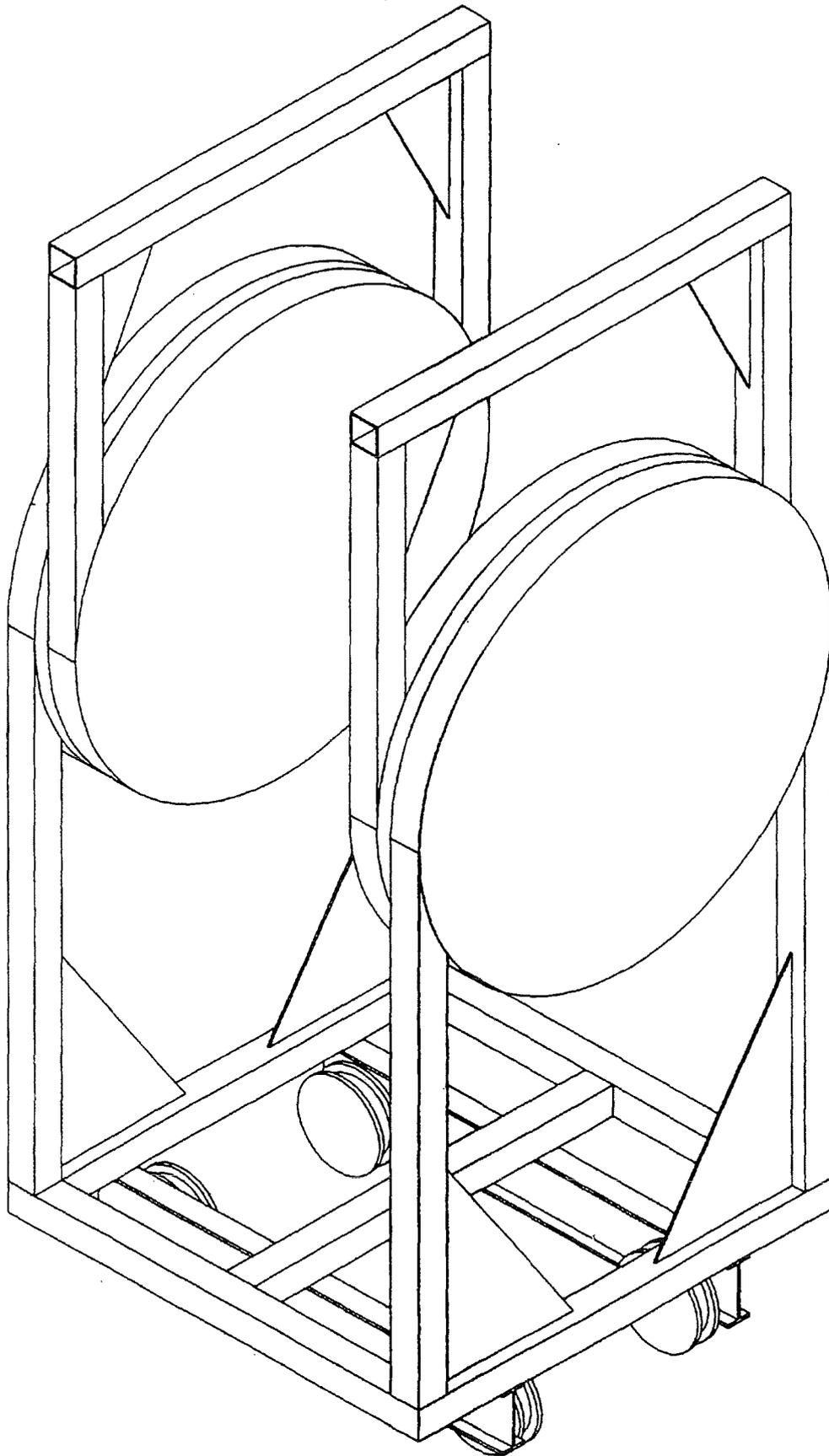
**Fig. 9:** Transfer device to move VTAs between Service Cell and Access Cell.
