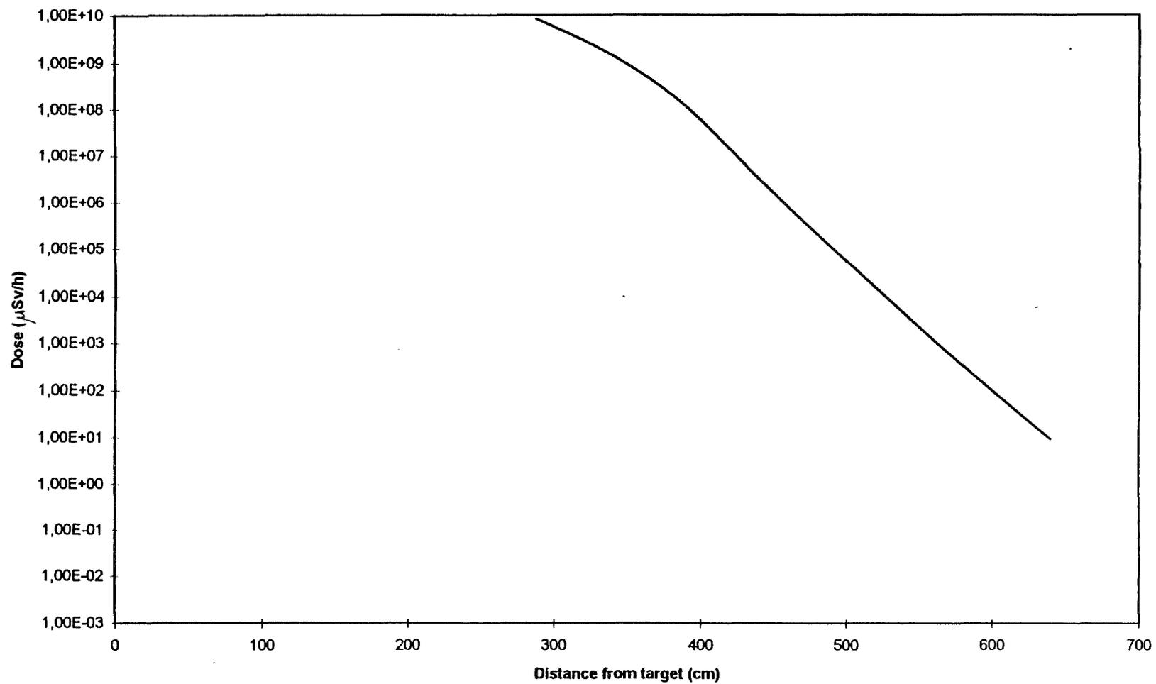
Fig.10 - Test Cell Frontal wall gamma attenuation with Assembly.
