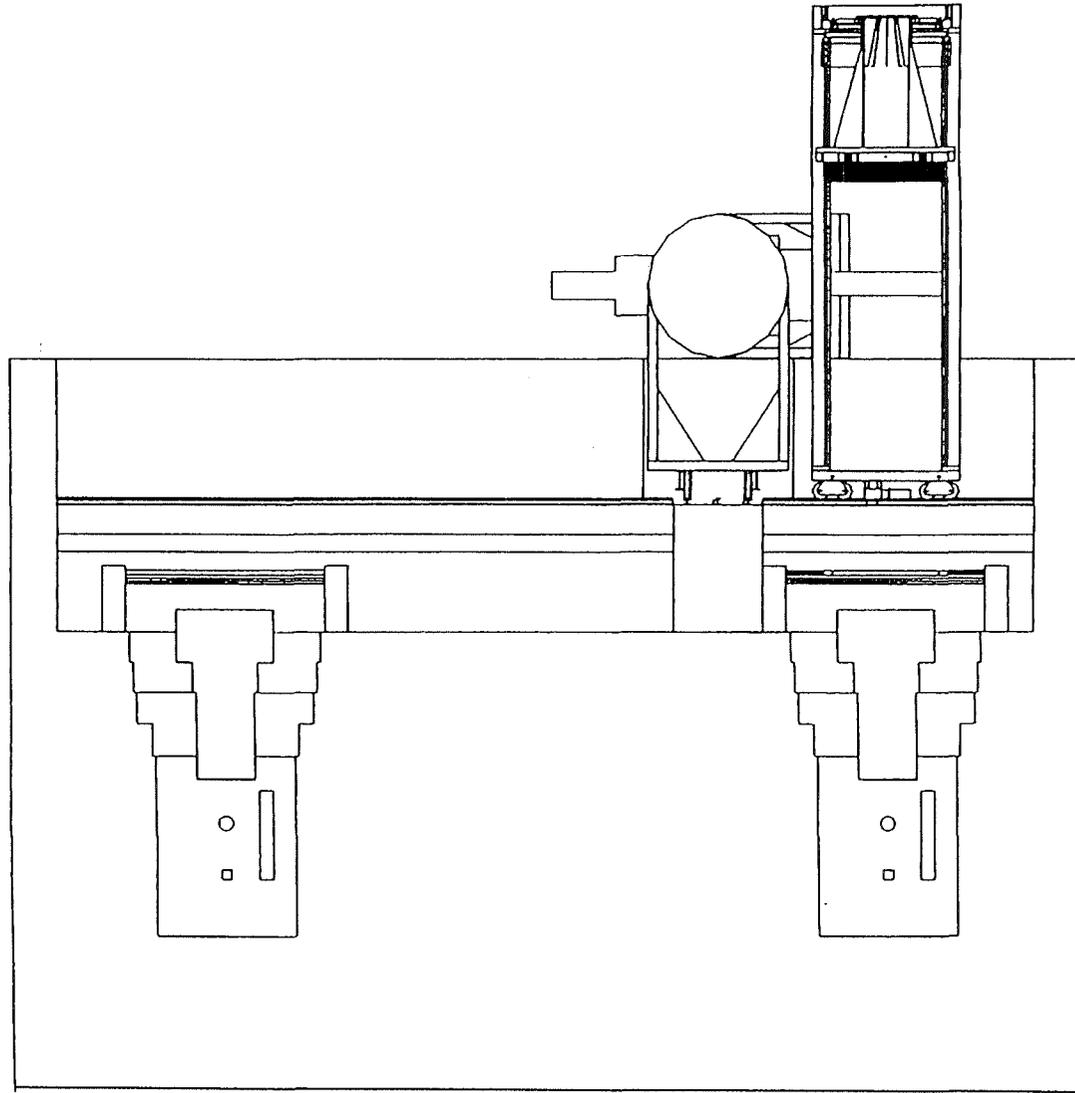
**Fig. 12:** Elevation view with the universal robot system, the transfer device (gripping a VTA) and the two test cells
