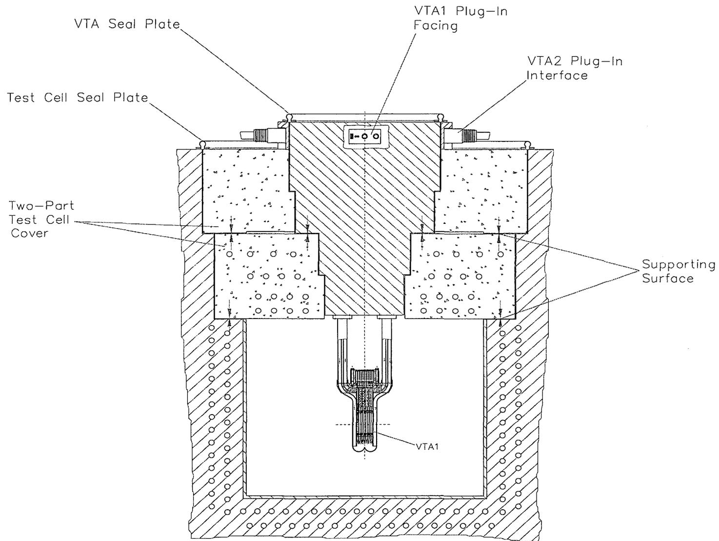
**Fig. 6:** Improved design configuration for VTA1 with assembled high flux test module; front view.
