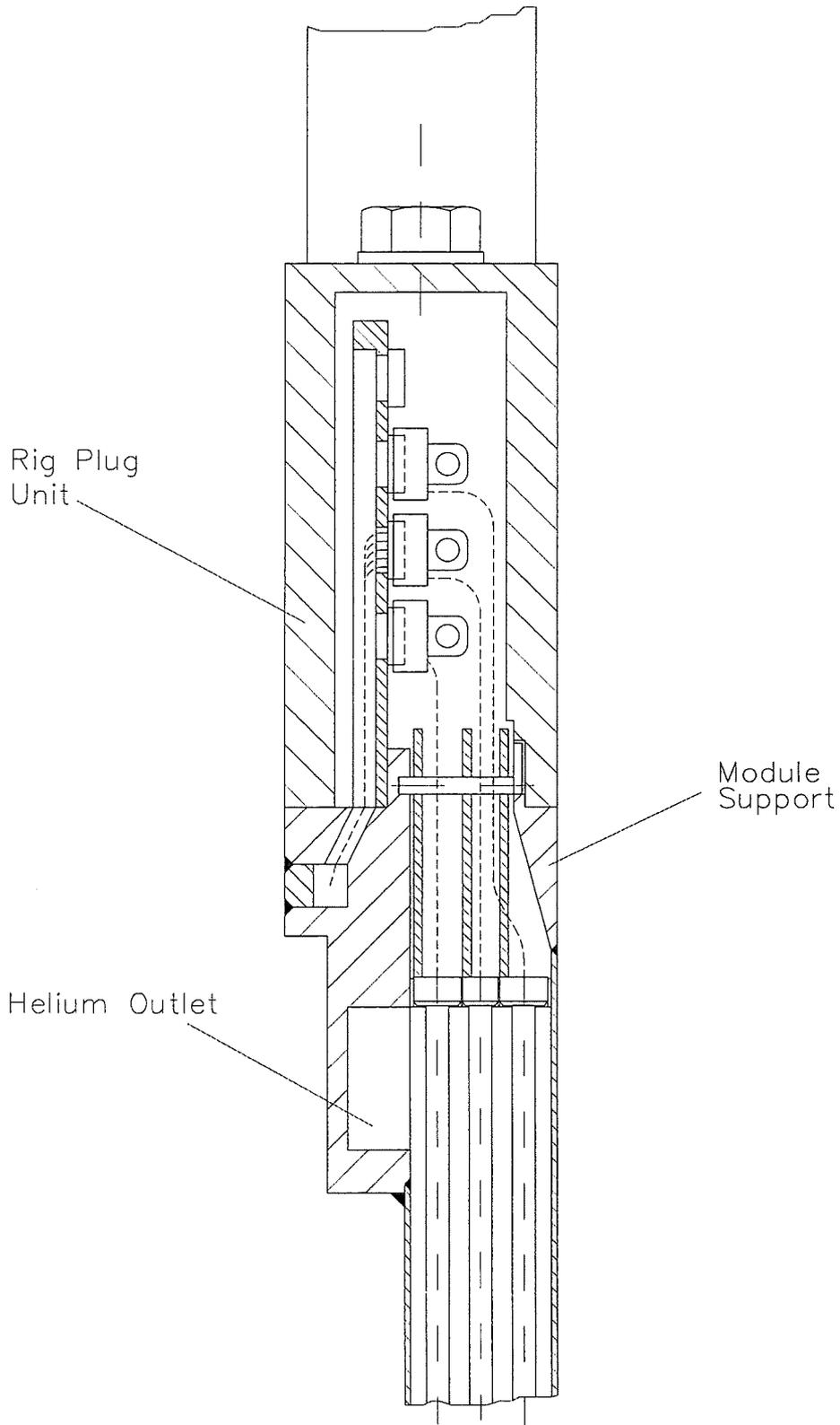
**Fig. 10:** Elevation view of the upper part of the helium gas cooled high flux test module.
