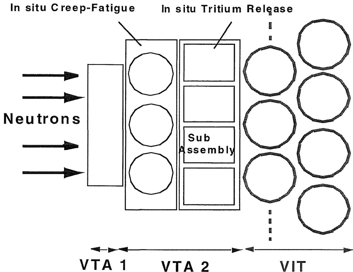
**Fig. 11:** Updated reference concept of the test module arrangement; VTA2 is assembled with two independent test modules for different types of in-situ experiments.
