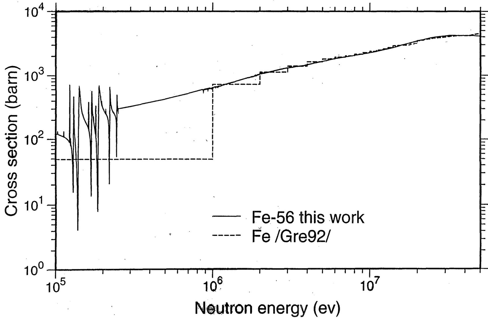
Fig. 3: Fe displacement cross sections
