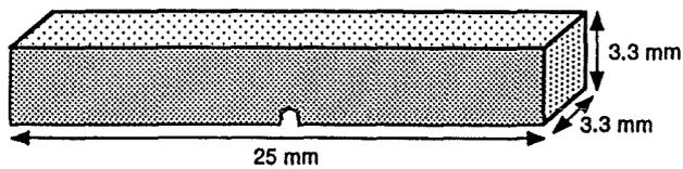
e) Dynamic/static fracture toughness
