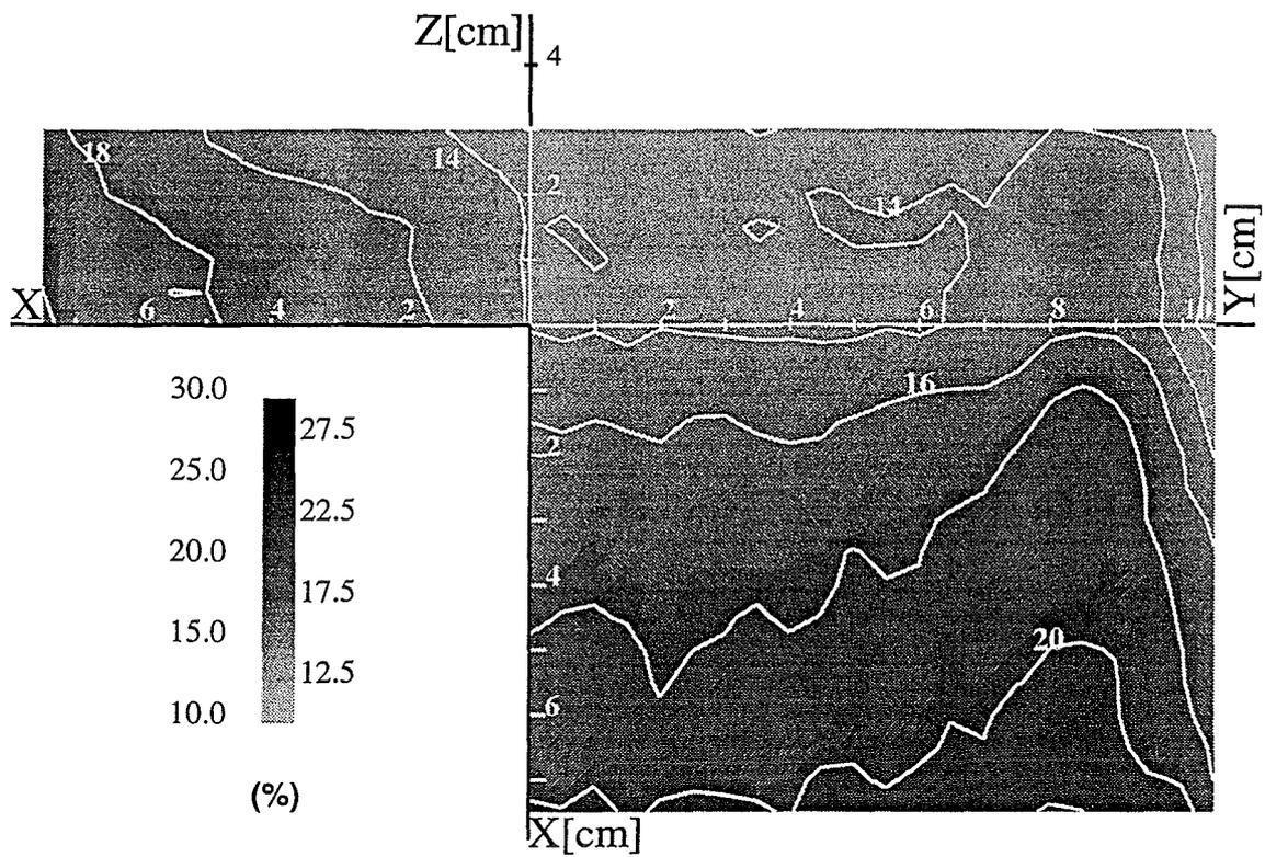
Figure 6. High Energy (>14.6 MeV) Neutron Flux Fraction
