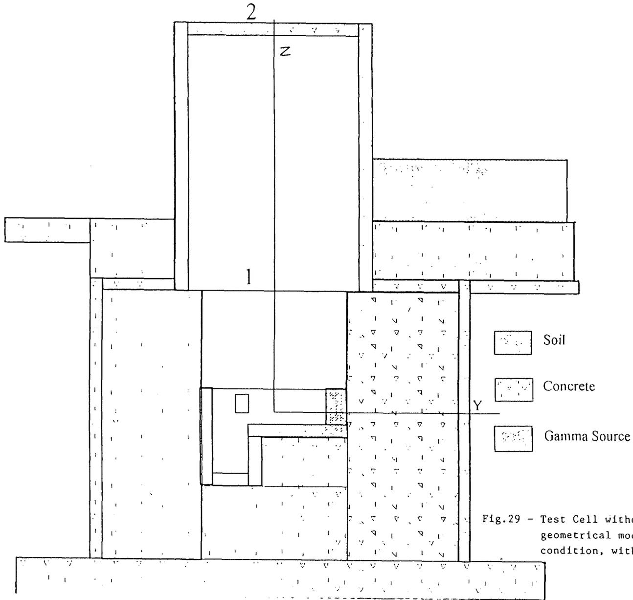
Fig.29 - Test Cell without plug MCNP geometrical model (shut down condition, without plug).
