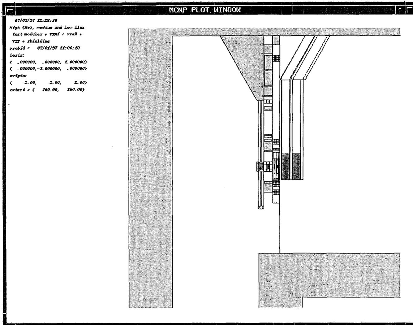
Fig. 8 Test modules with He cooled high flux test cell
