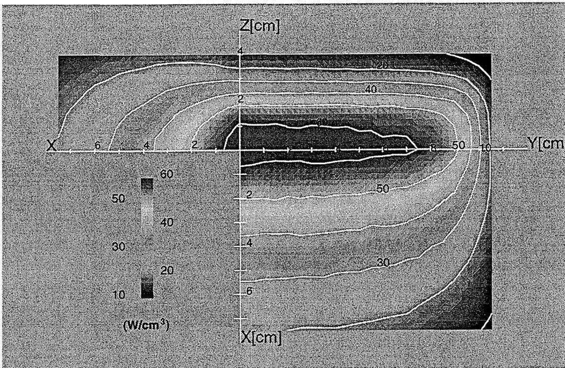
Figure 17. Nuclear Heating [uniform beam profile]
