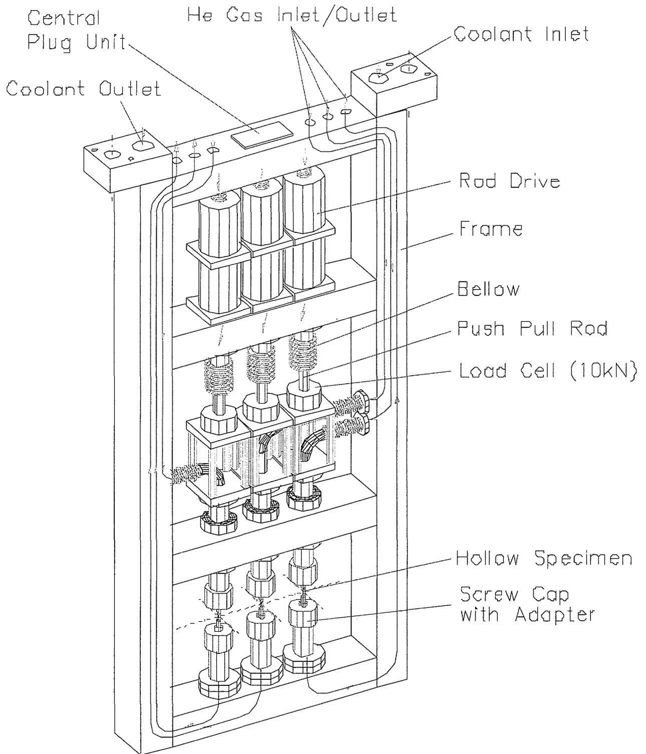
**Fig. 15:** Test module for in-situ creep-fatigue experiments on three independent specimens.
