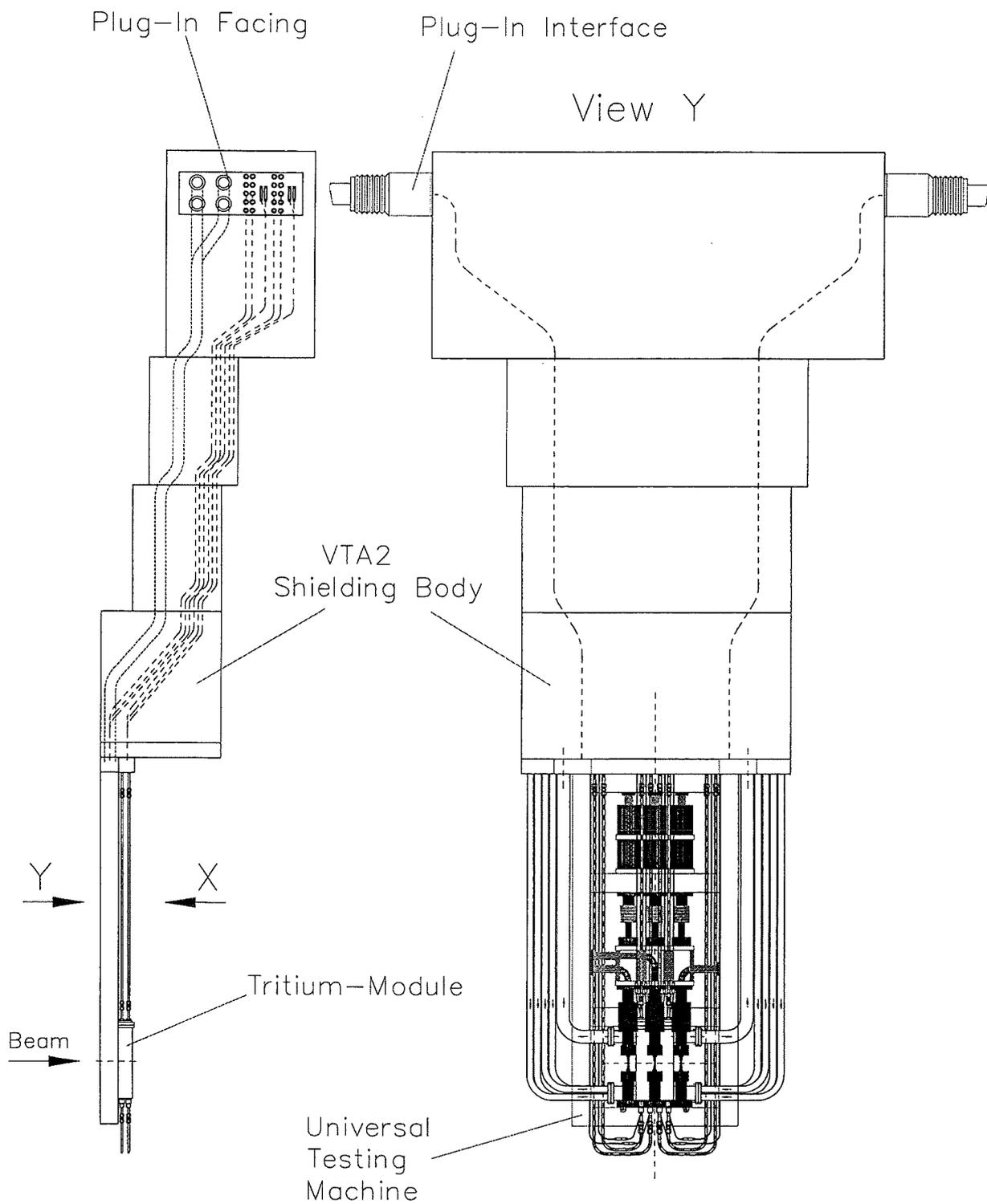
**Fig. 13:** VTA2 equipped with a test module for in-situ creep fatigue tests and another one for tritium release tests. The elevation (left side) and front views (right side) are shown.
