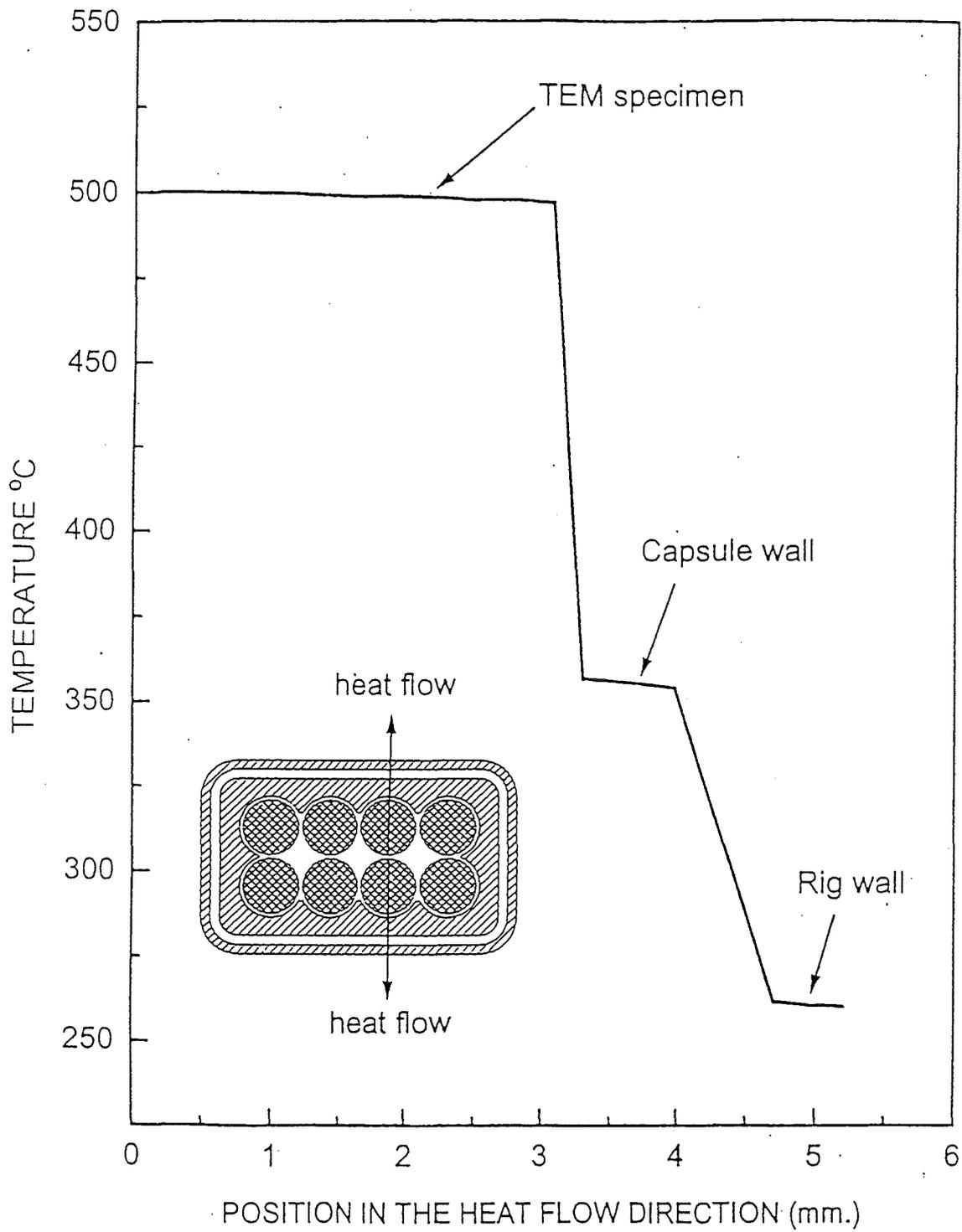
**Fig. 4:** Temperature Distribution over TEM Disk Specimen Rig
