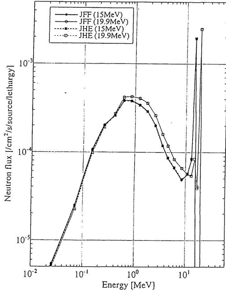
Fig. 3.3 Neutron spectra at radius 10cm in 10cm-radius sphere of  $^{56}\text{Fe}$  for checking the JENDL High-Energy File.
