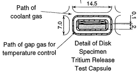
Detail of Disk Specimen Tritium Release Test Capsule
