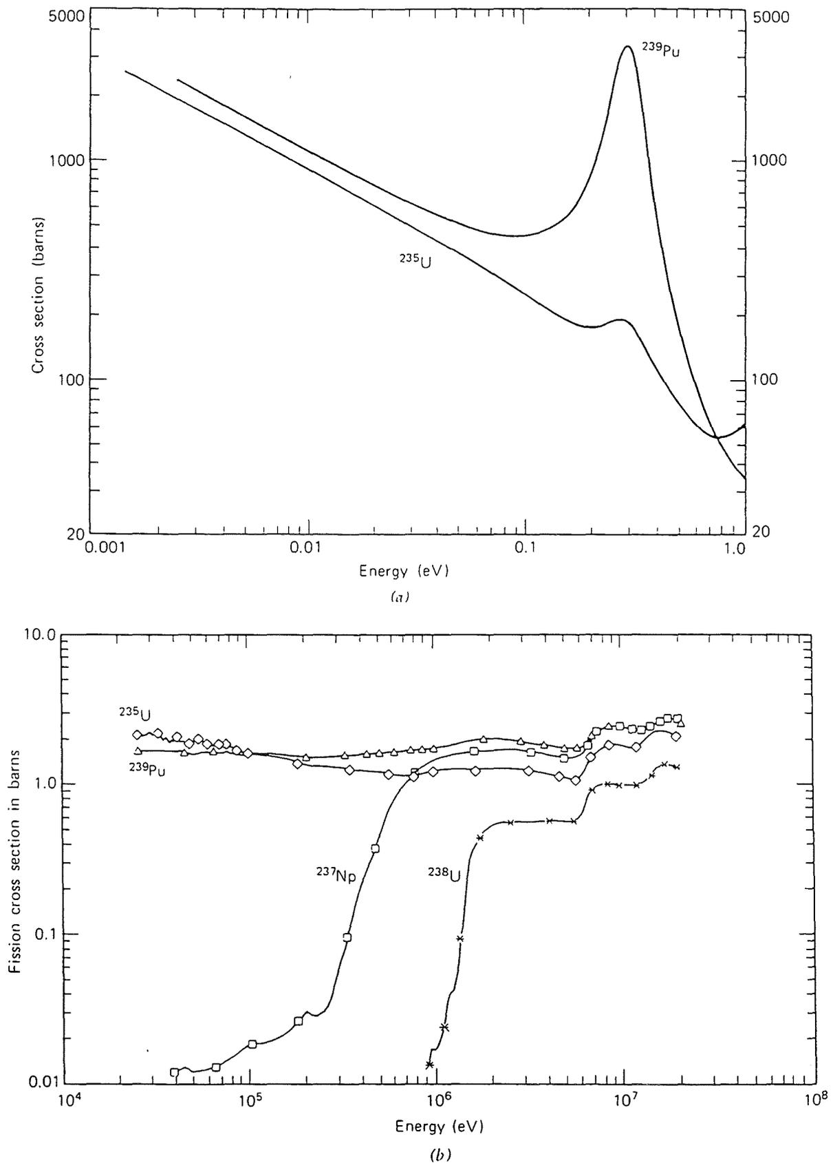
FIGURE 14-2. Fission cross sections of some common target nuclides used in fission chambers. Part (a) includes the slow neutron region where the cross sections shown are relatively large. The fast neutron region is shown in (b). Chambers with  $^{237}\text{Np}$  or  $^{238}\text{U}$  are used as "threshold detectors" sensitive only to fast neutrons.
