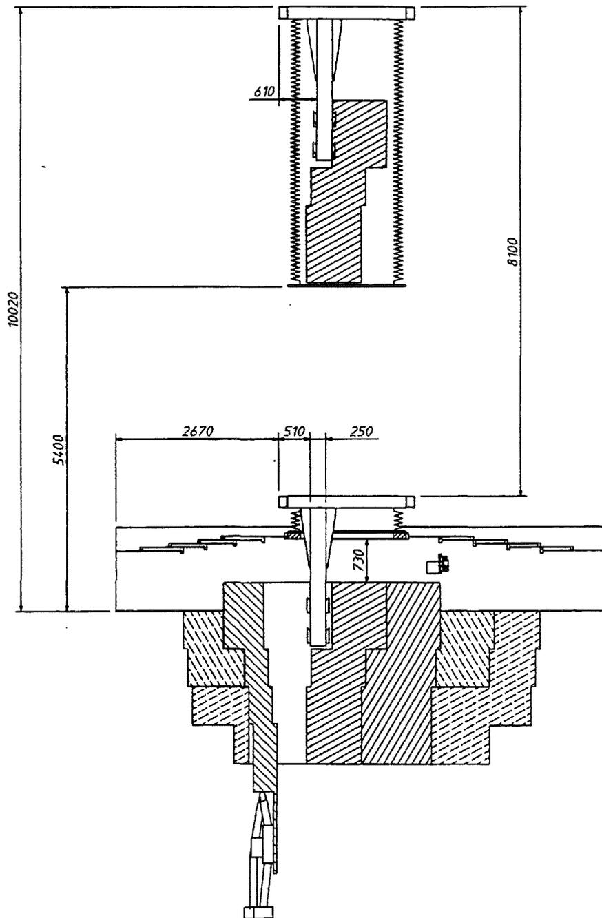
**Fig. 7:** Remote handling procedure; Gripper/bag gripping the Vertical Irradiation Tube (VIT) system.
