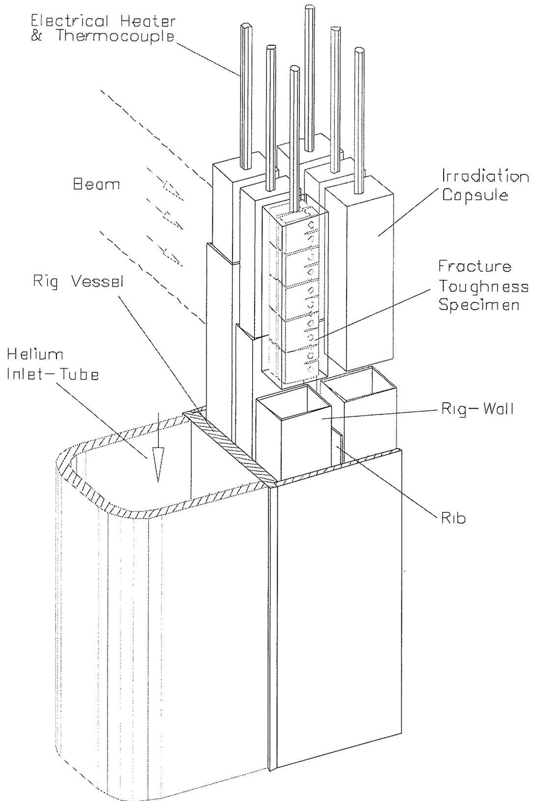
**Fig. 9:** Helium cooled high flux test module with vertical rigs that accommodate the encapsulated specimens.
