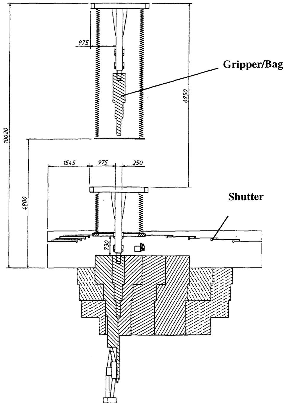
Fig. 4: Remote handling procedure; Gripper/bag gripping a shield plug.
