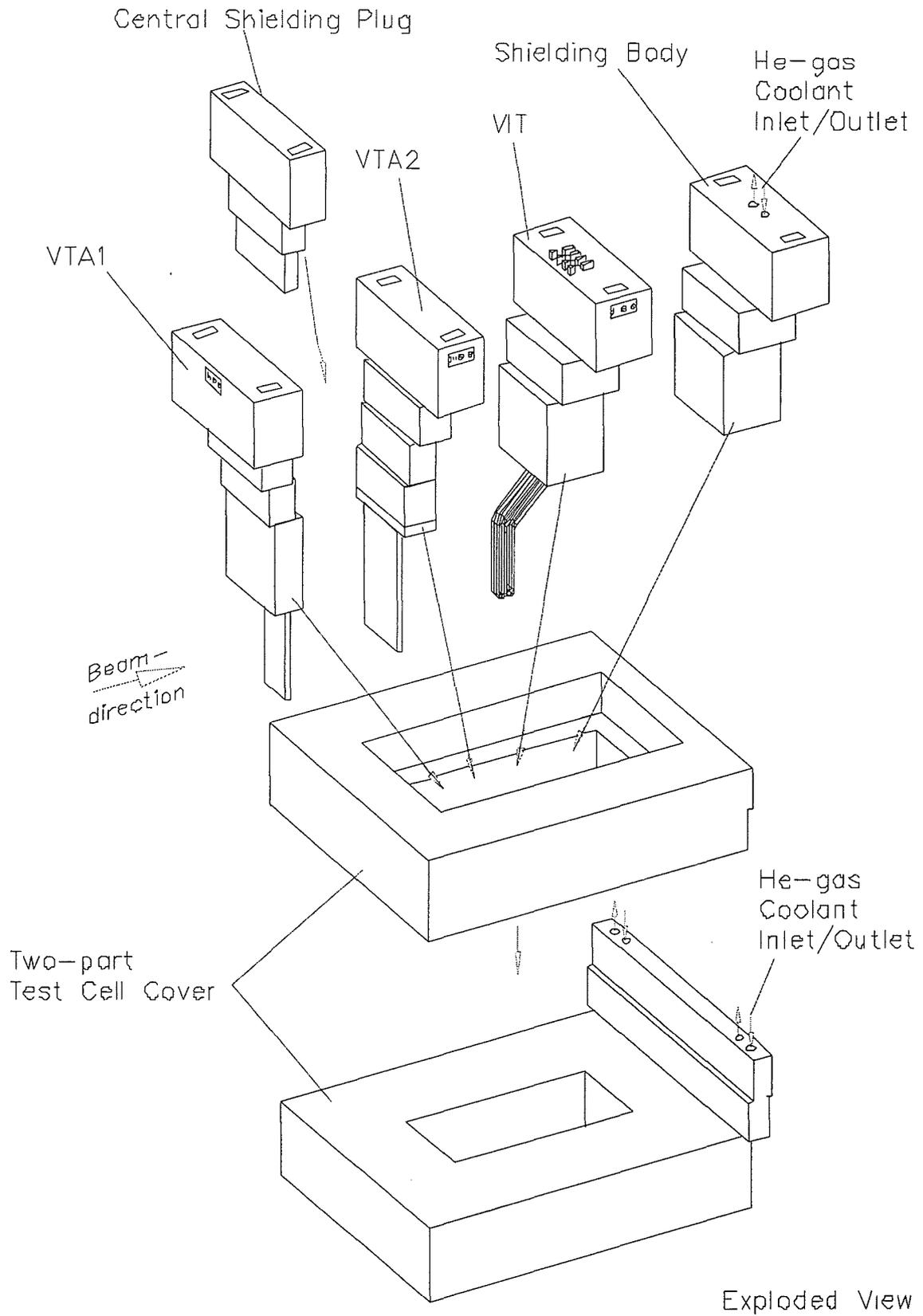
**Fig.5:** Explosion view of the test cell design concept.
