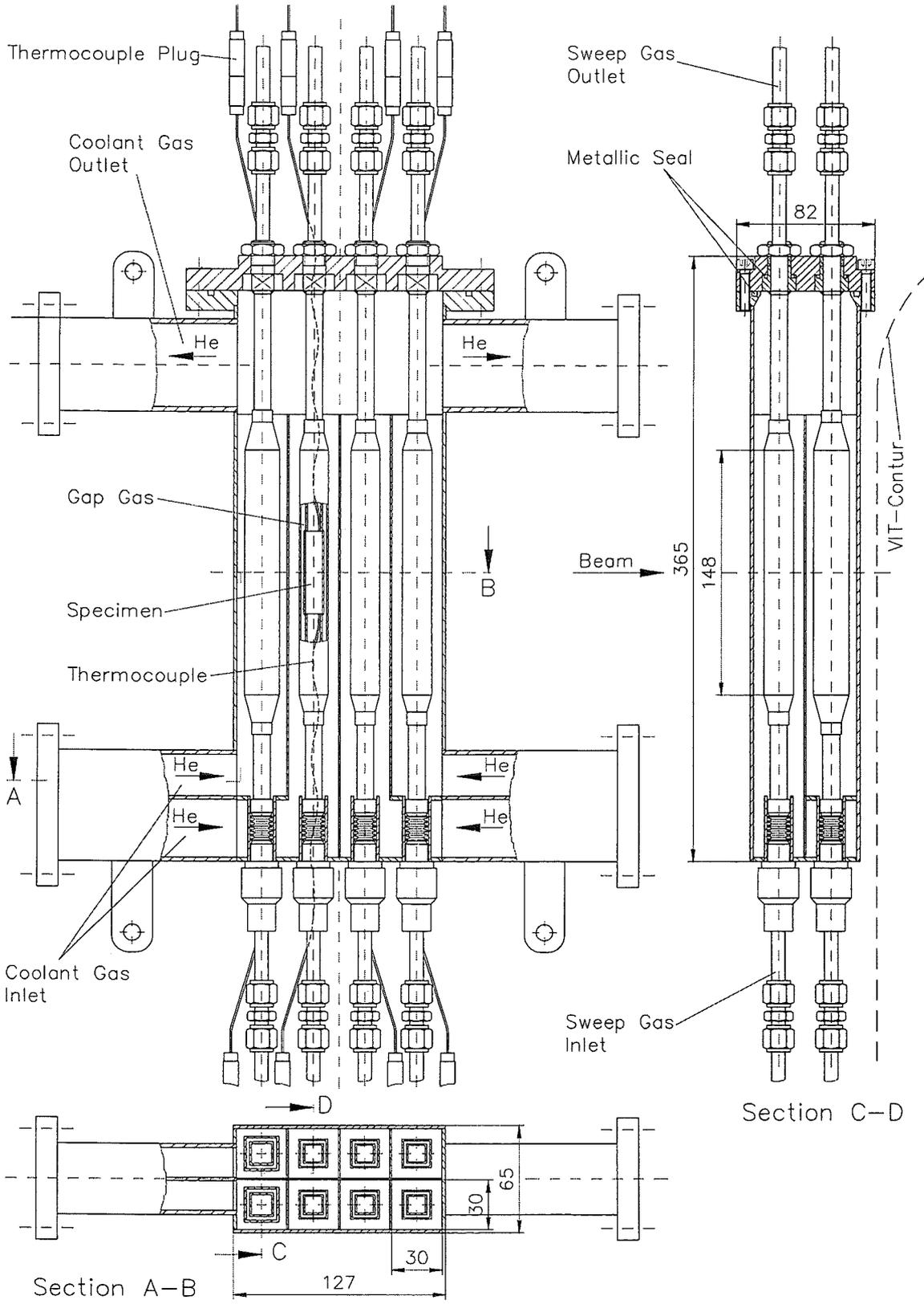
**Fig. 16:** Test module for in-situ tritium release experiments on ceramic specimens
