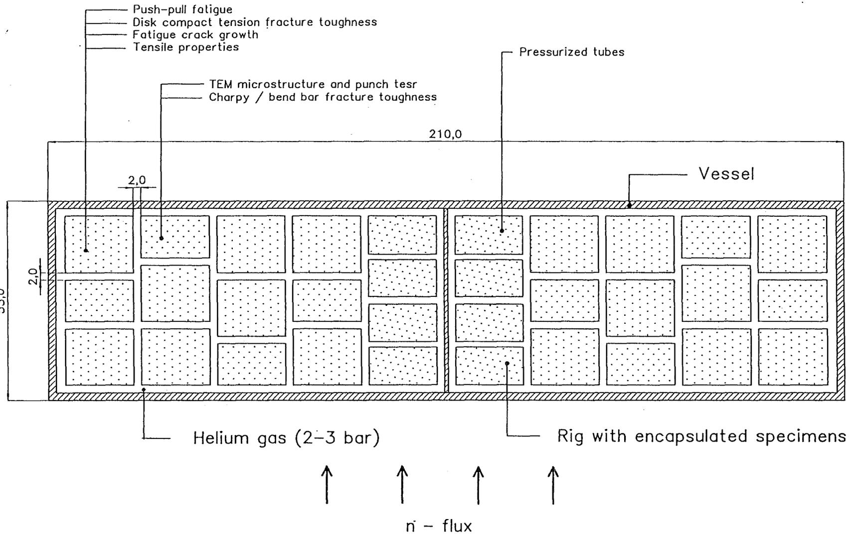
**Fig. 5:** Top View of Helium Gas Cooled High Flux Test Module
