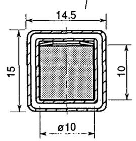
Detail of Pellet Specimen Tritium Release Test Capsule
