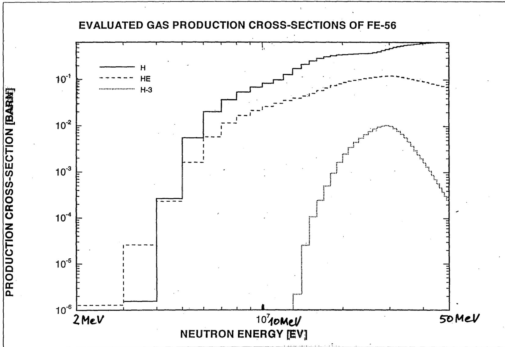
Fig. 4: Evaluated gas production cross sections of Fe-56
