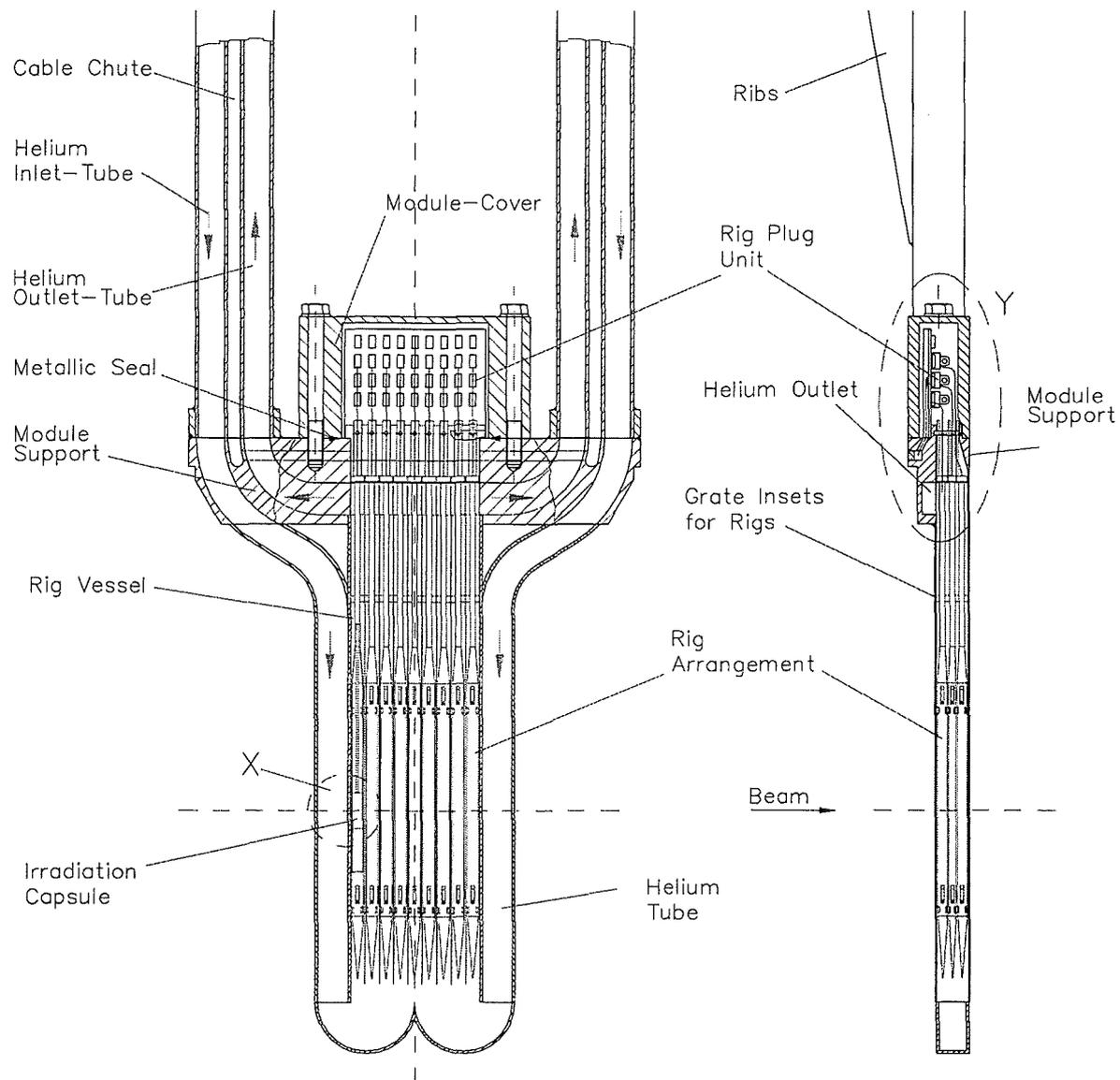
**Fig. 1:** Front an elevation view of the updated Design configuration for the helium gas cooled high flux test module.
