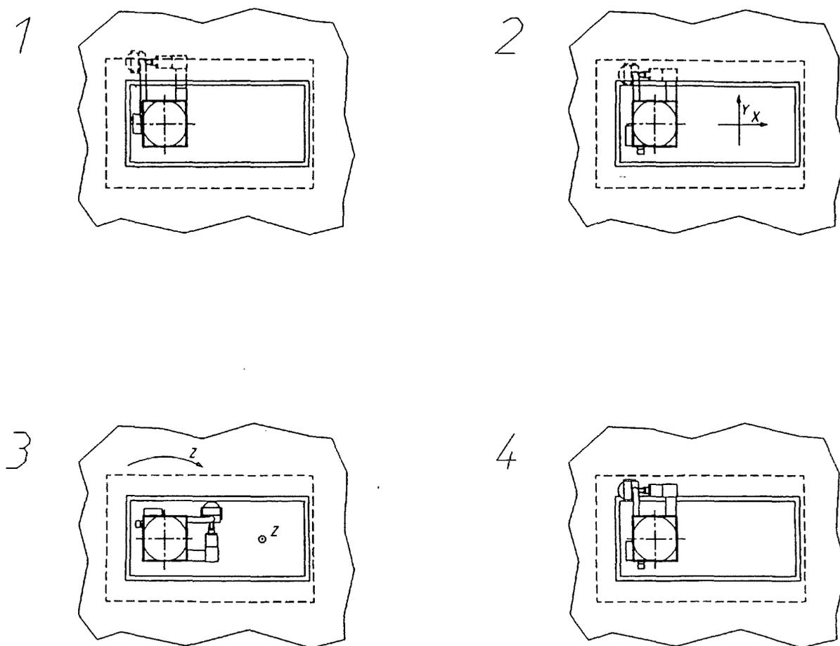
**Fig. 14:** Steps of operation for the removal of the Li-target
