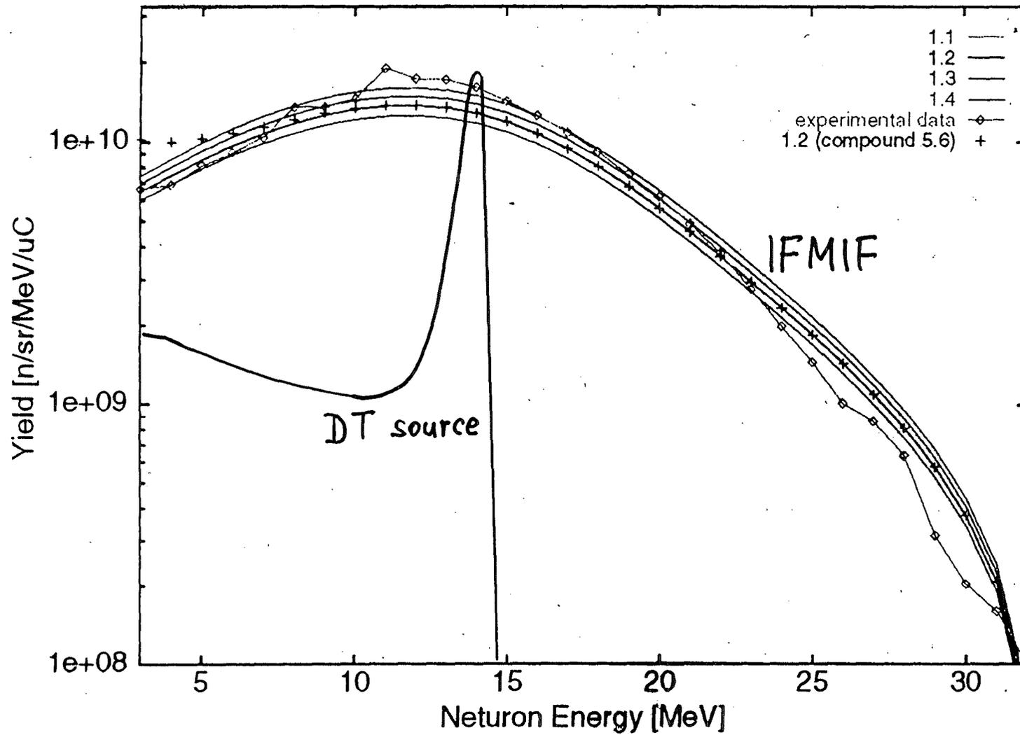
**Fig. 1:** Comparison between data and model in forward direction to determine magnitude of stripping component
