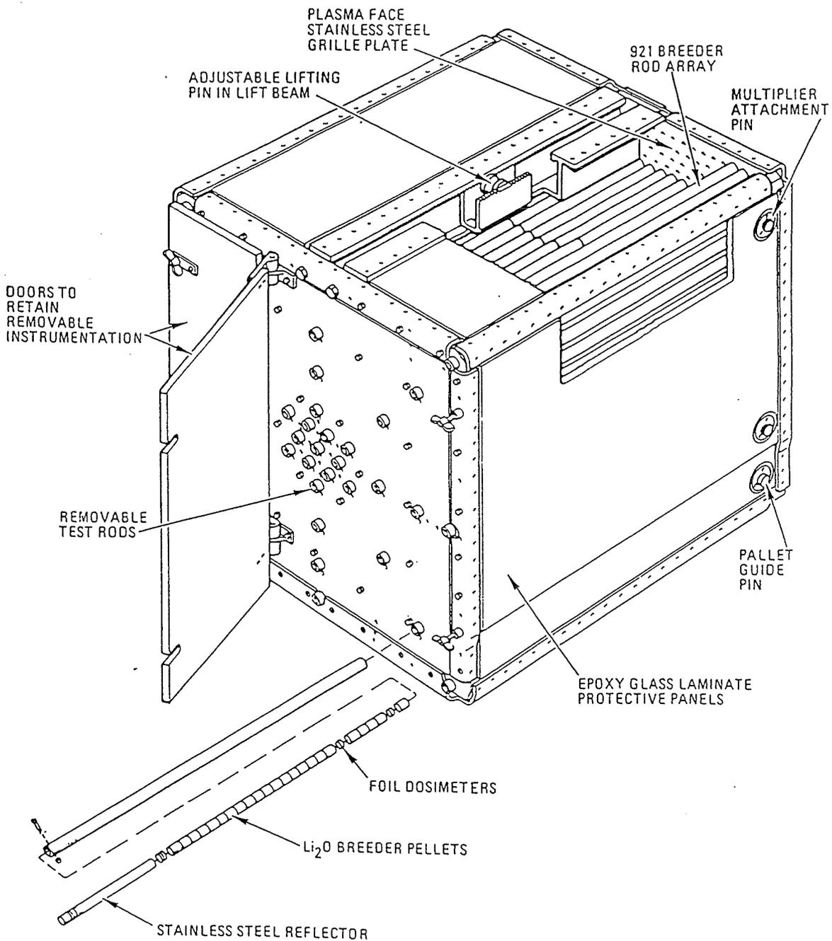
**Example of Wire Dosimeter Loading in Li Blanket Module**
