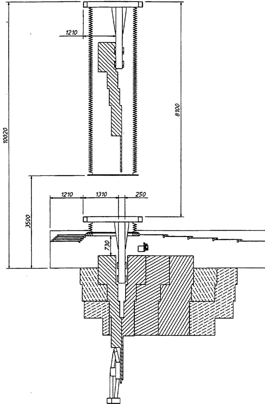
Fig. 5: Remote handling procedure; Gripper/bag gripping the high flux test module.
