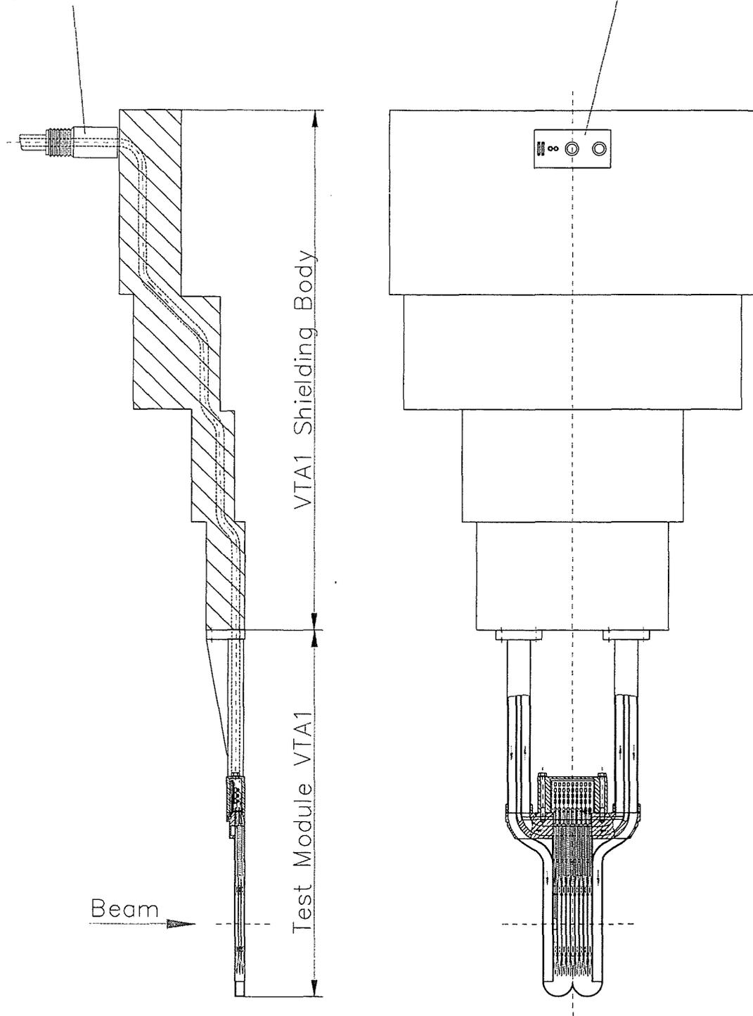
**Fig. 7:** Design configuration for the VTA1 (helium gas cooled version) with assembled test module; elevation view.
