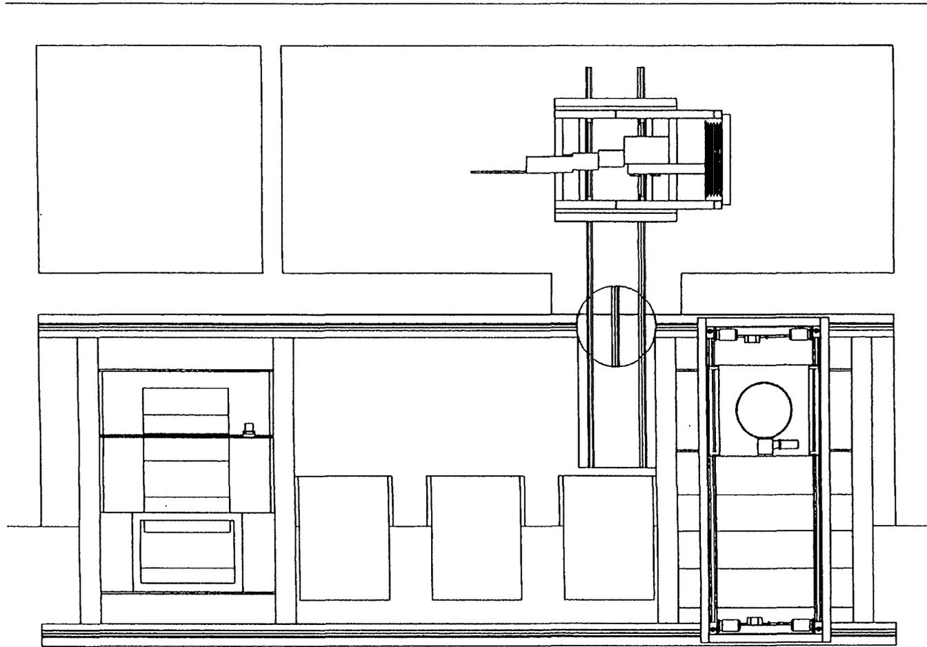
**Fig. 13:** Top view with the universal robot system and the transfer device (moving a VTA).
