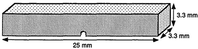
e) Dynamic/static fracture toughness
