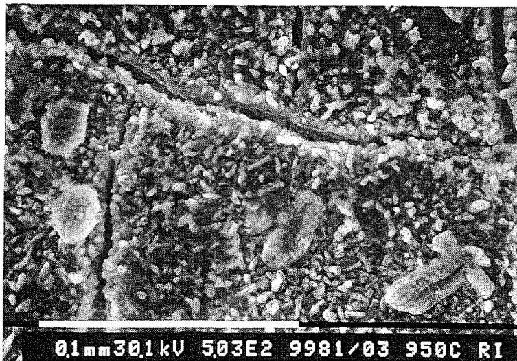
Figure 9c: Surface morphology of a heat treated MANET II sample pipe (type C: 950°C / 2 h, 750°C / 2 h, inside wall, x 500).
