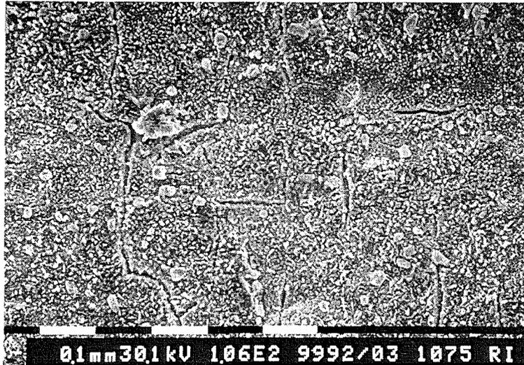
Figure 9d: Surface morphology of a heat treated MANET II sample pipe (type D: 1075°C / 0.5 h, 750°C / 2 h, inside wall, x 100).
