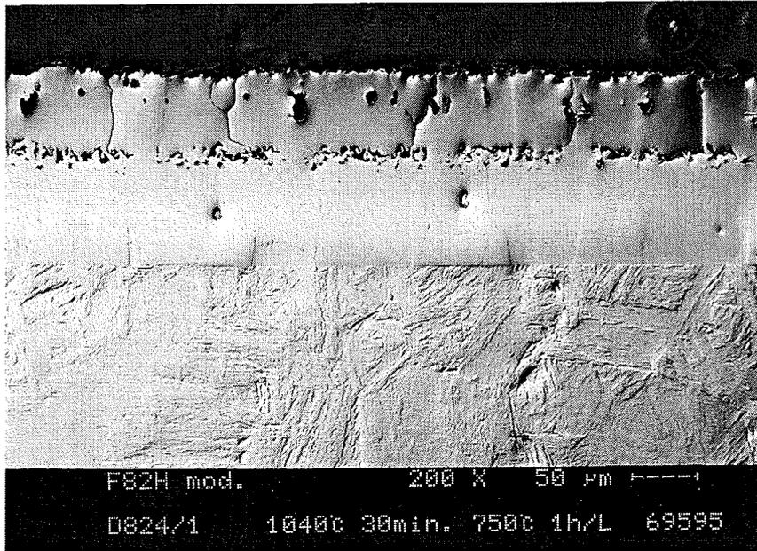
Figure 10a: Cross section of a heat treated F82H-mod. sample sheet (type A: 1040°C / 0.5 h, 750°C / 1 h, x 200).
