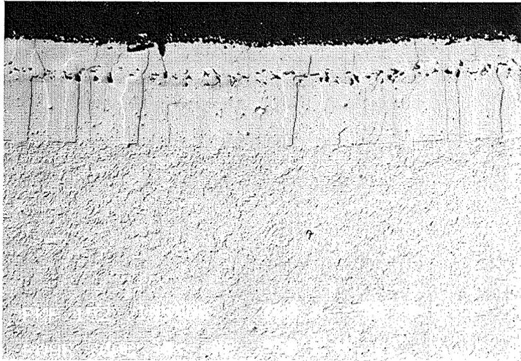
Figure 11b: Cross section of a heat treated MANET II sample pipe (type C: 950°C / 2 h, 750°C / 2 h, inside wall, x 200).
