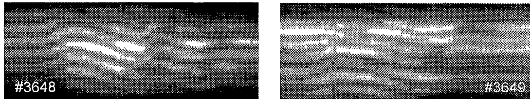
Figure 2.20: Line imaging ORVIS interferograms of spall experiments with deformed 0.28 mm thick molybdenum single crystals. Both samples were cut of the same piece of material. The measuring line was oriented parallel to the rolling direction (#3648) and perpendicular to it (#3649).
