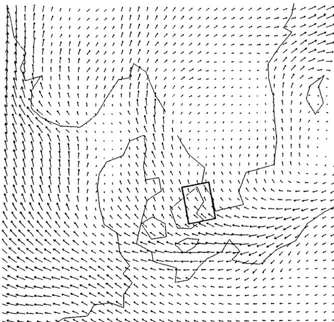
**Figure 4c:** Subset (40x40 grid points or ~ 1000 kmx 1000 km) of surface (10m) winds over Northern Europe on August 20, 1996 1300 UTC. The insert “box“ over Northern Zealand, Øresund and Copenhagen defines the bounds of the local scale model chain (i.e. the LSMC) nested grid.
