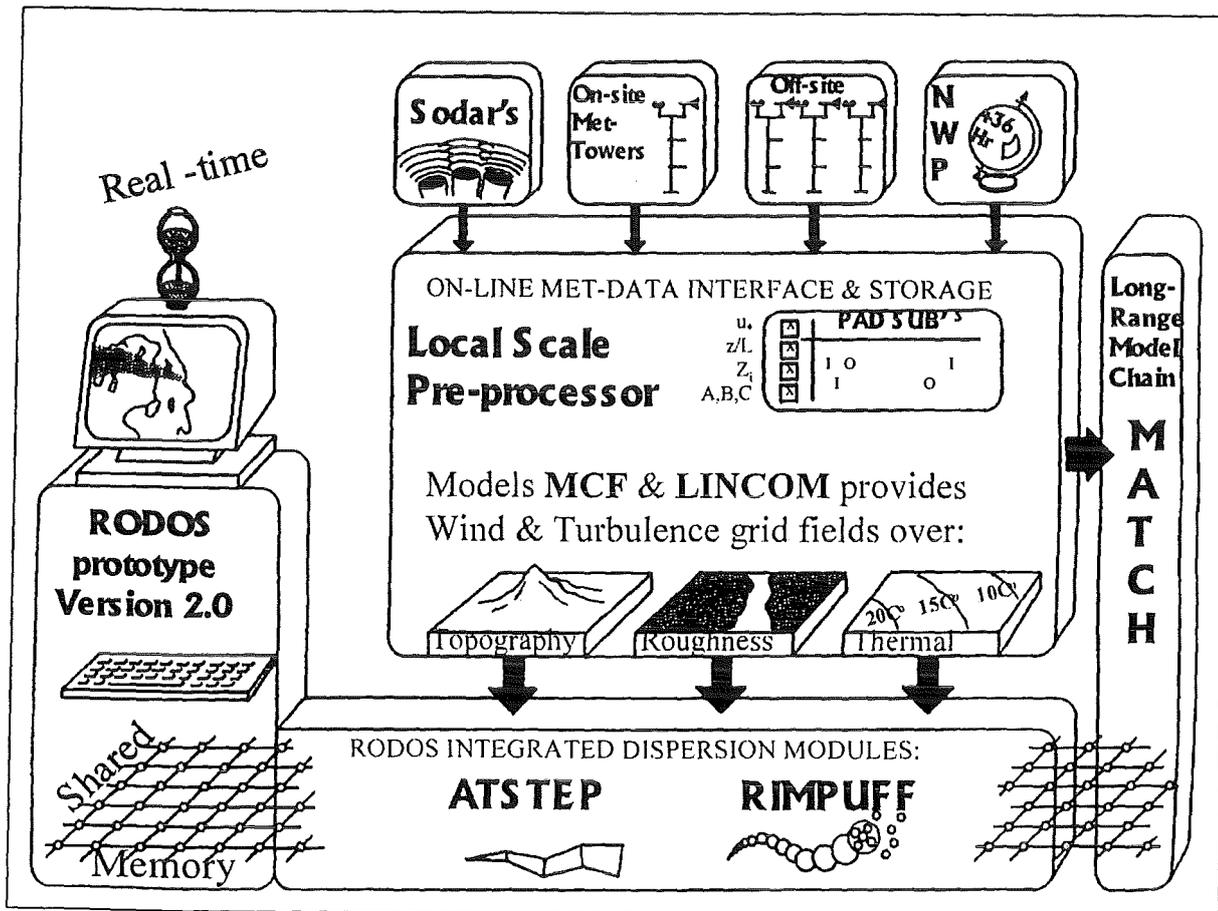
Figure 1a: The MET-RODOS system integrated with RODOS on a Unix based workstation
