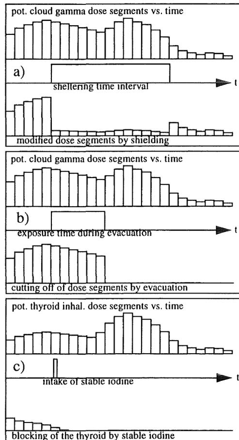
**Fig. 1: Modelling of the effect of emergency actions on dose; a) sheltering, B) evacuation, c) intake of stable iodine**
