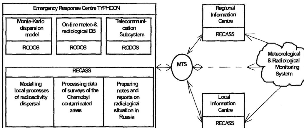
Figure 2: RECASS/RODOS coupling to ROSHYDROMET
