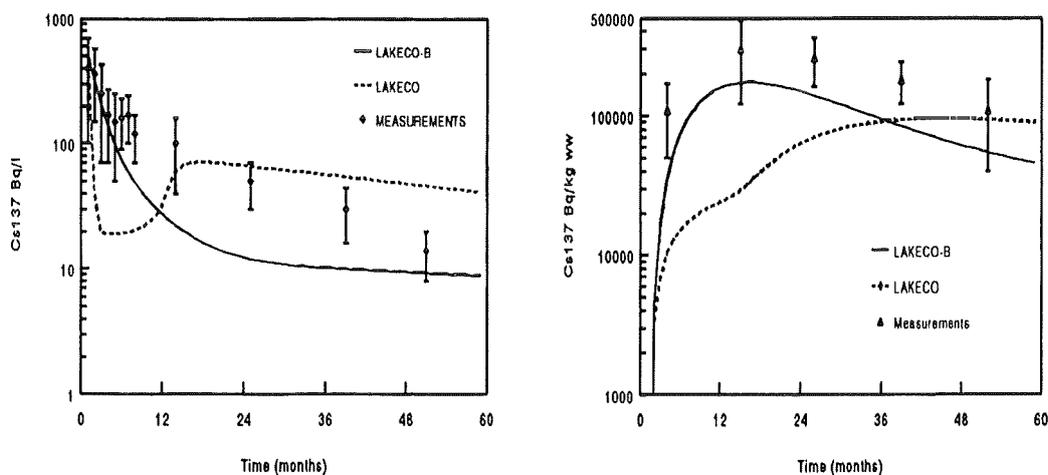
Fig. 6. LAKECO model results for Chernobyl NPP Cooling Pond
