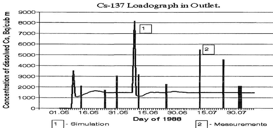
**Fig. 3. Simulation by RETRACE of  $^{137}\text{Cs}$  day averaged concentration in runoff from the Ilya River catchment**
