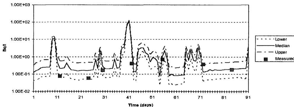
**Fig. 4. Simulation by RIVTOX of  $^{137}\text{Cs}$  concentration on suspended sediment at outflow from the Ilya River**
