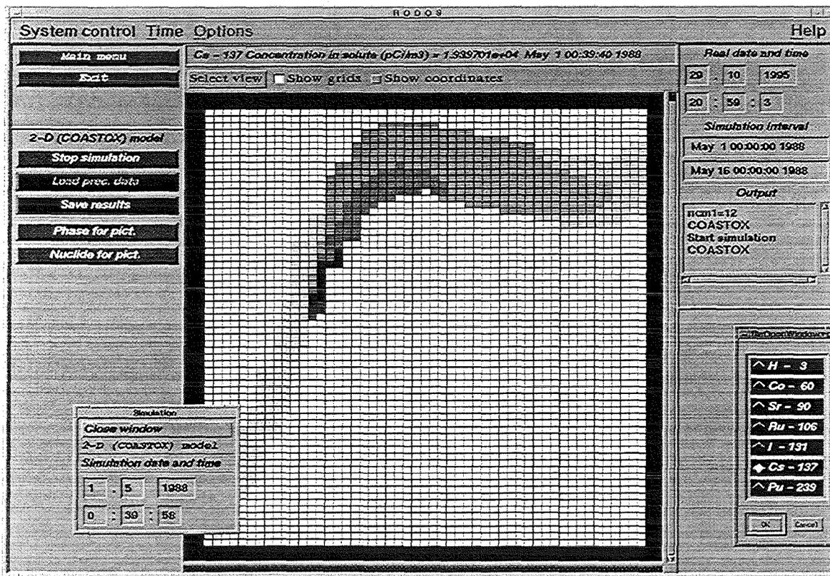
Fig. 5. Interface of COASTOX. Simulation of direct release into the Rhine River.
