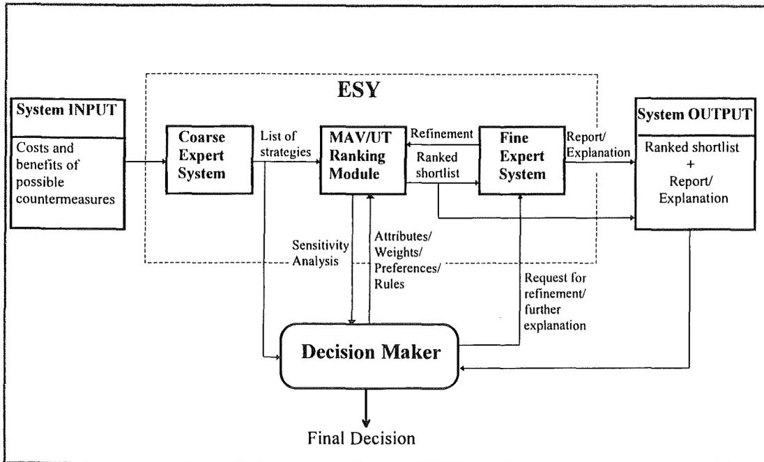
**Figure 1:** Outline of the proposed structure of the Evaluation Subsystem (ESY) of RODOS.
