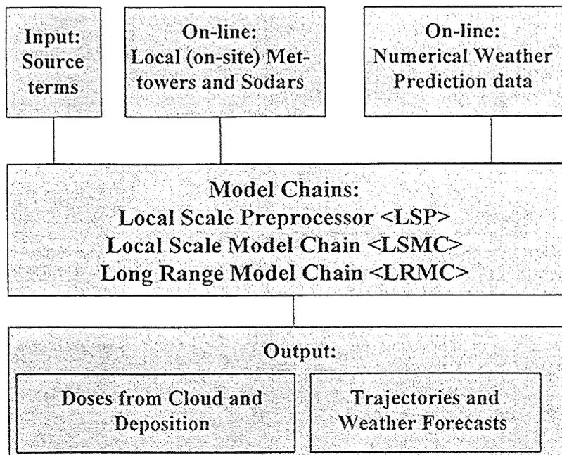
Figure 1c: MET-RODOS Input/Output and Model Chain Structure
