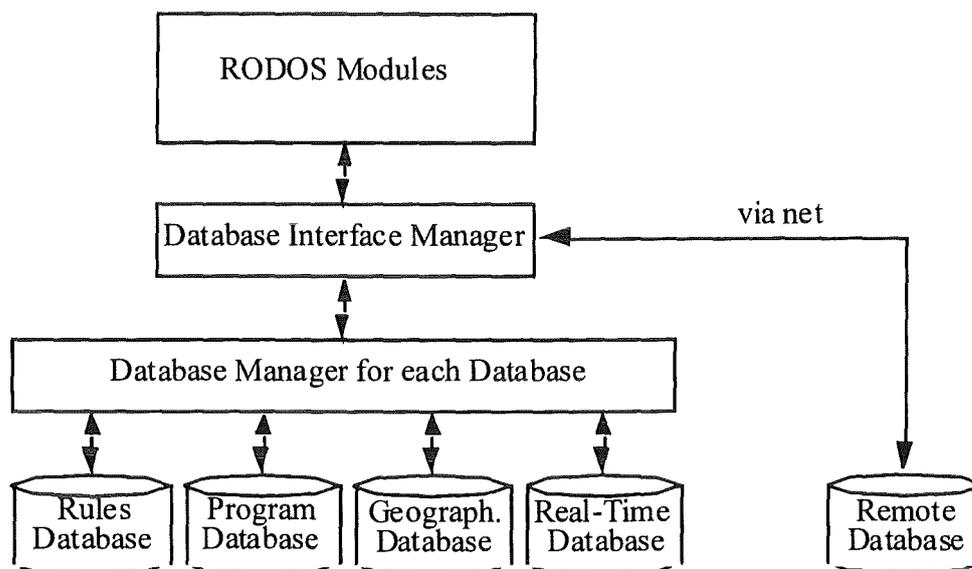
**Figure 2: Structure of the RODOS Distributed Database**
