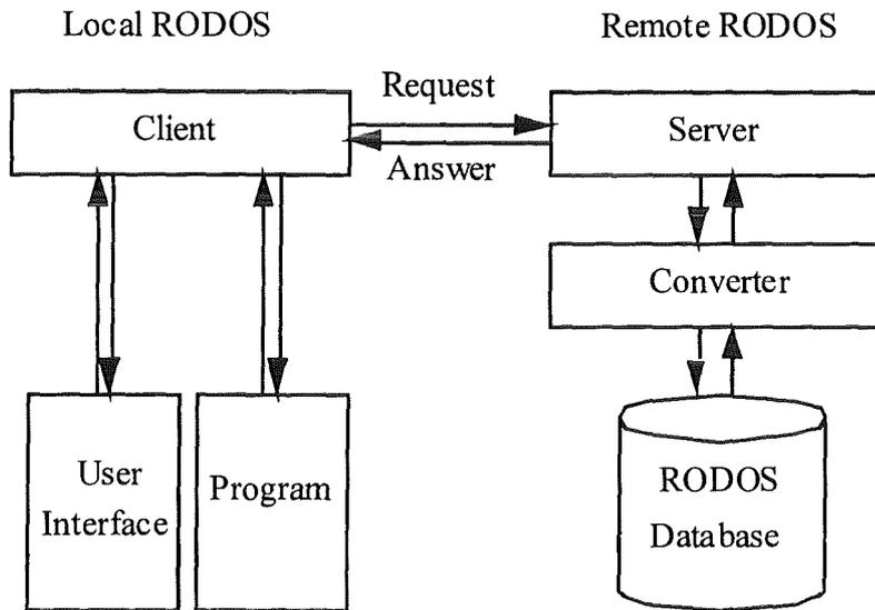
**Figure 3: The Connection to Remote Databases**
