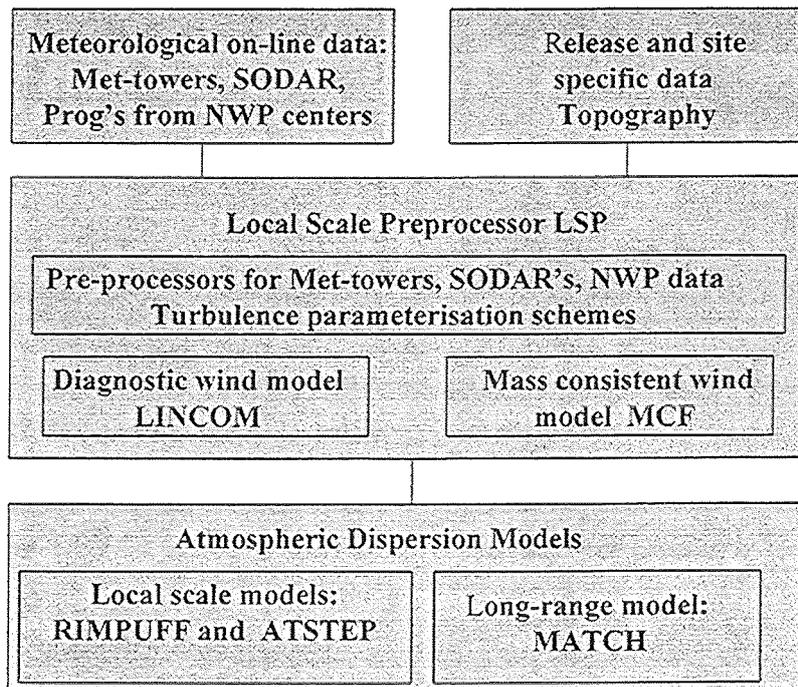
Figure 1b: MET-RODOS Atmospheric Dispersion Model Chain
