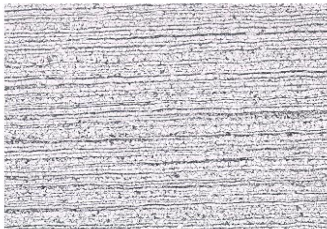
Figure 5.1 Optical micrograph showing TStE355 carbon steel microstructure (x80)
