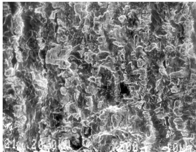
Figure 5.13 SEM micrograph of the fracture surface of a TStE355 steel specimen tested in NaCl brine at 170°C and a strain rate of 10^{-7} \text{ s}^{-1}
