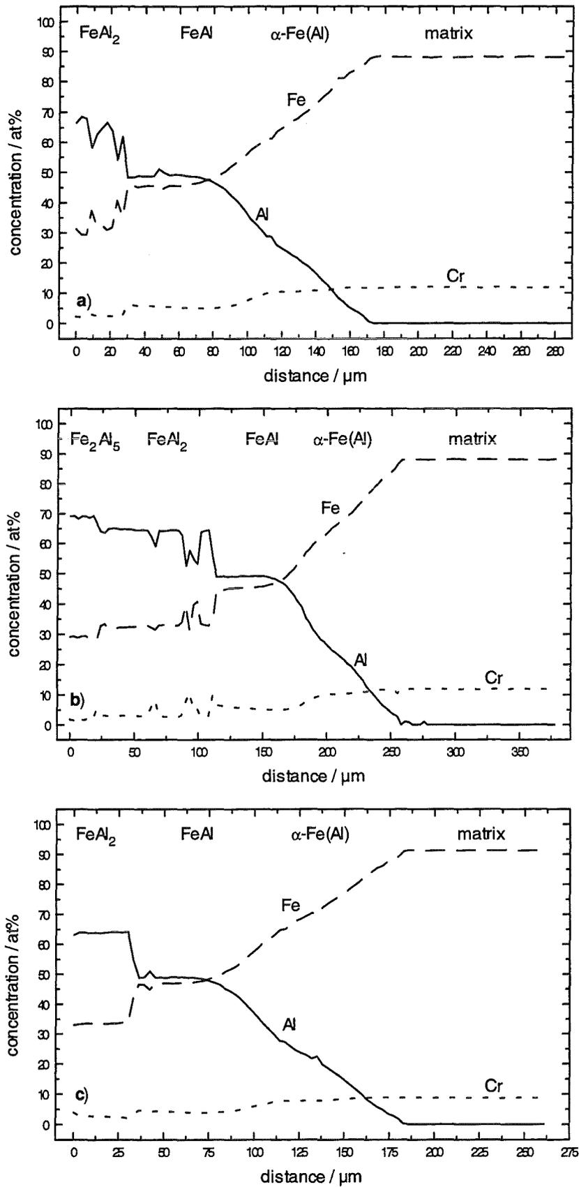
Fig. 5: EPMA line scans of hot dip aluminised F82H-mod. sample sheets after heat treatment (1040 °C / 30 min, 750 °C / 1 h) and HIPping under a) 1000 bar, b) 2000 bar and c) 3000 bar.
