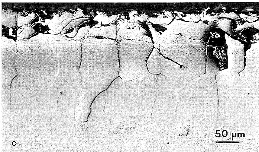
Fig. 3: Polished cross sections of hot dip aluminised F82H-mod. sample sheets after heat treatment (1040 °C / 30 min, 750 °C / 1 h) under a) 1000 bar, b) 2000 bar and c) 3000 bar.
