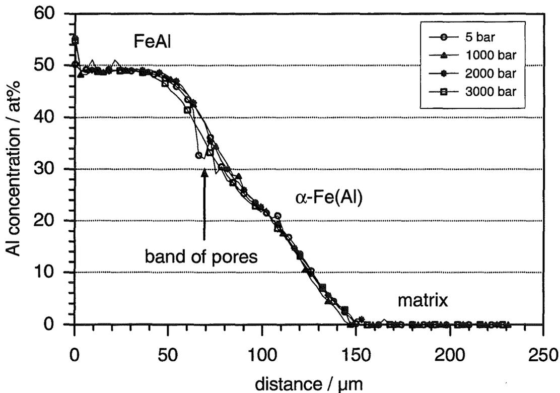
Fig. 6: Comparison of the Al concentration versus distance obtained for sample 1, 2, 3 and 4.
