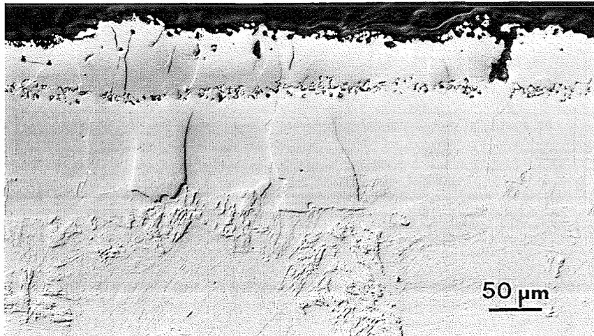
Fig. 2: Polished cross section of hot dip aluminised F82H-mod. sample after heat treatment (1040  $^{\circ}\text{C}$  / 30 min, 750  $^{\circ}\text{C}$  / 1 h) under 5 bar.
