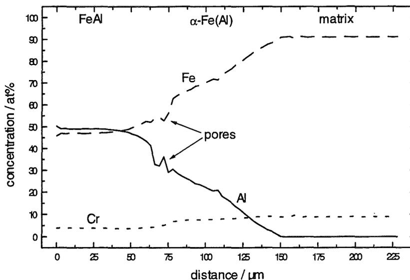
Fig. 4: EPMA line scans of hot dip aluminised F82H-mod. sample sheets after heat treatment (1040 °C / 30 min, 750 °C / 1 h) under 5 bar.
