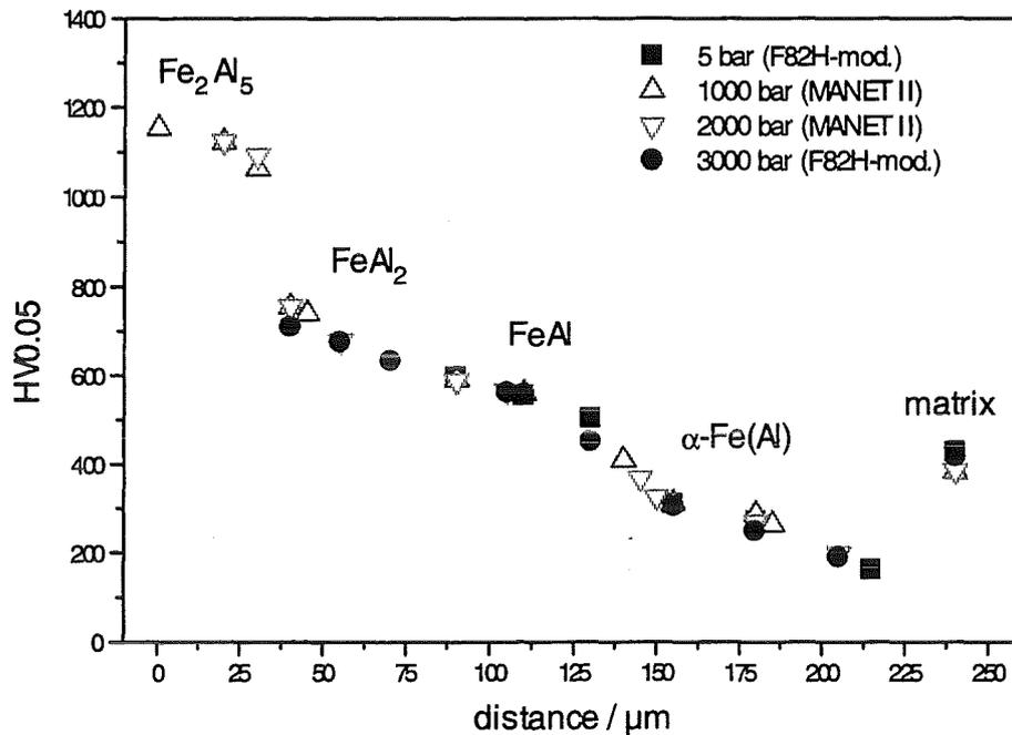
Fig. 7: Micro hardness measurements through the layers on samples 1, 2, 3 and 4.
