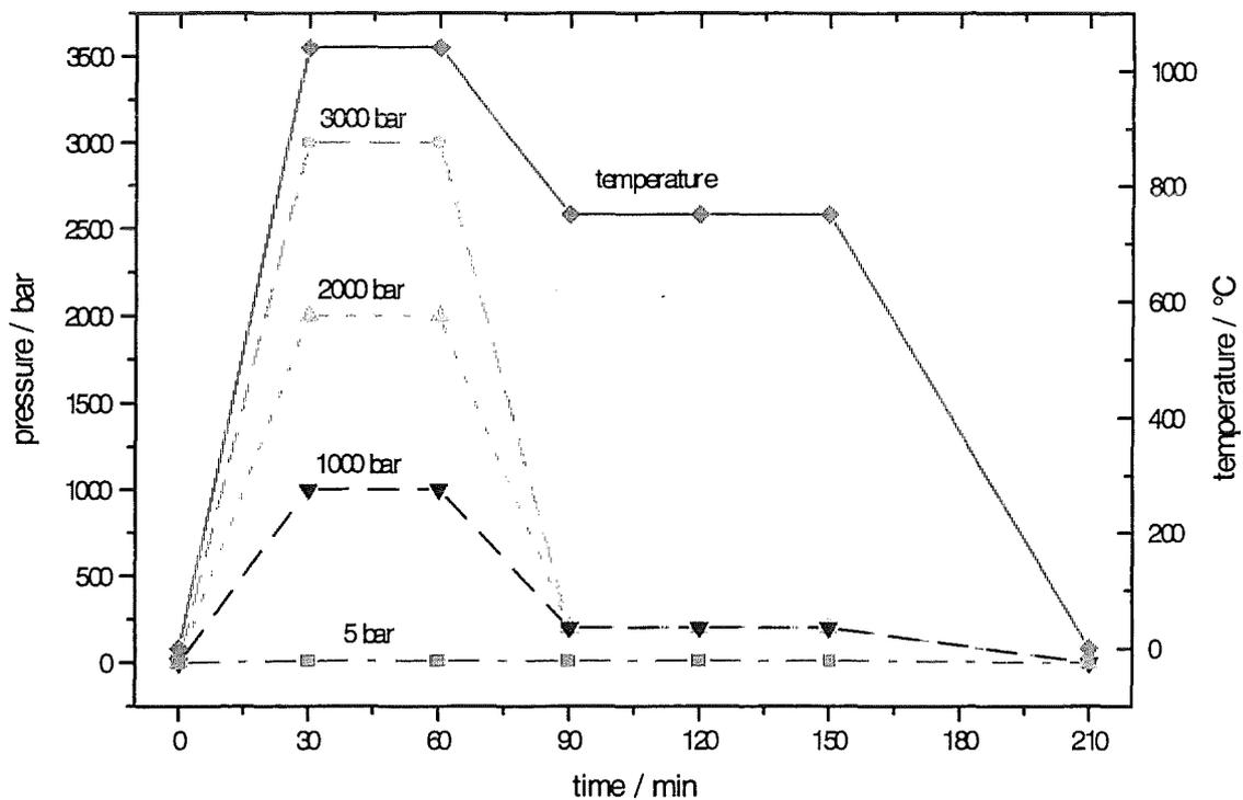
Fig. 1: HIP cycle used for austenitisation and tempering of hot dip aluminised steels.
